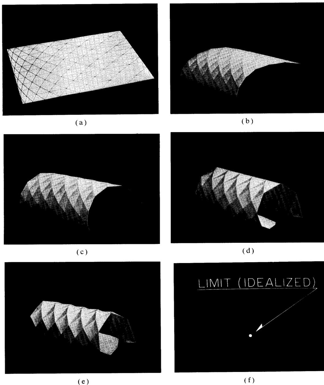
FIG. 17. Two-dimensional deployment mechanism by PCCP shell.
