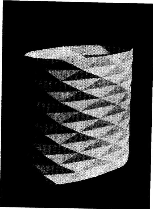
FIG. 6. Exaggerated view of an isometric, axially shortened surface corresponding to an elliptic cylindrical surface (major-to-minor axis ratio=2).
