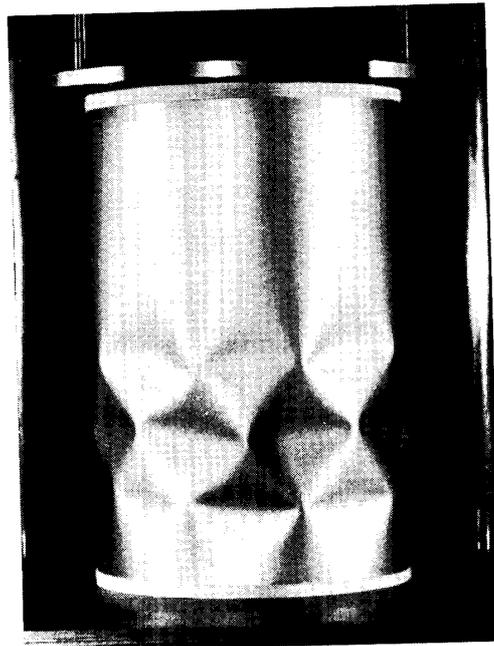
FIG. 3. Buckling pattern of a circular cylindrical shell subjected to axial loading.
