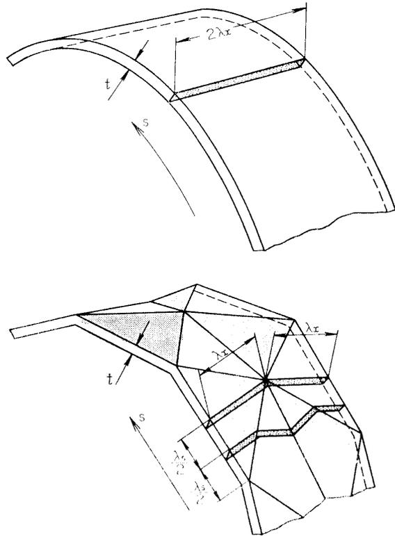
FIG. 16. Comparison of moment of inertia between cylindrical shell and PCCP shell.
