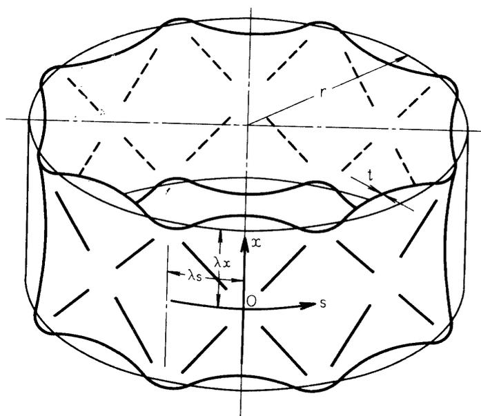
FIG. 1. Geometrical definitions of buckling deformation of circular cylindrical shell.
