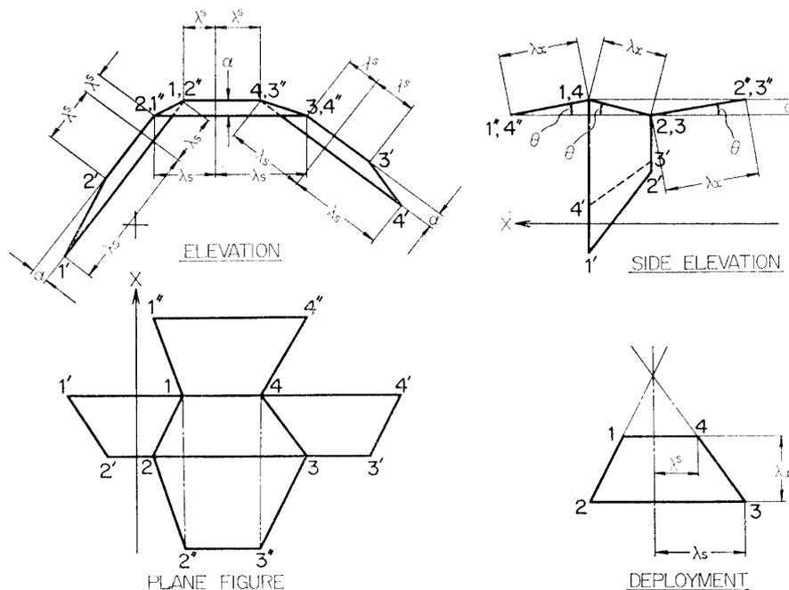
FIG. 14. Geometrical relation between elementary faces of PCCP surface (hexagonal pattern).
