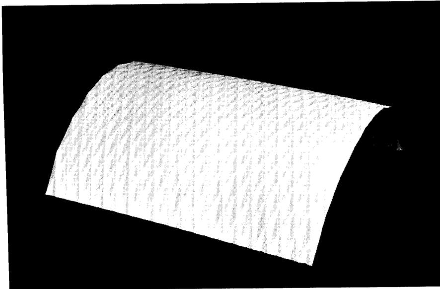
FIG. 19. Catenary PCCP shell as a large span structure (diamond pattern).
