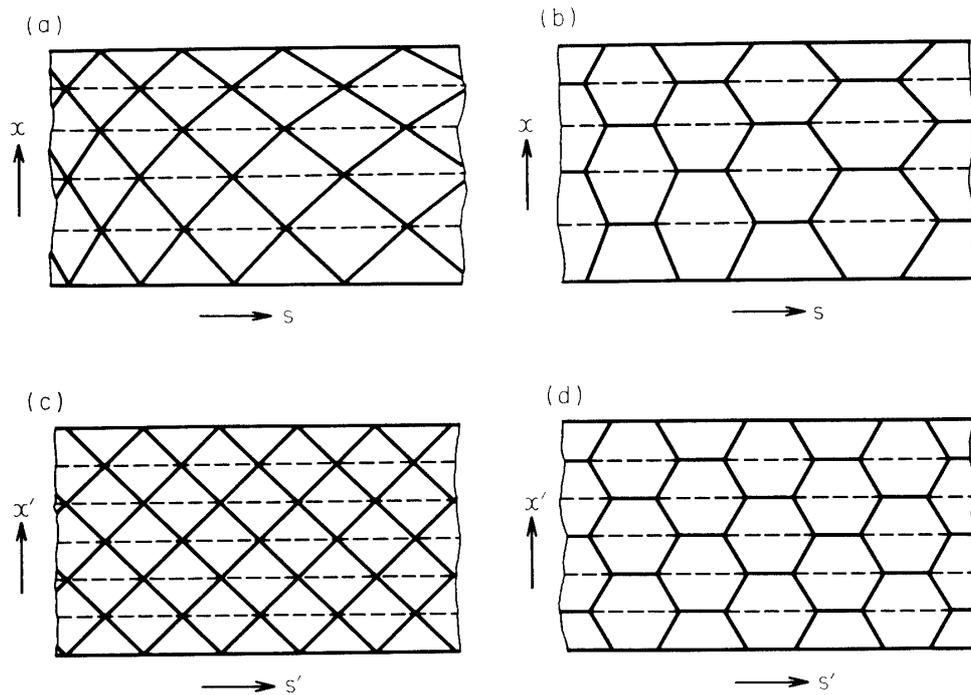
FIG. 12. Coordinate transfer of patterns to regular tessellation.
