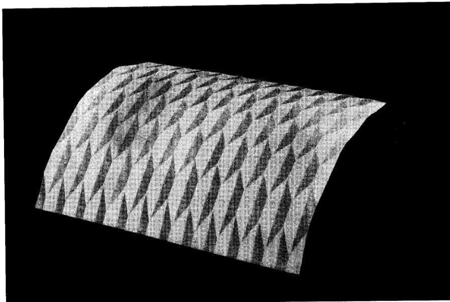
FIG. 20. Catenary PCCP shell as a large span structure (hexagonal pattern).
