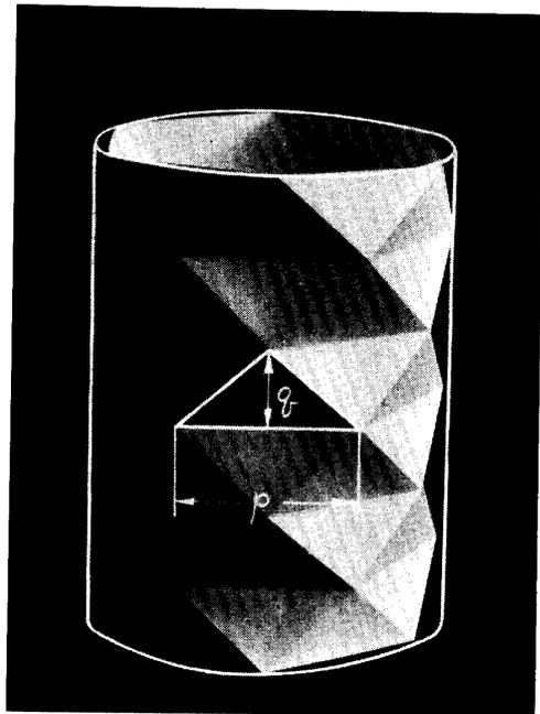
FIG. 7. Two-dimensional Euclidean complex  $K(p, q)$  inscribing a circular cylinder.
