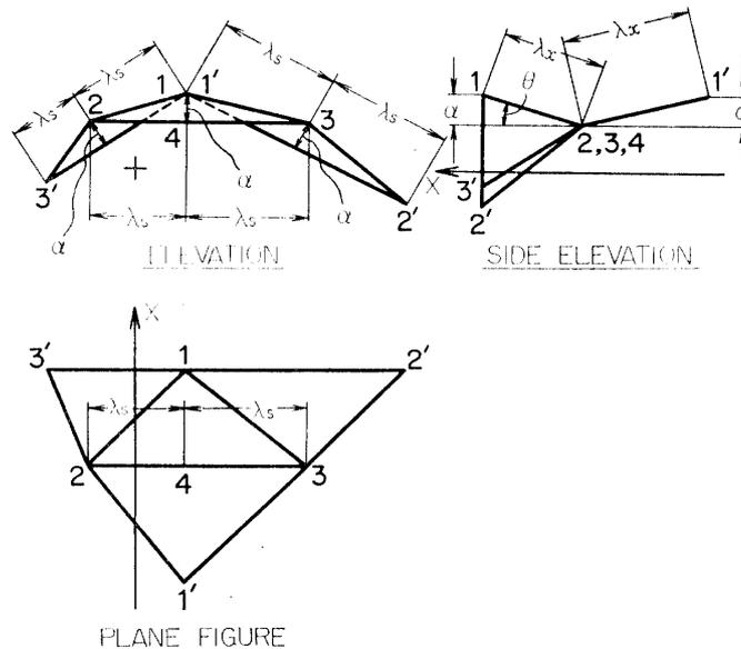
FIG. 13. Geometrical relation between elementary faces of PCCP surface (diamond pattern).
