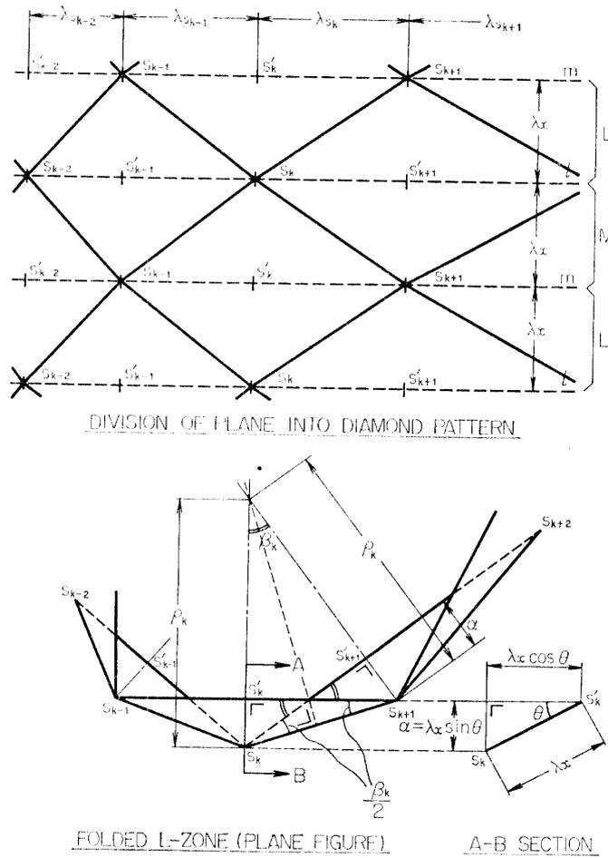
Fig. 5. Construction of a polyhedral surface from a plane.
