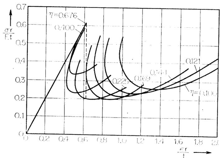
FIG. 15. Reduced compression stress  $\sigma_r/Et$  against unit end shortening  $\epsilon_r/t$  for  $\mu=1.00$  and different number of waves in circumferential direction (Kármán-Tsien).
