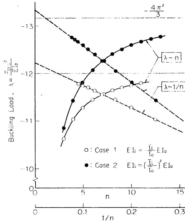
FIG. 3.3.2. Buckling Load at Optimum Shape.
