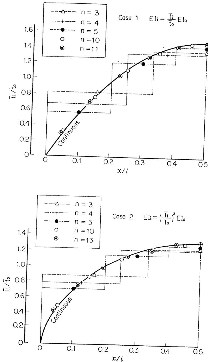
FIG. 3.3.3. Optimum Proportioning of Simply Supported Beam.
