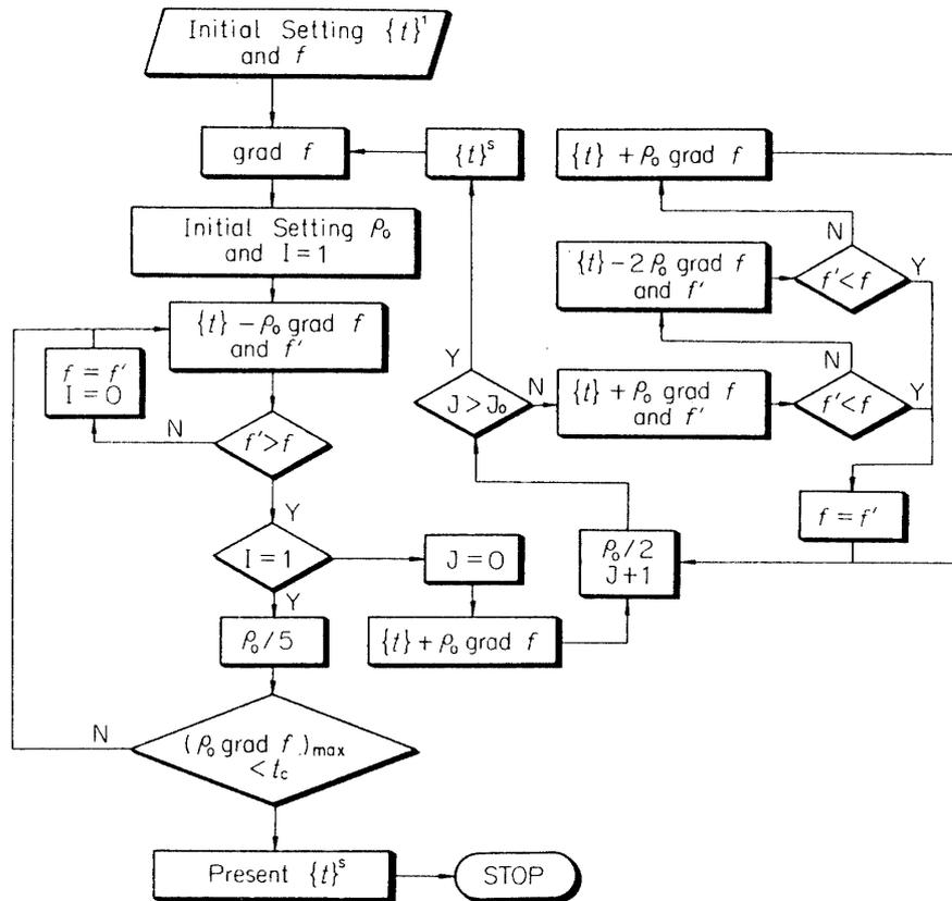
FIG. 2.4.4. Seeking the Minimum Point with the Steepest Descent Method.
