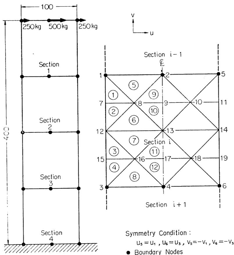
FIG. 3.1.1. Structural Partitioning
