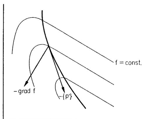
FIG. 2.4.6. Gradient Projection.
