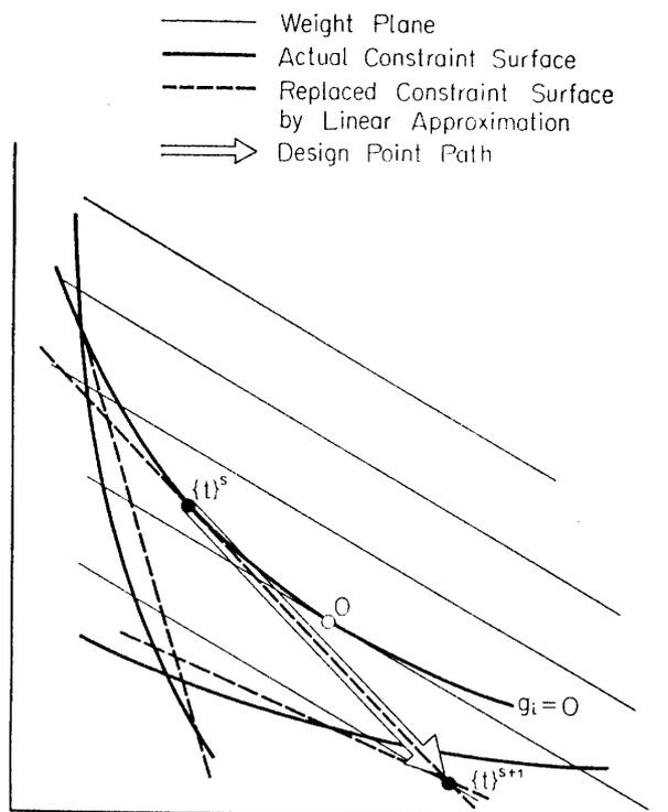
FIG. 2.4.5. Linearized Constraints and Path.
