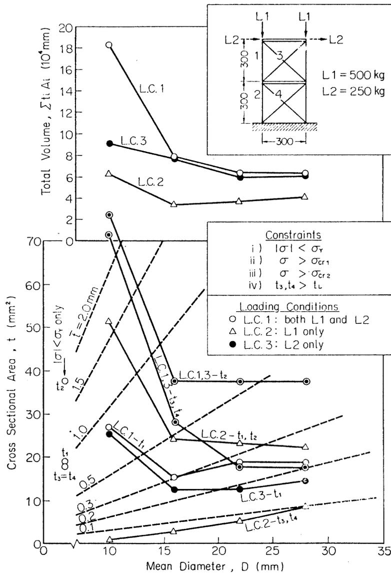
FIG. 3.2.1. Optimum Proportioning of Two Storied Truss.
