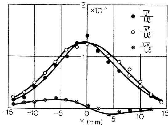
FIG. 5-29. Distributions of  $\bar{u}^2$ ,  $\bar{v}^2$  and  $\bar{uv}$  with sound of 630 Hz and 700 Hz.  $X=800$  mm.
