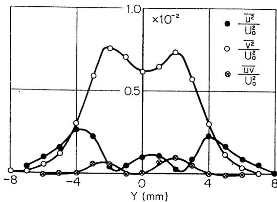
FIG. 4-20. Distributions of  $\overline{u^2}$ ,  $\overline{v^2}$  and  $\overline{uv}$  with sound of 630 Hz.  $X=150$  mm.
