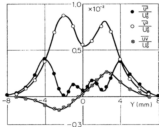
FIG. 4-19. Distributions of  $\overline{u^2}$ ,  $\overline{v^2}$  and  $\overline{uv}$  with sound of 630 Hz.  $X=100$  mm.
