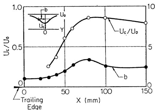
FIG. 3-2. Streamwise variations of non-dimensional velocity on the center line,  $U_c/U_0$  ( $U_0$ : free-stream velocity) and Half-value breadth,  $b$ , natural transition.
