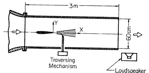
FIG. 2-3. Test-section arrangement and co-ordinate system.
