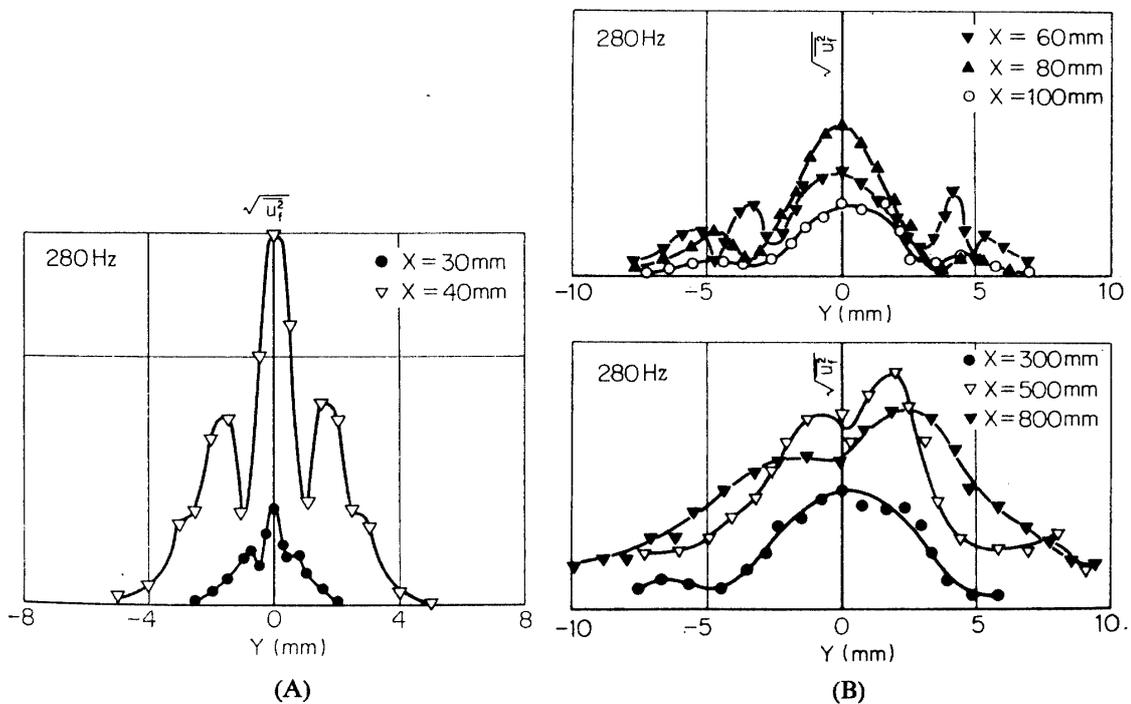
FIG. 5-20. Distribution of 280 Hz-component with sound of 630 Hz and 700 Hz. Ordinate scale is arbitrary. Relative values are expressed correctly.
