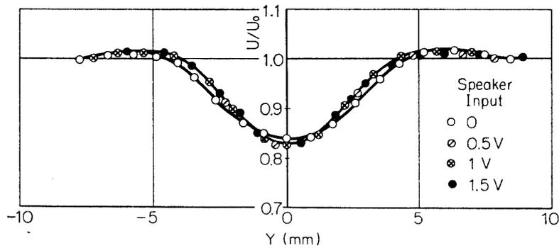
FIG. 4.3. Mean-velocity distribution with and without sound of 630 Hz,  $X=150$  mm,  $U_0=10$  m/s.
