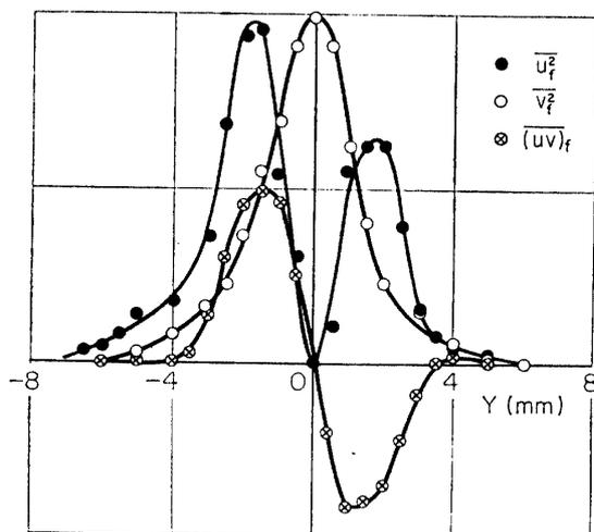
FIG. 5-33. Distributions of 700 Hz-components,  $\overline{u_f^2}$ ,  $\overline{v_f^2}$  and  $\overline{(uv)_f}$  with sound of 630 Hz and 700 Hz.  $X=40$  mm. Ordinate scale is arbitrary.
