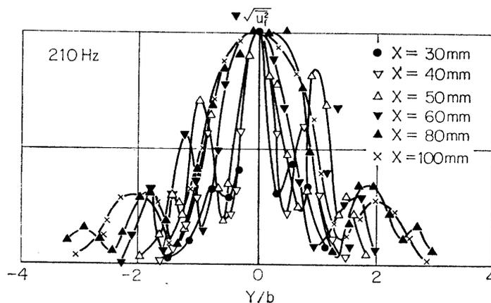
FIG. 6-8. Non-dimensional plot of distribution of 210 Hz-component with sound of 630 Hz and 700 Hz.
