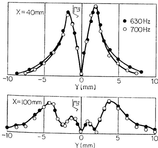
FIG. 5-2. Distributions of root-mean-square values of 630 Hz- and 700 Hz-fluctuation with sound of single frequency. Ordinate scale is arbitrary.  $X=4$ mm and 100mm.
