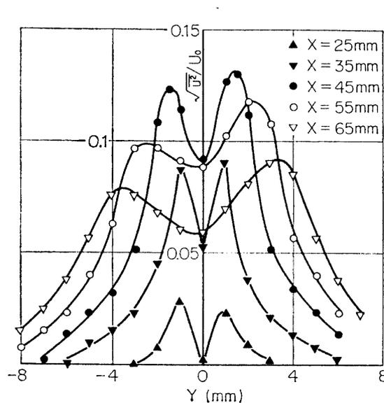
FIG. 4-14. Distribution of root-mean-square of  $u$ -fluctuation with sound of 630 Hz. Input to loudspeaker, 0.1 V.
