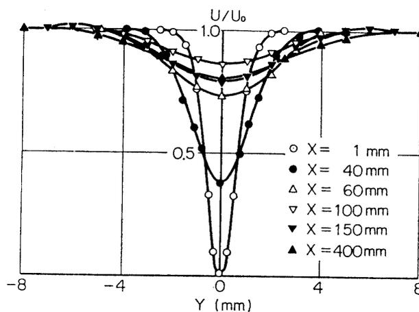
FIG. 3-1. Mean-velocity distribution in wake, natural transition, free-stream velocity,  $U_0=10$  m/s.
