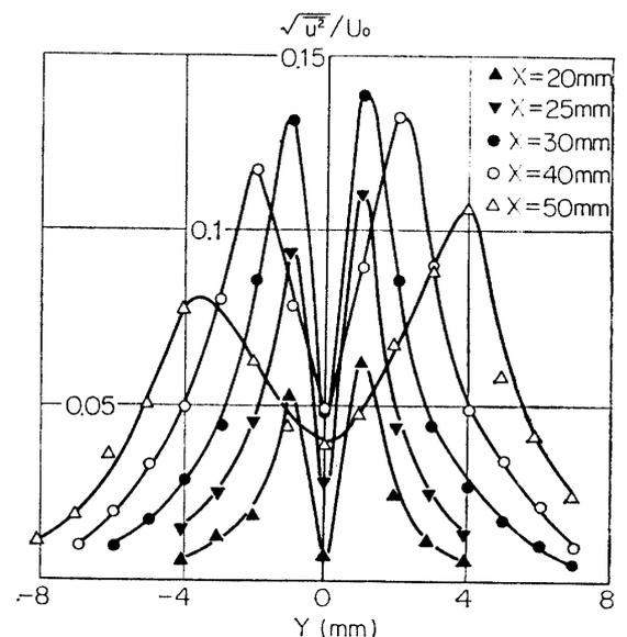
FIG. 4-15. Distribution of root-mean-square of  $u$ -fluctuation with sound of 630 Hz. Input to loudspeaker, 0.7 V.
