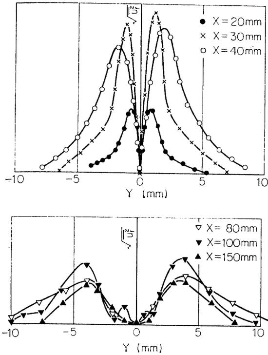
FIG. 5-22. Distribution of 630 Hz-component of  $u$ -fluctuation with sound of 630 Hz and 700 Hz. Ordinate scale is arbitrary.
