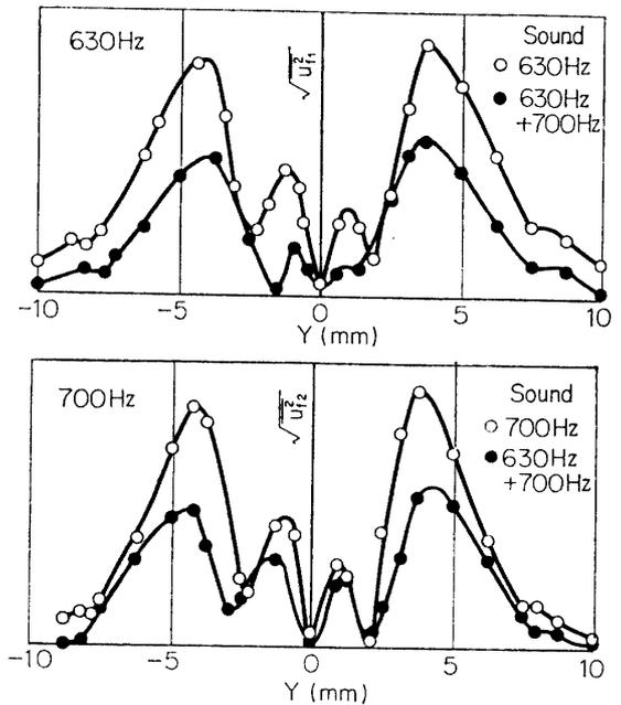
FIG. 5-5. Distributions of root-mean-squares of 630 Hz-,  $\sqrt{u_1^2}$ , and 700 Hz-fluctuation,  $\sqrt{u_2^2}$ , with sound of single frequency and two frequencies.  $X=100$  mm.
