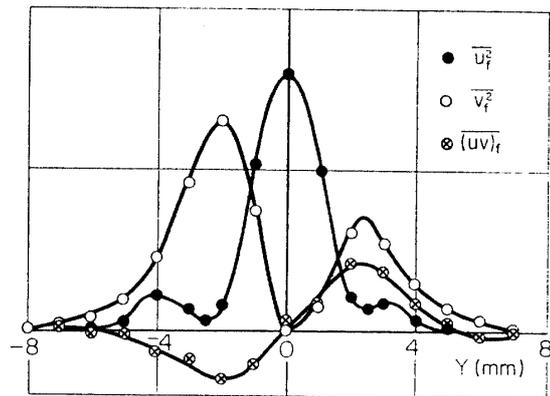
FIG. 5-36. Distributions of 1330 Hz-components,  $\overline{u_f^2}$ ,  $\overline{v_f^2}$  and  $\overline{(uv)_f}$  with sound of 630 Hz and 700 Hz.  $X=80$  mm. Ordinate scale is arbitrary.
