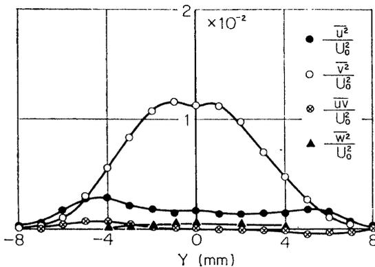
FIG. 3-11. Distributions of  $\overline{u^2}$ ,  $\overline{v^2}$ ,  $\overline{w^2}$  and  $\overline{uv}$ , natural transition,  $X=80$  mm.
