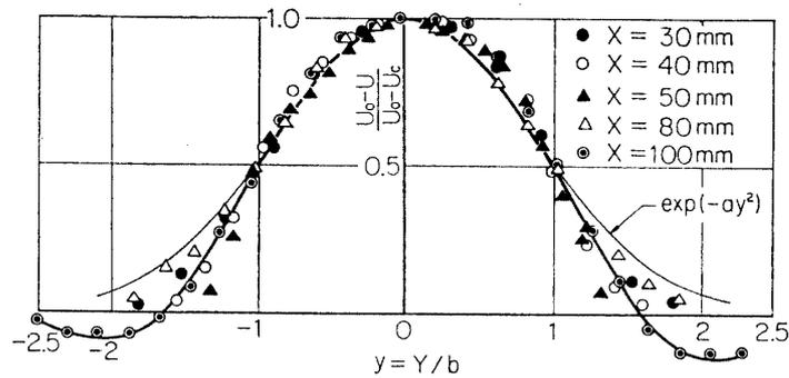
FIG. 6-1. Non-dimensional plot of mean-velocity distribution with sound of 630 Hz.  $U_0$ : freestream velocity,  $U_c$ : velocity on the center line,  $b$ : half-value breadth. Thin full line represents  $(U_0-U)/(U_0-U_c)=\exp(-ay^2)$ .
