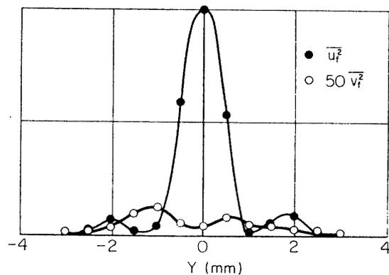
FIG. 5-30. Distributions of 70 Hz-components,  $\bar{u}_f^2$  and  $\bar{v}_f^2$  with sound of 630 Hz and 700 Hz.  $X=30$  mm. Ordinate scale is arbitrary.
