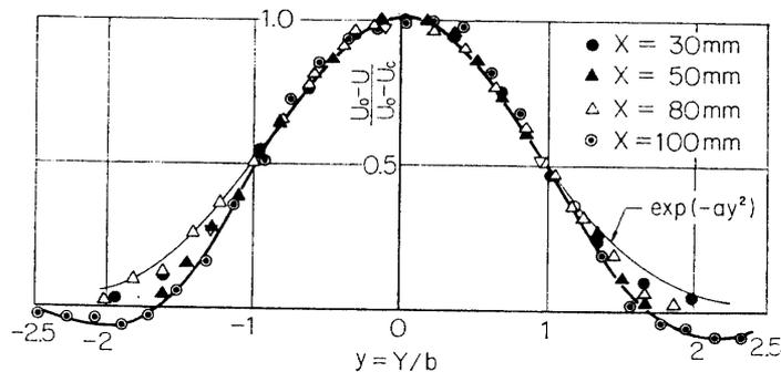
FIG. 6-2. Non-dimensional plot of mean-velocity distribution with sound of 630 Hz and 700 Hz.
