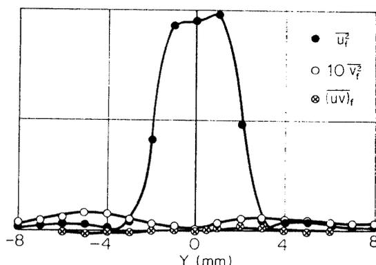
FIG. 5-32. Distributions of 70 Hz-components,  $\overline{u_f^2}$ ,  $\overline{v_f^2}$  and  $\overline{(uv)_f}$  with sound of 630 Hz and 700 Hz.  $X=80$  mm. Ordinate scale is arbitrary.
