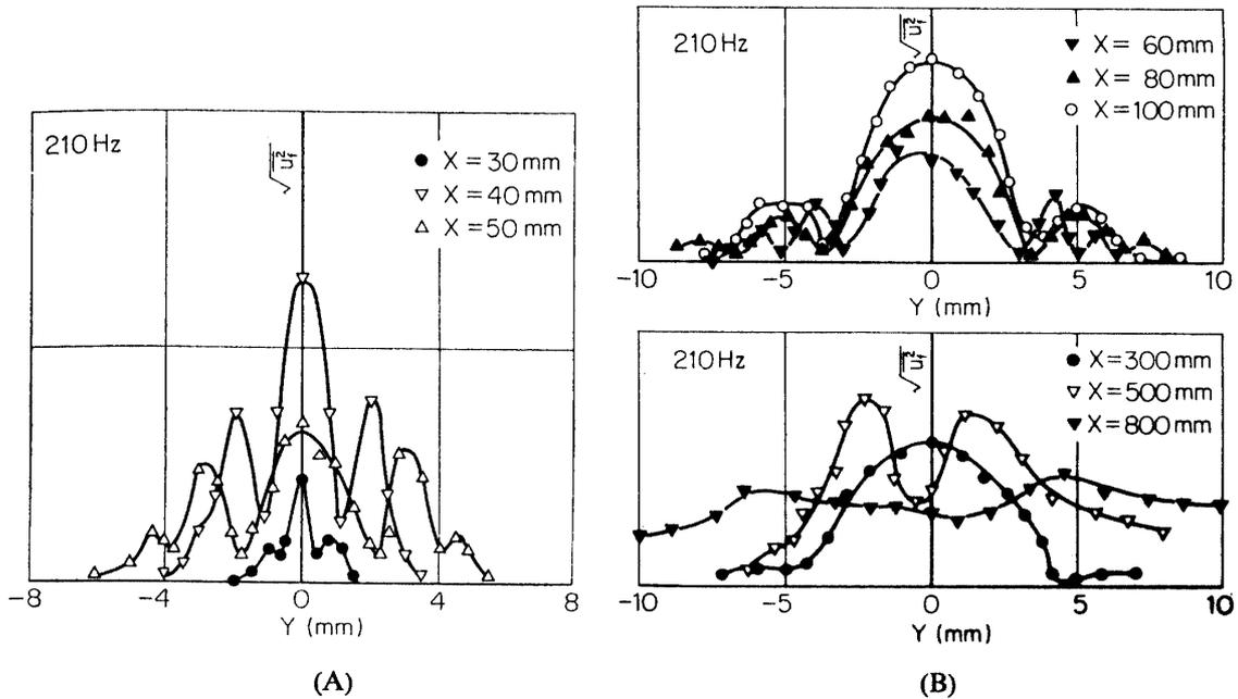
FIG. 5-19. Distribution of 210 Hz-component with sound of 630 Hz and 700 Hz. Ordinate scale is arbitrary. Relative values are expressed correctly.
