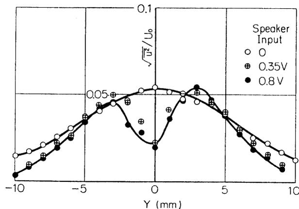
Fig. 4-13. Distribution of root-mean-square of  $u$ -fluctuation with and without sound of 630 Hz,  $X=600$  mm.
