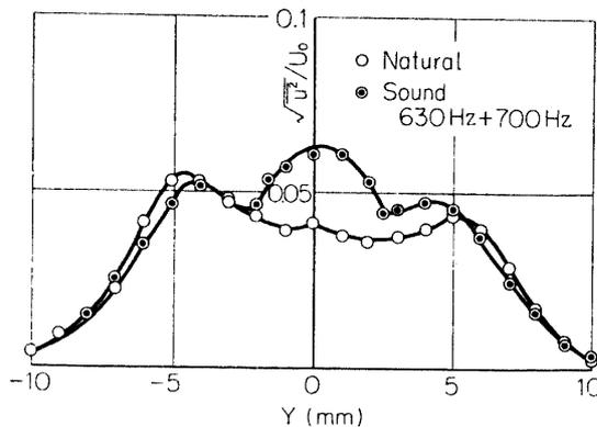
FIG. 5-13. Distribution of root-mean-square of  $u$ -fluctuation, natural and with two sounds.  $X=80$  mm.
