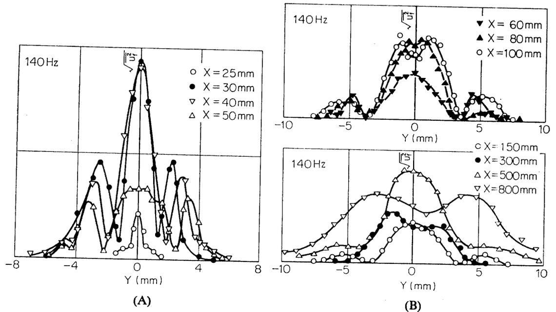
FIG. 5-18. Distribution of 140 Hz-component with sound of 630 Hz and 700 Hz. Ordinate scale is arbitrary. Relative values are expressed correctly.
