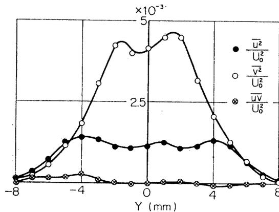
FIG. 3-15. Distributions of  $\overline{u^2}$ ,  $\overline{v^2}$  and  $\overline{uv}$ , natural transition,  $X=400$  mm.
