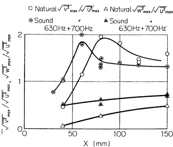
FIG. 6-11. Relative magnitudes of maximum values of  $\sqrt{\overline{u^2}}$ ,  $\sqrt{\overline{v^2}}$ , and  $\sqrt{\overline{w^2}}$  at each X-station. Natural transition and with sound of 630 Hz and 700 Hz.
