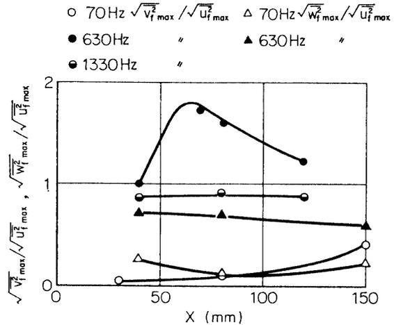
FIG. 6-12. Relative magnitudes of maximum values of spectral components (70 Hz, 630 Hz and 1330 Hz) at each X-station with sound of 630 Hz and 700 Hz.
