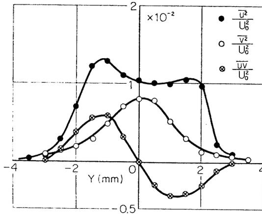
FIG. 5-25. Distributions of  $\overline{u^2}$ ,  $\overline{v^2}$  and  $\overline{uv}$  with sound of 630 Hz and 700 Hz.  $X=30$  mm.
