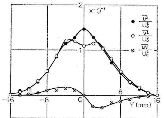
FIG. 3-16. Distributions of  $\overline{u^2}$ ,  $\overline{v^2}$  and  $\overline{uv}$ , natural transition,  $X=800$  mm.
