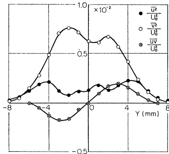
FIG. 3-12. Distributions of  $\overline{u^2}$ ,  $\overline{v^2}$  and  $\overline{uv}$ , natural transition,  $X=100$  mm.
