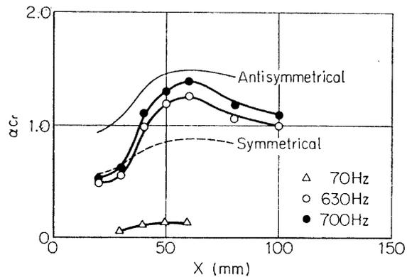
FIG. 6-4. Streamwise variations of non-dimensional frequency of three spectral components (70 Hz, 630 Hz and 700 Hz) with sound of 630 Hz and 700 Hz. Thin solid line, neutral frequency for antisymmetrical fluctuation and broken line, symmetrical fluctuation. Both by linear theory with local equilibrium.
