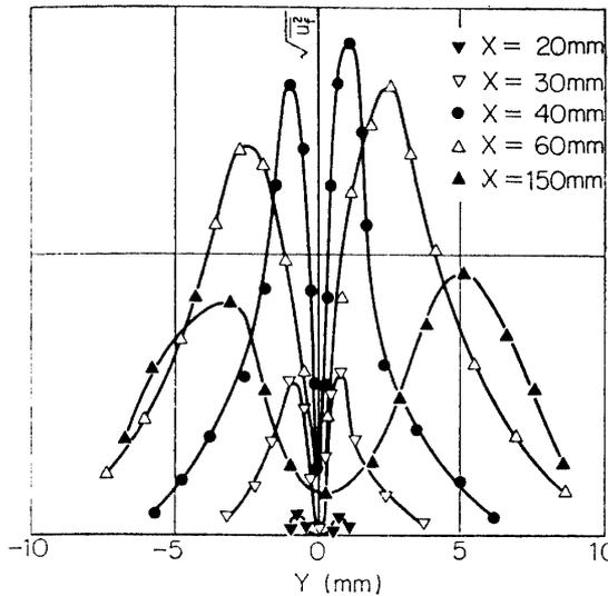
FIG. 3-17. Distribution of root-mean-square of fundamental component (630 Hz) of  $u$ -fluctuation, natural transition. Ordinate, arbitrary scale.
