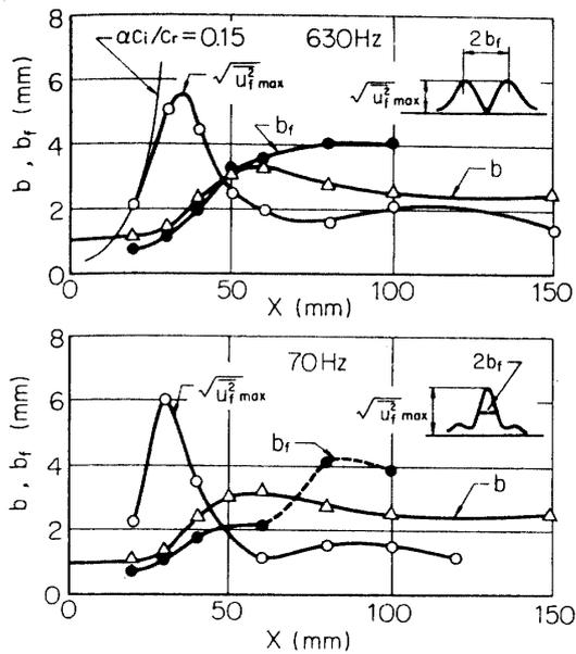
FIG. 6-3. Streamwise variations of maximum root-mean-square of spectral components at each  $X$ -station,  $\sqrt{u_f^2 \max}$  and of breadth of distributions,  $b_f$ .  $b$ : half-value breadth of mean-velocity distribution.
