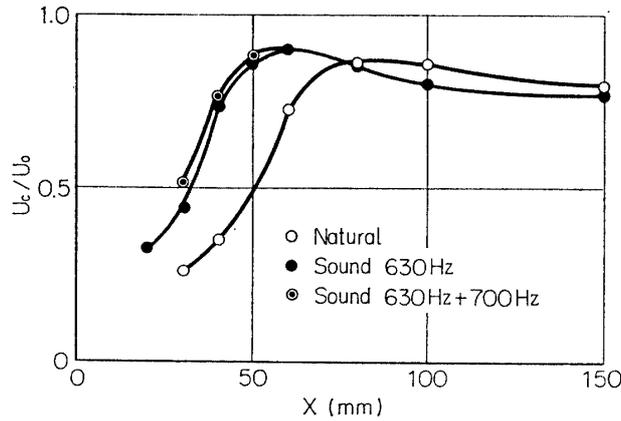
FIG. 5-6. Streamwise variation of velocity on the center line,  $U_c$ , in three cases.  $U_0=10$  m/s.
