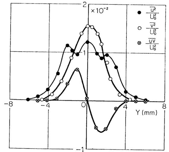
FIG. 5-26. Distributions of  $\overline{u^2}$ ,  $\overline{v^2}$  and  $\overline{uv}$  with sound of 630 Hz and 700 Hz.  $X=40$  mm.
