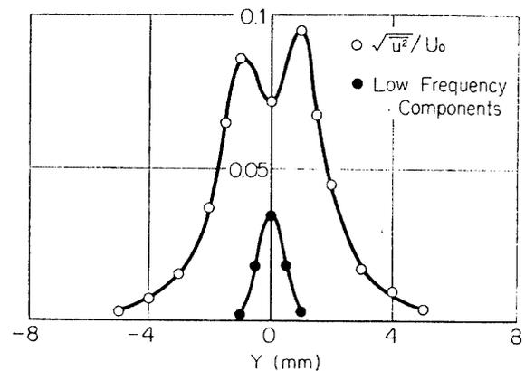
FIG. 8-2. Distributions of  $\sqrt{u^2}/U_0$  and low-frequency components at  $X=40$  mm. Natural transition.
