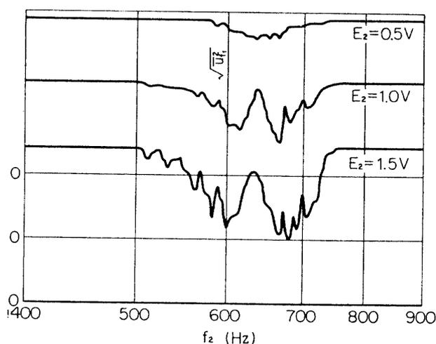
FIG. 5-1. Root-mean-square value of 630 Hz-component,  $\sqrt{u_1^2}$ , with second sound of various frequencies.  $X = 40$  mm,  $Y = 2$  mm,  $U_0 = 10$  m/s.
