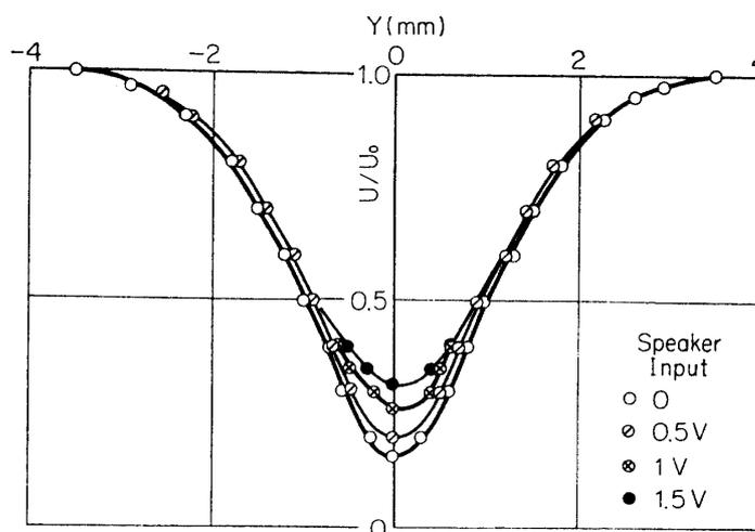
FIG. 4-1. Mean-velocity distribution with and without sound of 630 Hz,  $X=20$  mm,  $U_0=10$  m/s.
