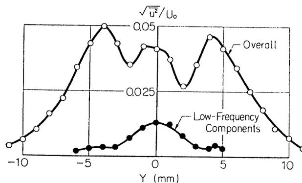
FIG. 8-3. Distributions of  $\sqrt{u^2}/U_0$  and low-frequency components at  $X=100$  mm. Natural transition.
