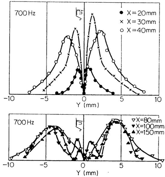
FIG. 5-23. Distribution of 700 Hz-component of  $u$ -fluctuation with sound of 630 Hz and 700 Hz. Ordinate scale is arbitrary.
