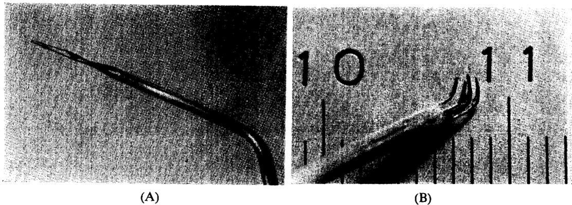
FIG. 2-5. (A) Single hot-wire anemometer. (B) X-wire, scale in centimeters.
