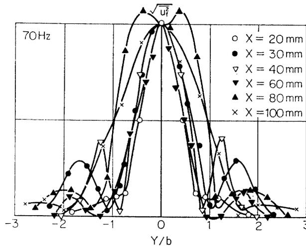
FIG. 6-7. Non-dimensional plot of distribution of 70 Hz-component, with sound of 630 Hz and 700 Hz.
