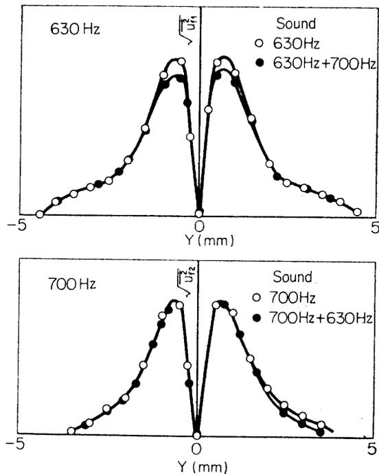
FIG. 5-3. Distributions of root-mean-square of 630 Hz-,  $\sqrt{u_{f_1}^2}$ , and 700 Hz-fluctuation,  $\sqrt{u_{f_2}^2}$ , with sound of single frequency and two frequencies.  $X=20$  mm.
