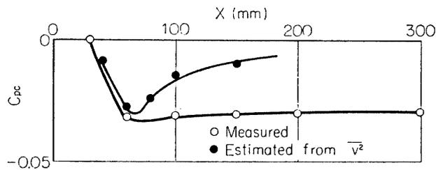
FIG. 7-1. Static-pressure coefficient on the center line, direct measurement and estimate from  $V^2$ . Natural transition.
