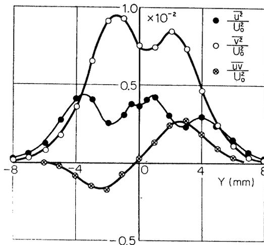
FIG. 5-27. Distributions of  $\overline{u^2}$ ,  $\overline{v^2}$  and  $\overline{uv}$  with sound of 630 Hz and 700 Hz.  $X=80$  mm.
