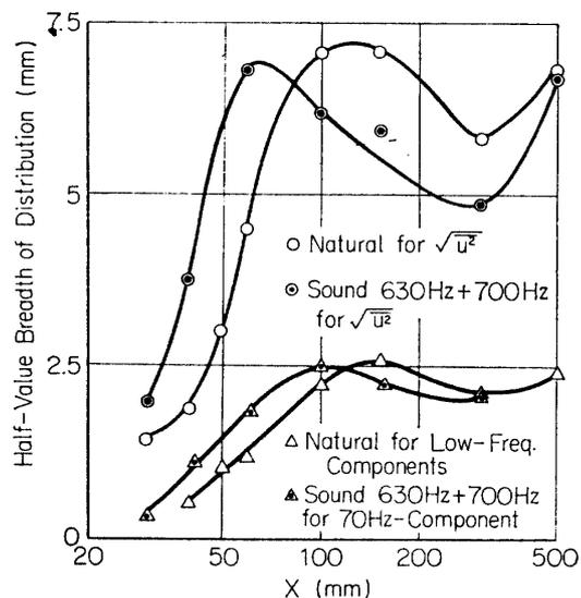
FIG. 8-5. Upper two curves: Streamwise variations of half-value breadth of distribution of  $\sqrt{u^2}$  in natural transition and with sound of 630 Hz and 700 Hz. Lower two curves: half-value breadth of distribution of root-mean-square of low-frequency components in natural transition and of 70 Hz-components with sound 630 Hz and 700 Hz.
