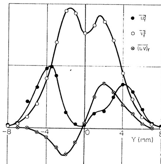
FIG. 5-34. Distributions of 700 Hz-components,  $\overline{u_f^2}$ ,  $\overline{v_f^2}$  and  $\overline{(uv)_f}$  with sound of 630 Hz and 700 Hz.  $X=80$  mm. Ordinate scale is arbitrary.
