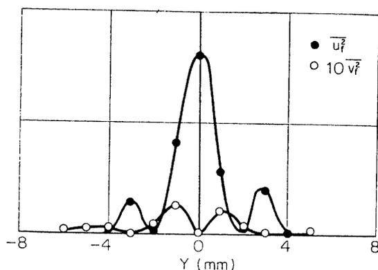
FIG. 5-31. Distributions of 70 Hz-components,  $\overline{u_f^2}$  and  $\overline{v_f^2}$  with sound of 630 Hz and 700 Hz.  $X=40$  mm. Ordinate scale is arbitrary.
