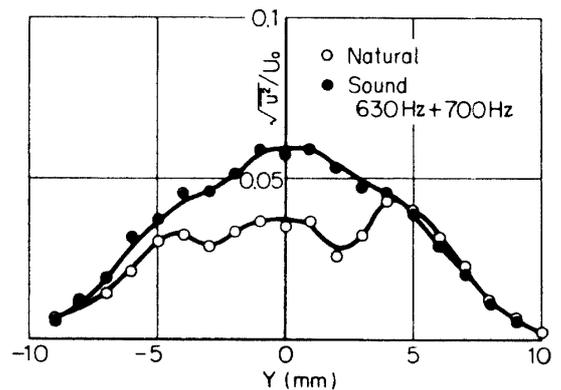
FIG. 5-14. Distribution of root-mean-square of  $u$ -fluctuation, natural and with two sounds.  $X=150$  mm.
