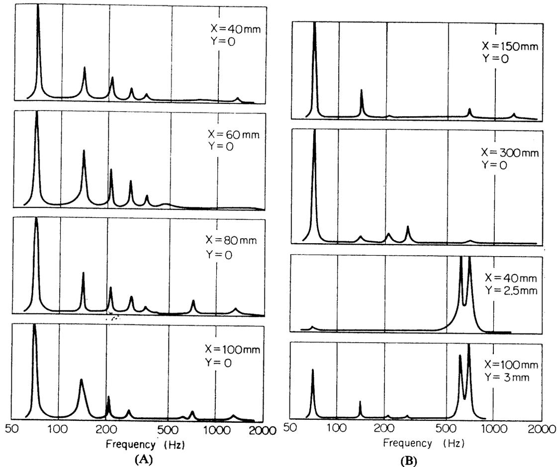
FIG. 5-16. Spectra of  $u$ -fluctuation with sound of 630 Hz and 700 Hz. Normalized by maximum values.
