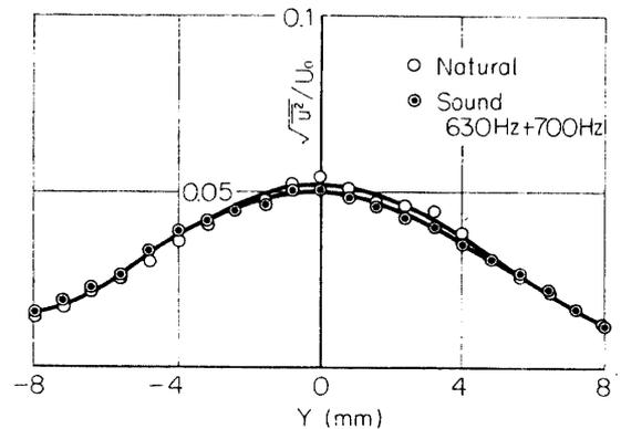
FIG. 5-15. Distribution of root-mean-square of  $u$ -fluctuation, natural and with two sounds.  $X=600$  mm.
