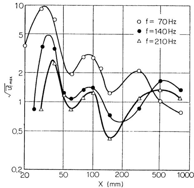
FIG. 5-21. Streamwise variations of three low-frequency components of  $u$ -fluctuation with sound of 630 Hz and 700 Hz.  $\sqrt{u_f^2}_{max}$ : maximum of  $\sqrt{u_f^2}$  at each  $X$ -station. Ordinate scale is arbitrary. Relative values are expressed correctly.
