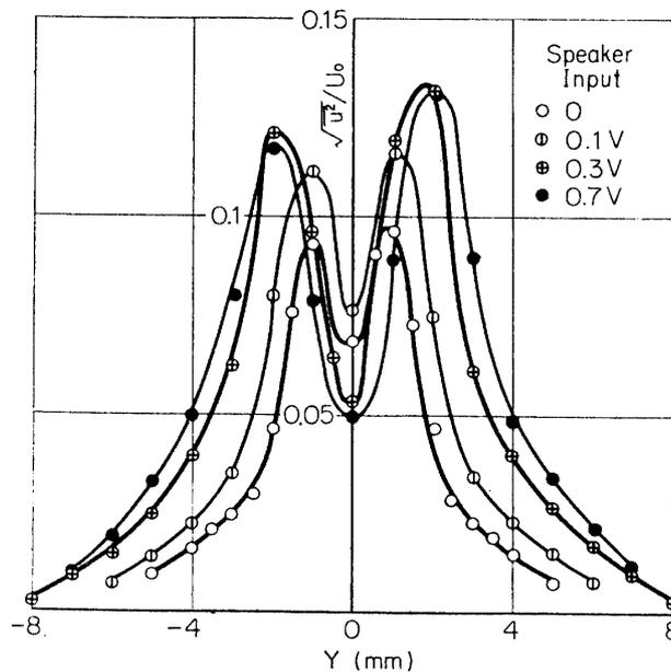
FIG. 4-12. Distribution of root-mean-square of  $u$ -fluctuation with and without sound of 630 Hz,  $X=40$  mm.
