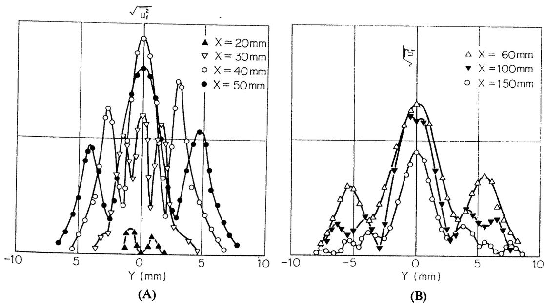
FIG. 5-24. Distribution of 1330 Hz-component of  $u$ -fluctuation with sound of 630 Hz and 700 Hz. Ordinate scale is arbitrary.
