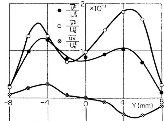
FIG. 4-21. Distributions of  $\overline{u^2}$ ,  $\overline{v^2}$  and  $\overline{uv}$  with sound of 630 Hz.  $X=800$  mm.
