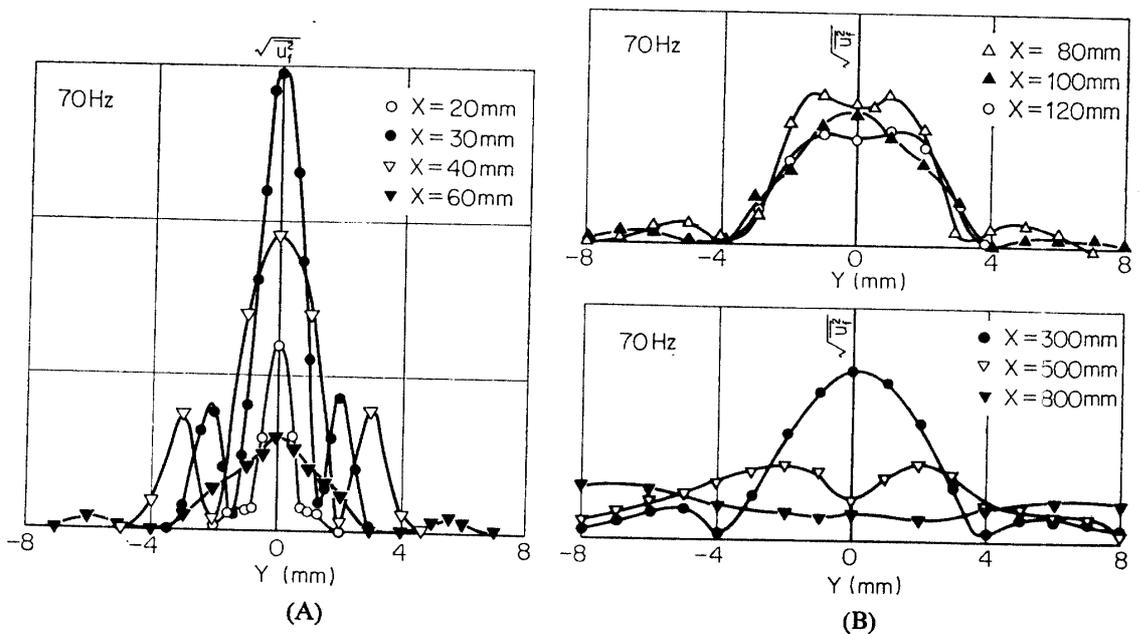
FIG. 5-17. Distribution of 70 Hz-component with sound of 630 Hz and 700 Hz. Ordinate scale is arbitrary. Relative values are expressed correctly.
