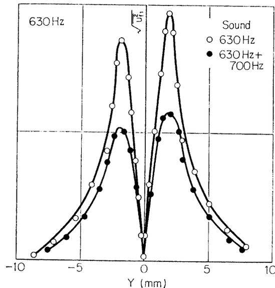
FIG. 5-4. Distribution of root-mean-square of 630 Hz-fluctuation with sound of single frequency (630 Hz) and two frequencies (630 Hz + 700 Hz).  $X=40$  mm. Ordinate scale is arbitrary.
