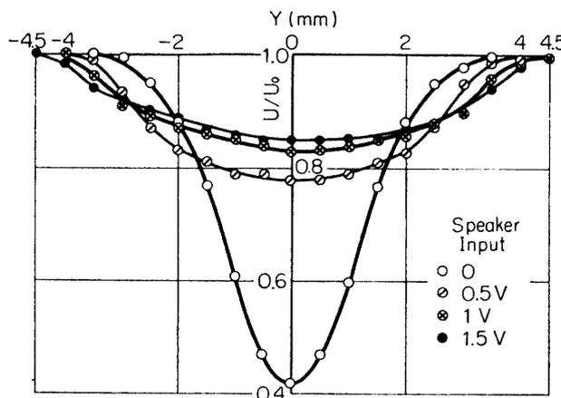
FIG. 4-2. Mean-velocity distribution with and without sound of 630 Hz,  $X=40$  mm,  $U_0=10$  m/s.
