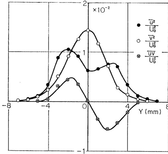
FIG. 3-10. Distributions of  $\overline{u^2}$ ,  $\overline{v^2}$  and  $\overline{uv}$ , natural transition,  $X=60$  mm.
