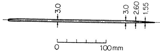
FIG. 2-2. Dimensions of wake-producing plate. All dimensions in millimeters.
