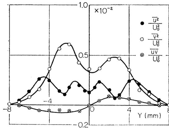
FIG. 3-13. Distributions of  $\overline{u^2}$ ,  $\overline{v^2}$  and  $\overline{uv}$ , natural transition,  $X=120$  mm.
