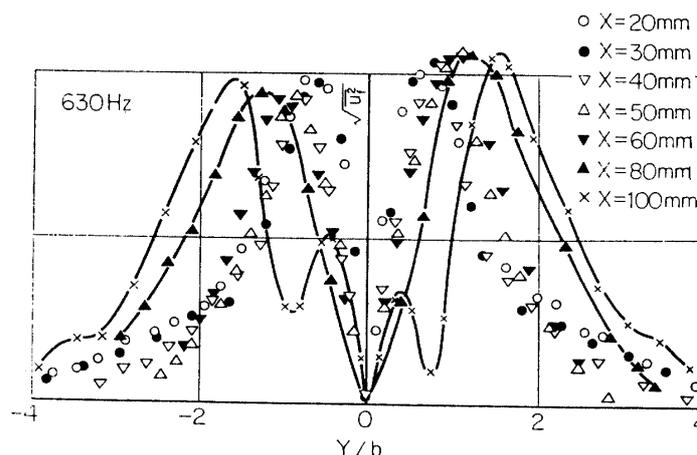
FIG. 6-6. Non-dimensional plot of distribution of 630 Hz-component with sound of 630 Hz. Abscissa is non-dimensionalized by half breadth,  $b$  and ordinate is normalized by mean of two peak values.
