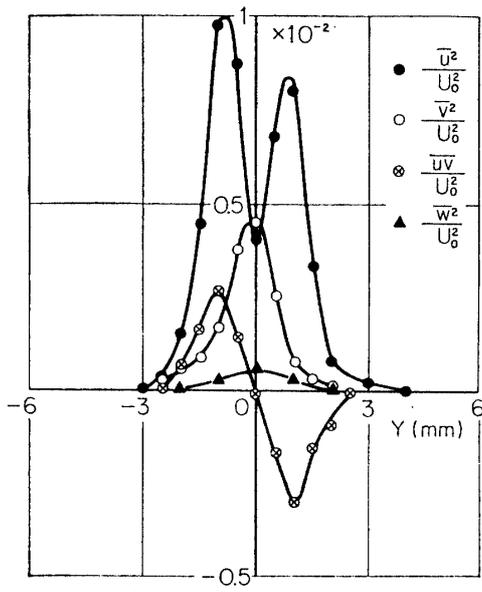
FIG. 3-9. Distributions of  $\overline{u^2}$ ,  $\overline{v^2}$ ,  $\overline{w^2}$ , and  $\overline{uv}$ , natural transition,  $X=40$  mm.
