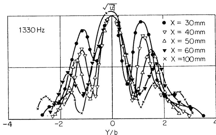
FIG. 6-10. Non-dimensional plot of distribution of 1330 Hz-component with sound of 630 Hz and 700 Hz.
