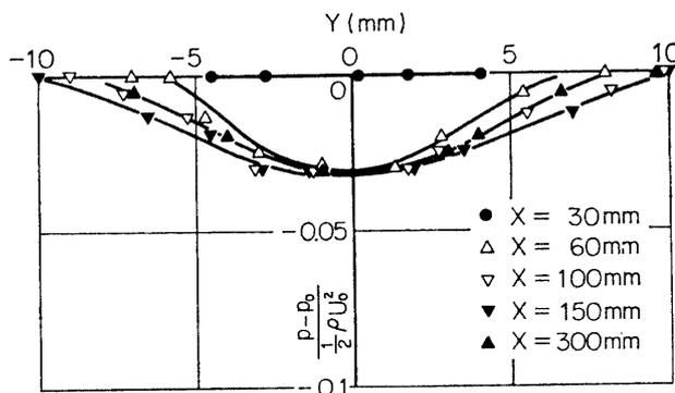
FIG. 3-4. Static-pressure distribution at five  $X$ -stations  $p$ : pressure in wake,  $p_0$ : pressure in free stream. Natural transition.
