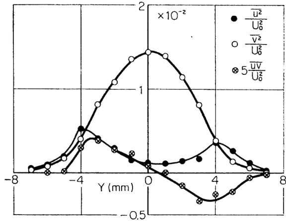
FIG. 4-17. Distributions of  $\overline{u^2}$ ,  $\overline{v^2}$  and  $\overline{uv}$  with sound of 630 Hz.  $X=60$  mm.
