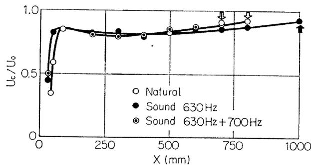
FIG. 5-8. Streamwise variation of velocity on the center line,  $U_c$  in three cases.  $U_0=100$  m/s. Arrows indicate  $X$ -stations where wave-forms of velocity fluctuations become random.
