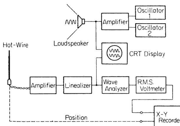
FIG. 2-6. Block diagram of hot-wire system.
