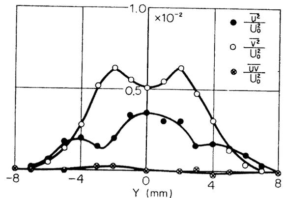
FIG. 5-28. Distributions of  $\overline{u^2}$ ,  $\overline{v^2}$  and  $\overline{uv}$  with sound of 630 Hz and 700 Hz.  $X=120$  mm.
