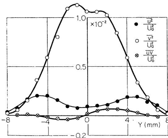
FIG. 4-18. Distributions of  $\overline{u^2}$ ,  $\overline{v^2}$  and  $\overline{uv}$  with sound of 630 Hz.  $X=80$  mm.
