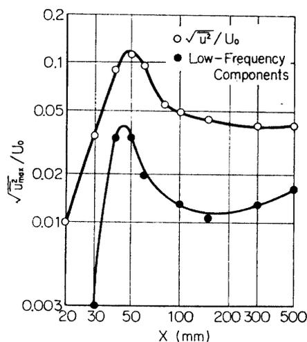
FIG. 8-4. Streamwise variations of maximum values of  $\sqrt{u^2}$  and low-frequency components at each  $X$ -station. Natural transition.
