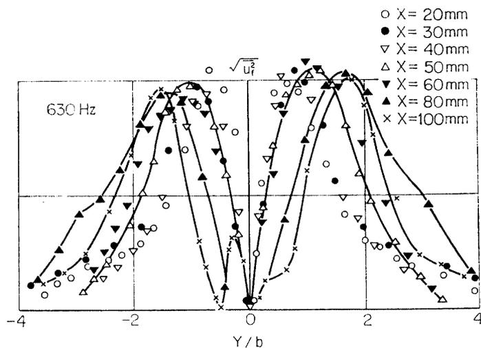
FIG. 6-9. Non-dimensional plot of distribution of 630 Hz-component with sound of 630 Hz and 700 Hz.
