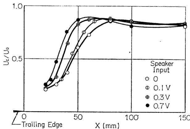
FIG. 4.4. Streamwise variation of velocity on the center line,  $U_c$ , with and without sound 630 Hz.  $U_0=10$  m/s.
