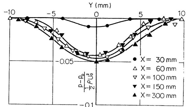
FIG. 4-7. Static-pressure distribution with sound of 630 Hz.  $p$ : pressure in wake,  $p_0$ : pressure in free stream.  $U_0=10$  m/s.
