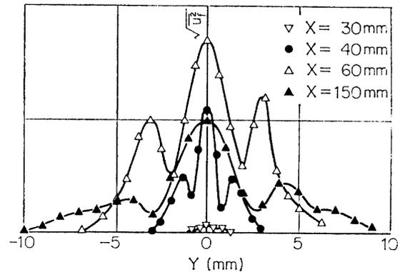
Fig. 3-18. Distribution of root-mean-square of second harmonics (1260 Hz) of  $u$ -fluctuation, natural transition. Ordinate, arbitrary scale.
