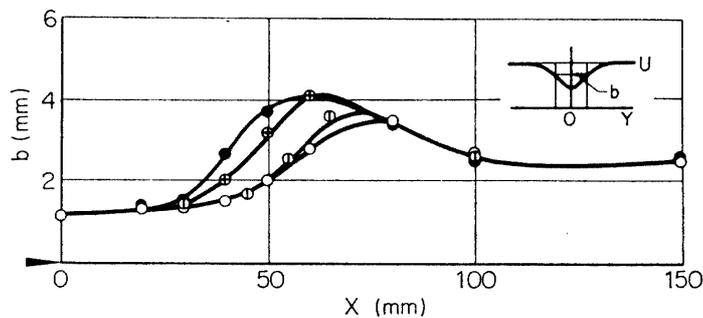
FIG. 4-5. Streamwise variation of half-value breadth,  $b$ , with and without sound of 630 Hz.  $U_0=10$  m/s. For legend, see figure 4-4.
