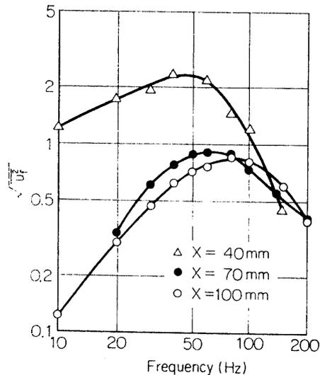
FIG. 8-1. Low-frequency portions of spectra of  $u$ -fluctuation at  $Y=0$ . Natural transition. Ordinate is arbitrary scale.
