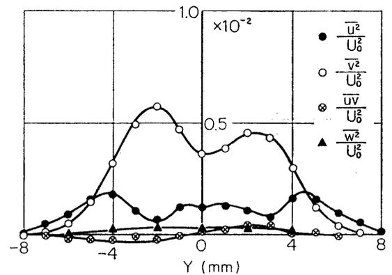
FIG. 3-14. Distributions of  $\overline{u^2}$ ,  $\overline{v^2}$ ,  $\overline{w^2}$  and  $\overline{uv}$ , natural transition,  $X=150$  mm.
