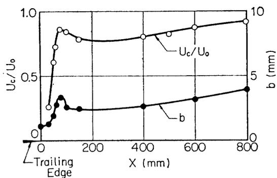
FIG. 3-3. Streamwise variations of non-dimensional velocity on the center line,  $U_c/U_0$  ( $U_0$ : free-stream velocity) and half-value breadth,  $b$  natural transition.
