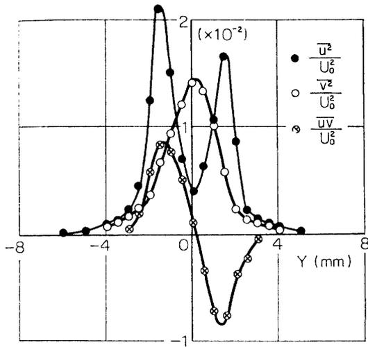
FIG. 4-16. Distributions of  $\overline{u^2}$ ,  $\overline{v^2}$  and  $\overline{uv}$  with sound of 630 Hz.  $X=40$  mm.
