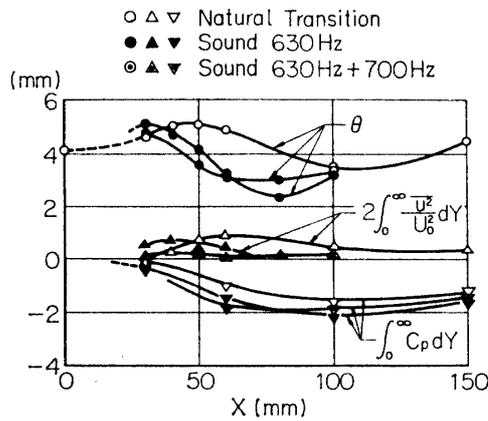
FIG. 7-2. Three terms of momentum flux calculated from experimental date. Natural transition, with sound of 630 Hz and with sound of 630 Hz and 700 Hz.
