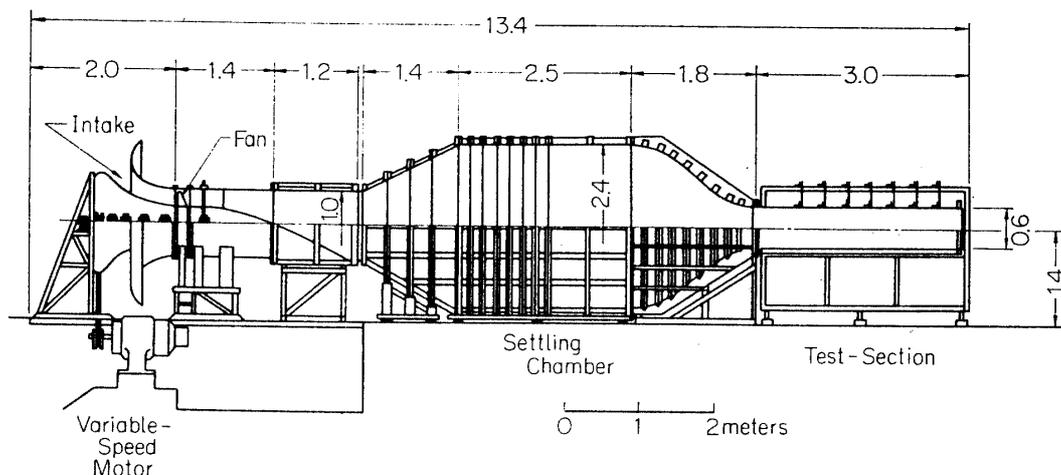
FIG. 2-1. No. 2 Low-Turbulence Wind-Tunnel. Flow, from left to right. All dimensions in meters.
