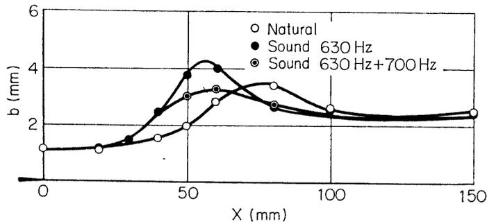
FIG. 5-7. Streamwise variation of half-value breadth,  $b$ , in three cases.  $U_0=10$  m/s.
