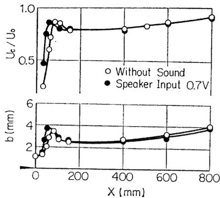
FIG. 4-6. Streamwise variation of velocity on the center line,  $U_c$ , and half-value breadth,  $b$ , with and without sound of 630 Hz.
