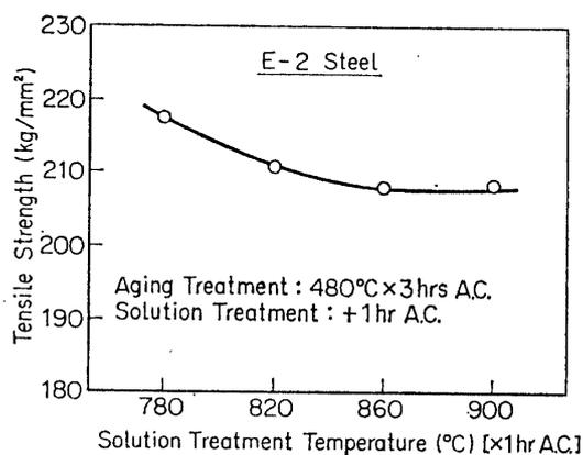
FIG. 1. Effect of solution treatment temperature on tensile strength.
