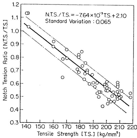
FIG. 9. Results of NASA notch tension test of the air melt materials.
