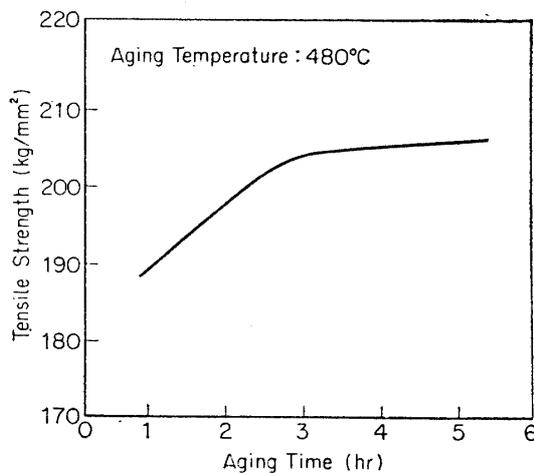
FIG. 3. Effect of aging time on tensile strength (B-1 steel).
