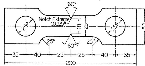
FIG. 8. Specimen of NASA notch tension test.
