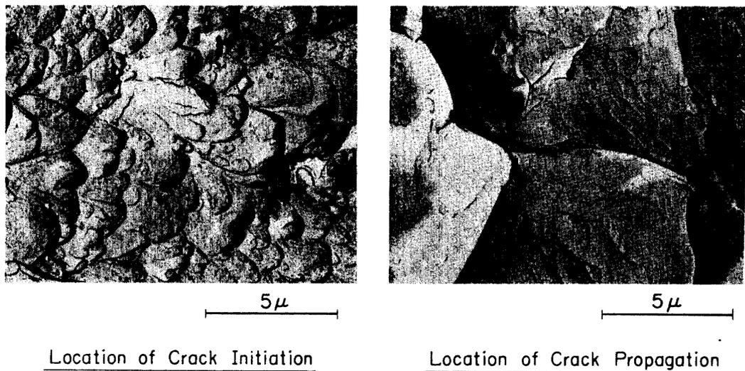
FIG. 28. Electron microscope fractographs of rocket chamber model (E-2 steel).
