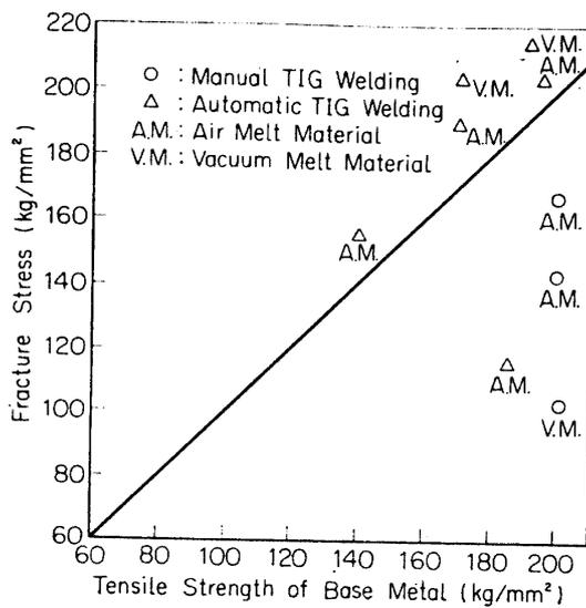
FIG. 25. Tensile strength of base metal vs. fracture stress.
