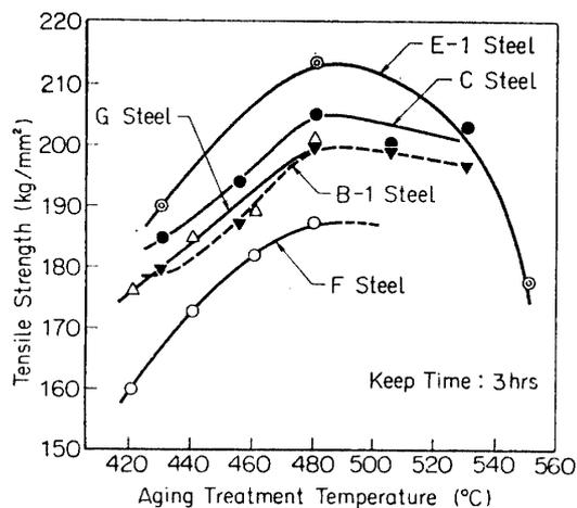
FIG. 2. Effect of aging treatment temperature on tensile strength.
