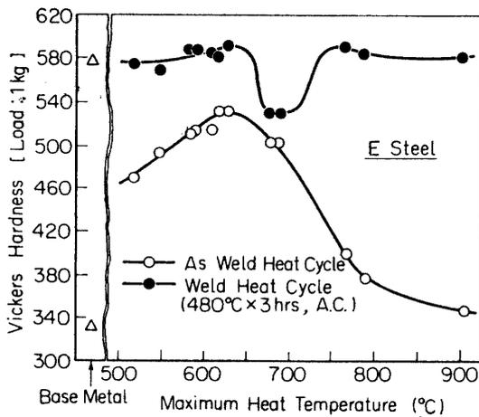
FIG. 18. Maximum heat temperature on simulated weld heat cycle vs. Vickers hardness.
