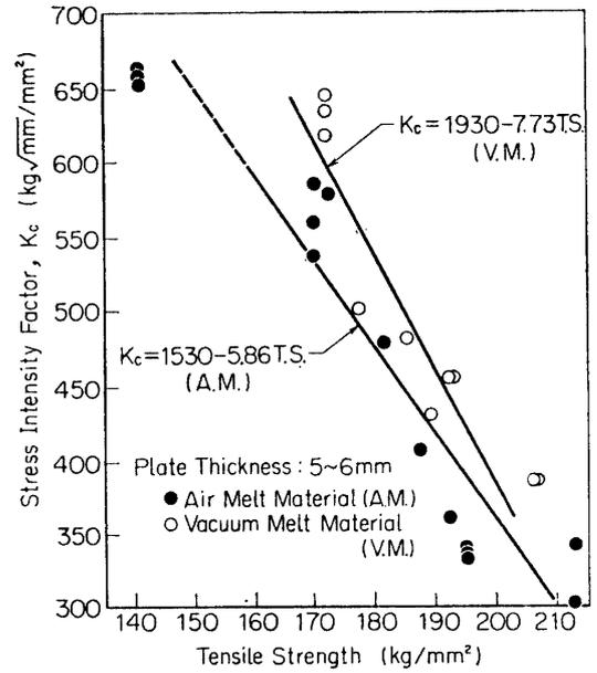
FIG. 13. Tensile strength vs. stress intensity factor ( $K_c$ ).
