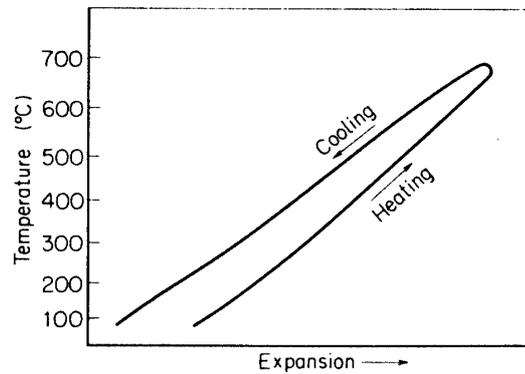
FIG. 19. Heat expansion vs. temperature in simulated test of heat affected zone (maximum heat temperature: 690°C).
