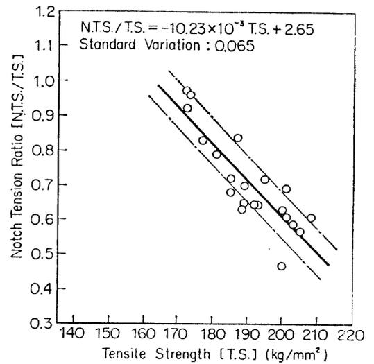
FIG. 10. Results of NASA notch tension test of the vacuum melt materials.
