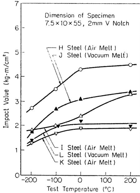
FIG. 6. Results of V-notch Charpy impact test of base metal (average of triplicate tests).
