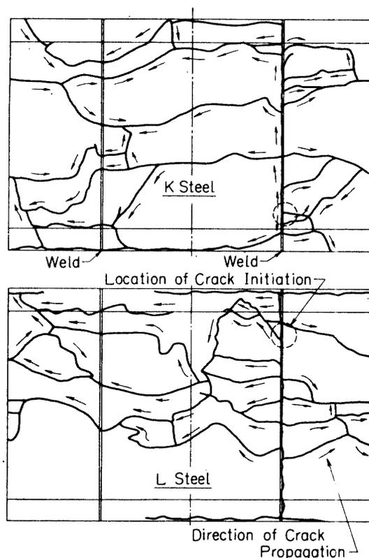
FIG. 24. Deployed view of fracture part of rocket chamber models.
