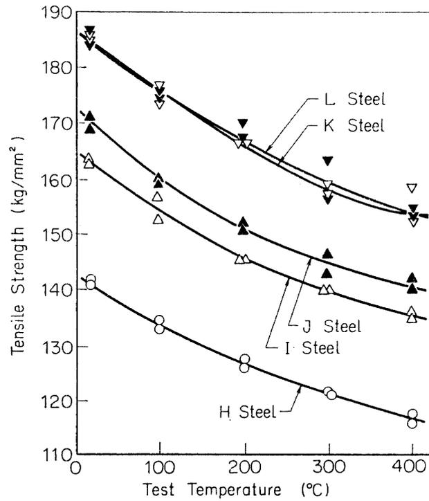
FIG. 5. Examples of the tensile strength of maraging steel at high temperature.
