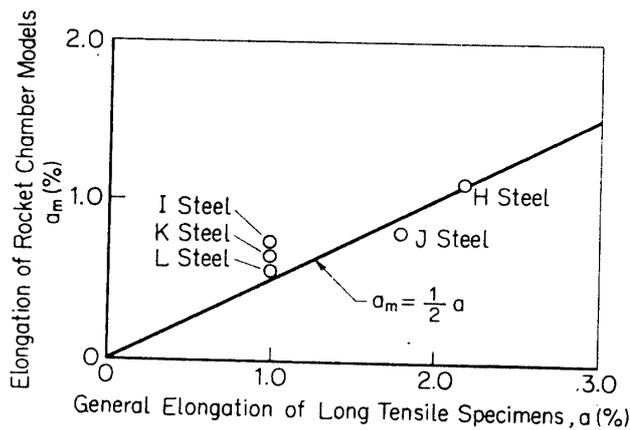
FIG. 27. General elongation of long tensile specimens vs. elongation of rocket chamber models.
