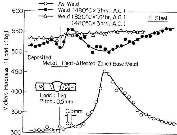
FIG. 17. Distribution of hardness of weldment for E steel.
