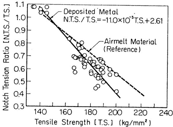
FIG. 16. Results of NASA notch tension test of deposited metal.
