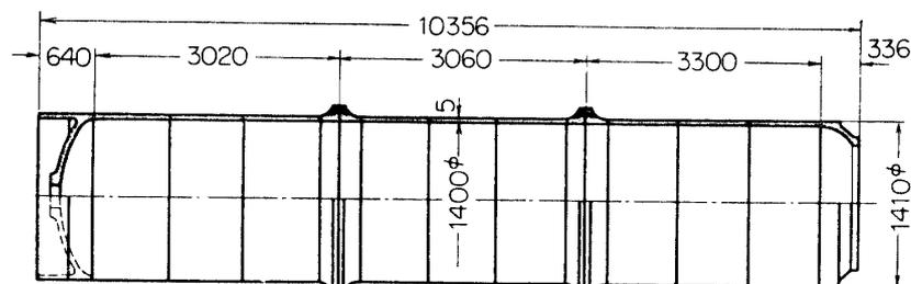
FIG. 29. The sketch of the first stage engine case of Mu rocket.
