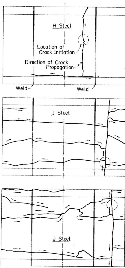
FIG. 23. Deployed view of fracture part of rocket chamber models.
