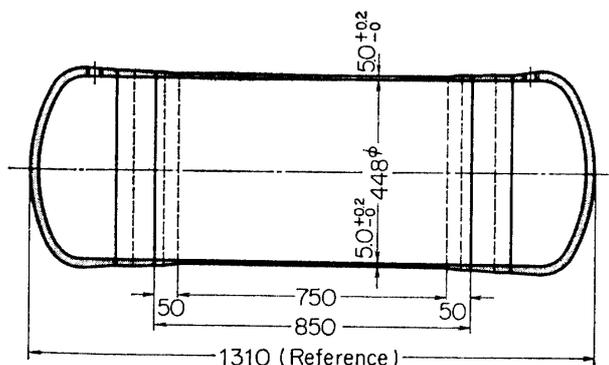
FIG. 21. Dimensions of model vessel.
