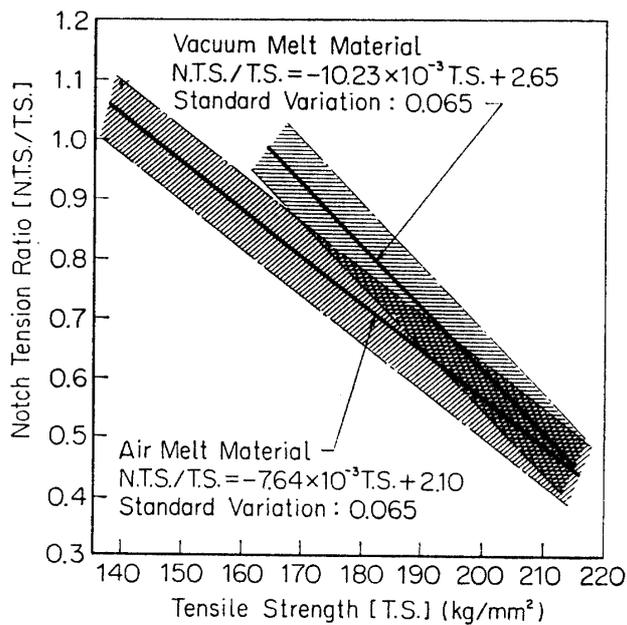
FIG. 11. Results of NASA notch tension test for the air melt materials and vacuum melt materials.
