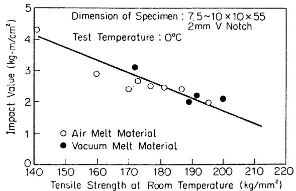
FIG. 7. Tensile strength at room temperature vs. impact value.
