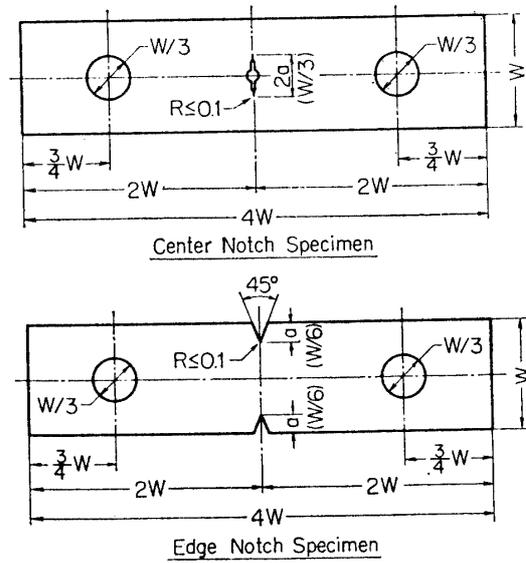
FIG. 12. Specimen of ASTM notch tension test.
