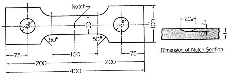
FIG. 14. Specimen of surface notch tension test.
