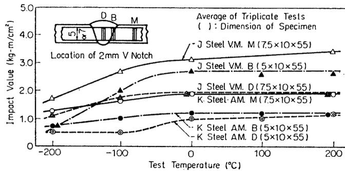
FIG. 15. Charpy transition curves of weldment for precipitation hardenable high strength steel.
