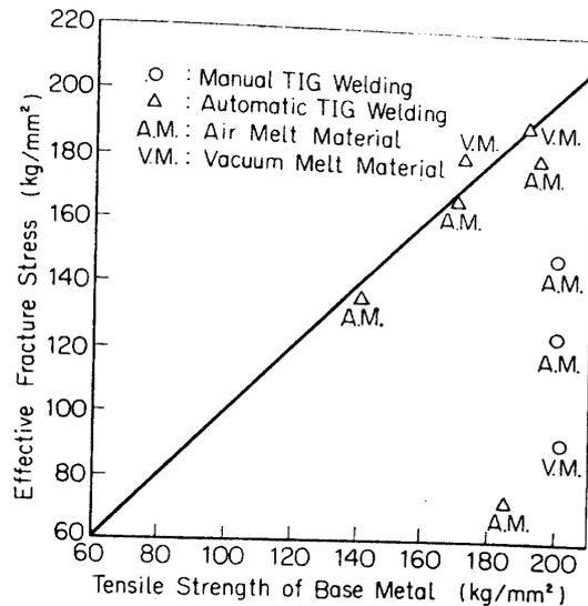
FIG. 26. Tensile strength of base metal vs. effective fracture stress.
