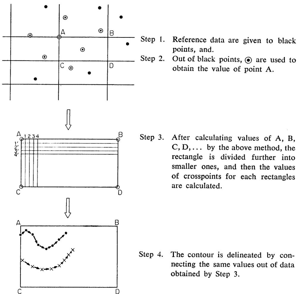
FIG. 3. Method of drawing ECPNL contour.
