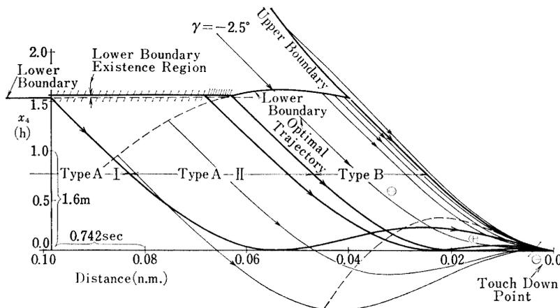
FIG. 4-12. Upper and lower height boundary and corresponding trajectories: aircraft-1, approach-2,  $\gamma_0 = -2.5$  deg.,  $|\delta_e| \leq 0.055$
