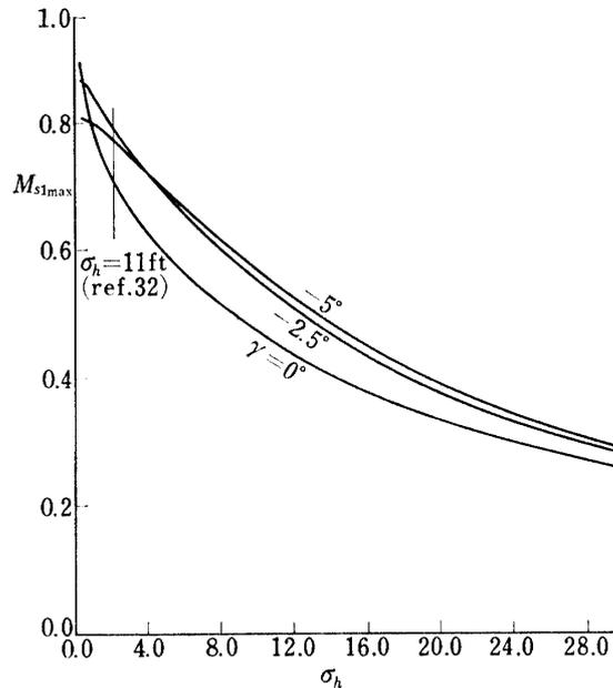
FIG. 5-20. Relation between maximum approach margin  $M_{s1max}$  and standard deviation  $\sigma_h$ : aircraft-1, approach-2,  $|\delta_e| \leq 0.055$ ,  $R=1/3$  n.m.
