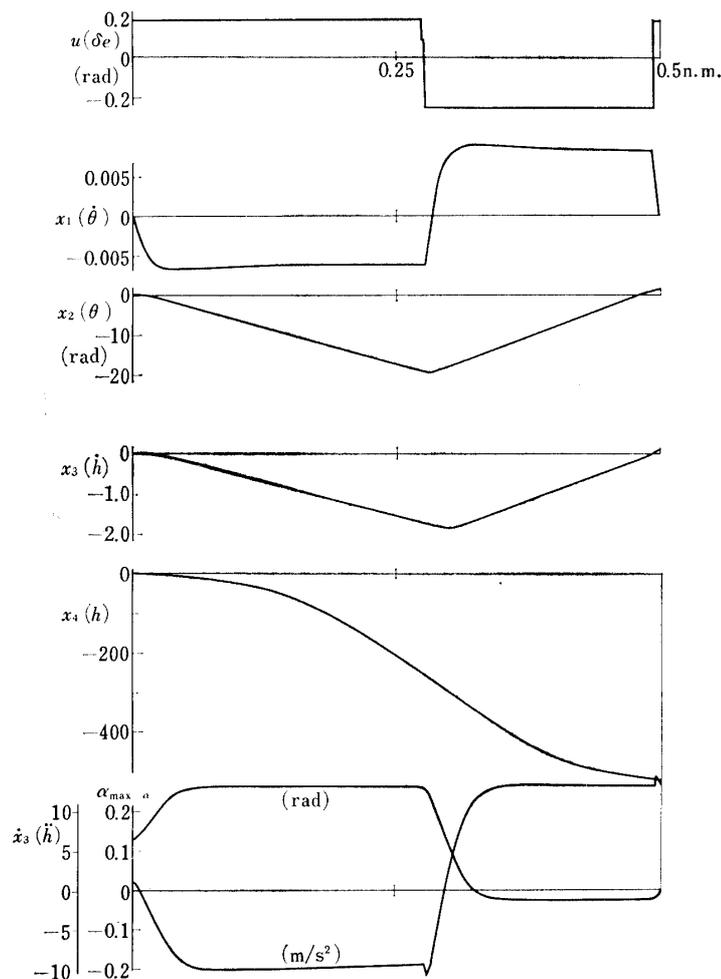
FIG. 4-1. Optimal control and trajectories for maximum initial height: aircraft-1, approach-2,  $U=49.9$  m/s,  $\gamma_0=\theta_0=-2.5$  deg.,  $-0.255 \leq \delta_e \leq 0.195$
