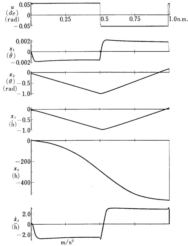
FIG. 5-4. Optimal control trajectories for for upper height boundary: aircraft-1, approach-2,  $U = 49.9$  m/s,  $\gamma_0 = \theta_0 = -2.5$  deg.,  $|\delta_e| \leq 0.055$ ,  $R \leq 1.0$  n.m.
