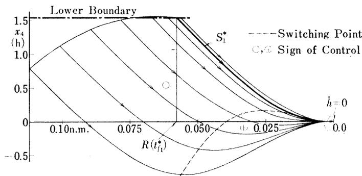
FIG. 4-7. Optimal trajectories which enter into ground tangentially and give maximum initial height: aircraft-1, approach-2,  $\gamma_0 = \theta_0 = -2.5$  deg.,  $|\delta_e| \leq 0.055$ ,  $R \leq 1/9$  n.m.
