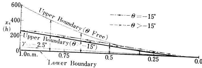
FIG. 5-10. Controllable height boundary with attitude constraint for  $\gamma_0 = -2.5$  deg. (continued)
