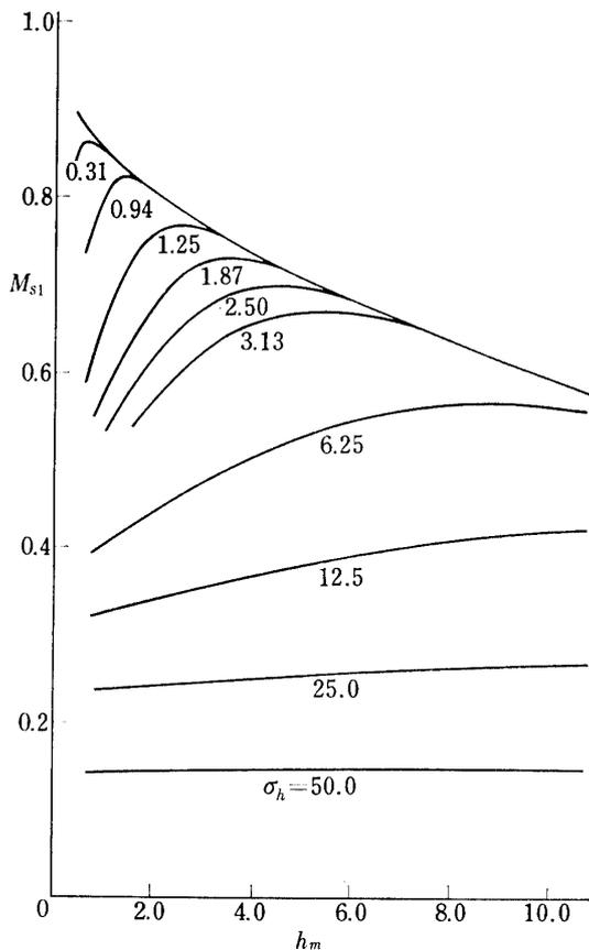
FIG. 5-17. Relation between approach margin  $M_{s1}$  and objective height  $h_m$  at  $R=1/3$  n.m. with respect to standard deviation  $\sigma_h$ : aircraft-1, approach-2,  $|\delta_e| \leq 0.055$ ,  $\gamma_0=0.0$  deg. (continued)
