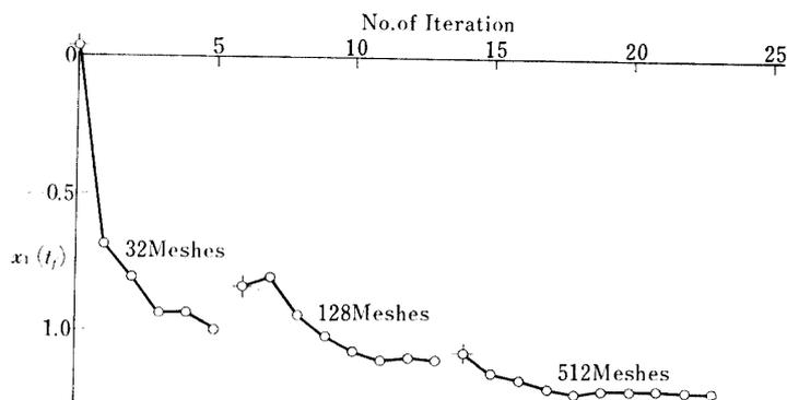
FIG. 3-6. Aspect of convergence of TPO method in Example 2
