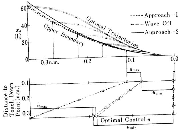
FIG. 5-12. Effect of flight phases in approach: aircraft-1,  $U=49.9$  m/s,  $|\delta_e| \leq 0.055, \gamma_0 = -2.5$  deg.
