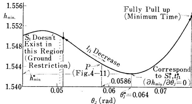
FIG. 4-9. Relation of  $\theta_f$  and  $h_{min}$  which gives  $S_1$ : aircraft-1, approach-2,  $\gamma_0 = -2.5$  deg.,  $h(t_f) = 0.0$ ,  $|\delta_e| \leq 0.055$
