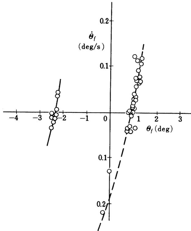
FIG. 5-5. Aircraft attitude and its rate of change at the touch down point: aircraft-1,  $\gamma_0=0.0\sim-5.0$  deg.,  $R\leq 1.0$  n.m.,  $|\delta_e|\leq 0.055$
