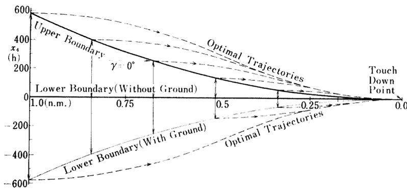
FIG. 5-1. Controllable height boundary and corresponding trajectories for  $\gamma_0=0.0$  deg.: aircraft-1, approach-2,  $U=49.9$  m/s,  $|\delta_e| \leq 0.055$ ,  $h(t_f) = -0.3$  m/s (continued)
