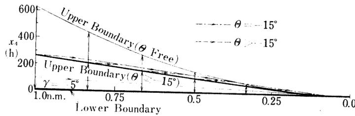
FIG. 5-11. Controllable height boundary with attitude constraint for  $\gamma_0 = -5.0$  deg. (concluded)
