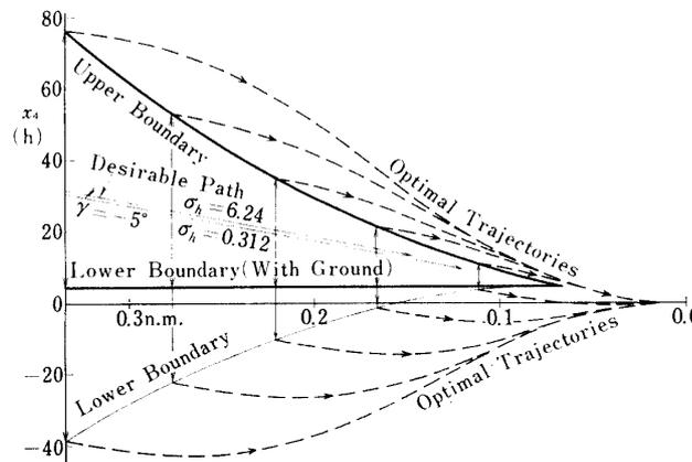
FIG. 5-8. Controllable height boundary and corresponding trajectories for  $\gamma_0 = -5.0$  deg. and  $R = 1/3$  n.m. (concluded)
