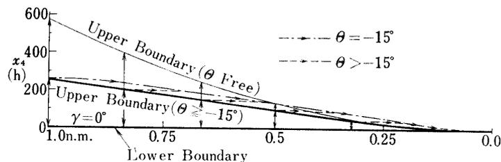
FIG. 5-9. Controllable height boundary with attitude constraint for  $\gamma_0 = 0.0$  deg.: aircraft-1, approach-2,  $U = 49.9$  m/s,  $|\delta_e| \leq 0.055$ ,  $h(t_f) = -0.3$  m/s (continued)
