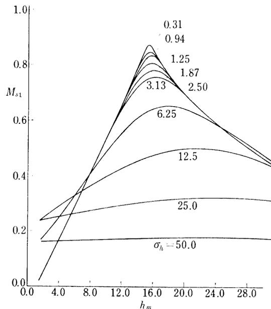
FIG. 5-18. Relation between approach margin  $M_{s1}$  and objective height  $h_m$  at  $R=1/3$  n.m. with respect to standard deviation  $\delta_h: = -2.5$  deg. (continued)
