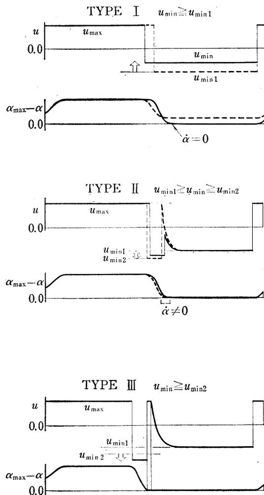
FIG. 4-5. Classification of optimal solution with respect to control limit
