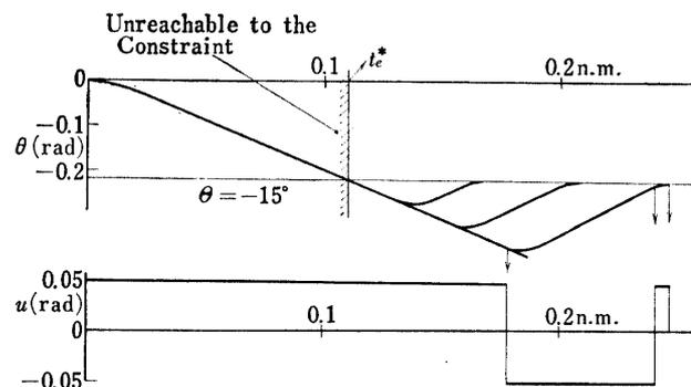
FIG. 4-2. Optimal trajectories which enter into attitude constraint smooth:  $\min h$ , aircraft-1, approach-2,  $\gamma_0 = \theta_0 = -2.5$  deg.
