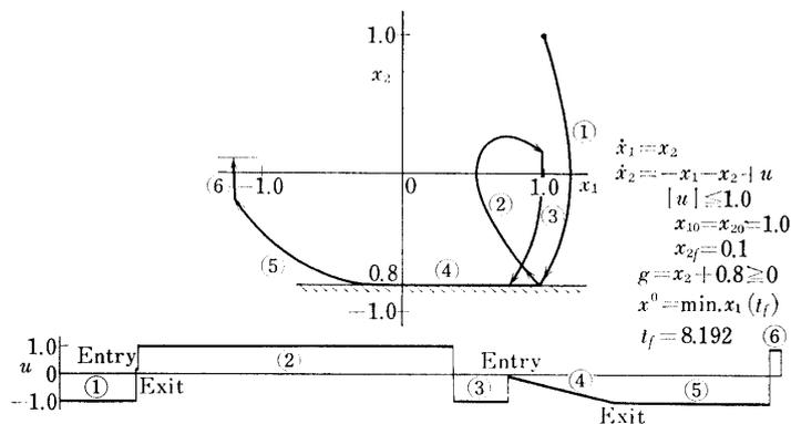
FIG. 3-5. Numerical example of TPO method in state constrained case: converged trajectory and control
