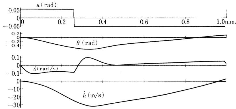
FIG. 5-13. Optimal control and trajectories giving upper height boundary for aircraft-2:  $\gamma_0 = -2.5$  deg.,  $R = 1.0$  n.m.
