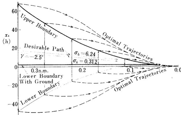
FIG. 5-7. Controllable height boundary and corresponding trajectories for  $\gamma_0 = -2.5$  deg. and  $R = 1/3$  n.m. (continued)
