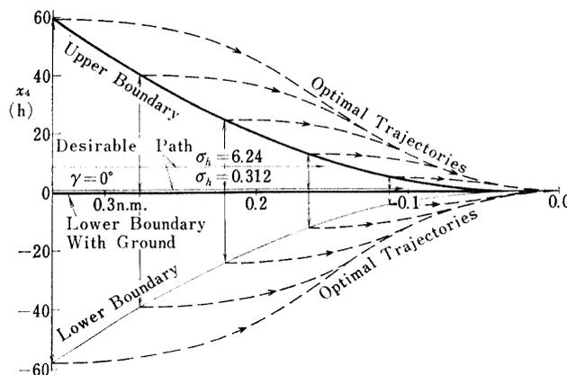
FIG. 5-6. Controllable height boundary and corresponding trajectories for  $\gamma_0=0.0$  deg. and  $R=1/3$  n.m.: aircraft-1, approach-2,  $U=49.9$  m/s,  $|\delta_e|\leq 0.55$ ,  $\dot{h}(t_f)=-0.3$  m/s (continued)
