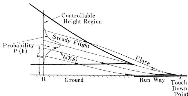
FIG. 5-16. Controllable height region and capable steady approach time  $t_s$
