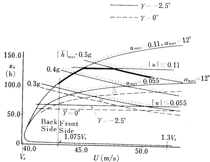
FIG. 5-15. Controllable height regions related to approach velocity, acceleration limits and control limits: aircraft-1, approach-2,  $\gamma_0 = -2.5$  deg.,  $\alpha_{\max} = 12$  deg.,  $R = 1/3$  n.m.
