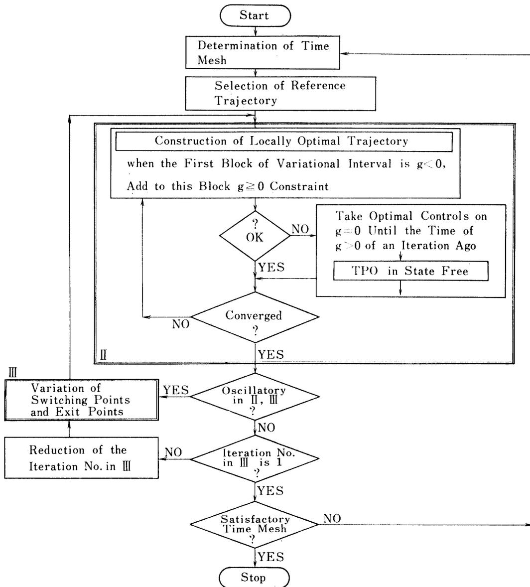
FIG. 3-3. Flow chart of TPO method in state constrained case
