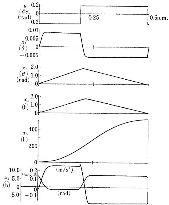
FIG. 4-6. Optimal control and trajectories for minimum initial height: aircraft-1, approach-2,  $U=49.9$  m/s,  $\gamma_0 = \theta_0 = -2.5$  deg.,  $-0.255 \leq \delta_e \leq 0.195$
