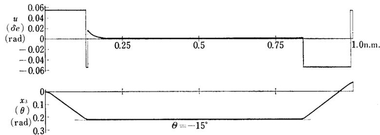
FIG. 4-4. Optimal control and trajectory which gives upper height gives upper height boundary in attitude constrained case: aircraft-1, approach-2,  $U = 49.9$  m/s,  $\gamma_0 = \theta_0 = -2.5$  deg.,  $|\delta_e| \leq 0.055$
