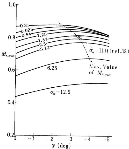
FIG. 5-21. Relation between maximum approach margin  $M_{s1max}$  and approach angle  $\gamma$ : aircraft-1, approach-2,  $|\delta_e| \leq 0.055$ ,  $R=1/3$  n.m.
