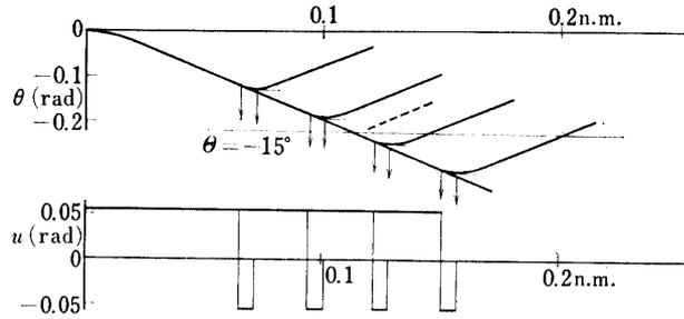
FIG. 4-3. Construction of optimal trajectory which enters into attitude constraint smooth and does not violate the constraint before the entry: min  $h$ , aircraft-1, approach-2,  $\gamma_0 = \theta_0 = -2.5$  deg.
