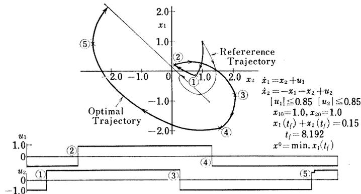
FIG. 3-2. Numerical example of TPO method: converged trajectory and controls
