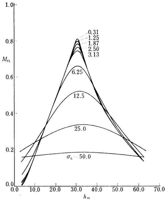
FIG. 5-19. Relation between approach margin  $M_{s1}$  and objective height  $h_m$  at  $R=1/3$  n.m. with respect to standard deviation  $\sigma_h$ :  $\gamma_0 = -5.0$  deg. (concluded)
