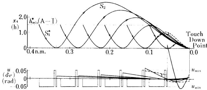
FIG. 4-8. Matching of optimal trajectory  $S_1^*$  and suitable trajectory  $S_2$ : aircraft-1, approach-2,  $\gamma_0 = \theta_0 = -2.5$  deg.,  $|\delta_e| \leq 0.055$
