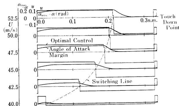
FIG. 5-14. Relation between approach velocity  $U$  and controls giving upper height boundary: aircraft-1, approach-2,  $\gamma_0 = -2.5$  deg.,  $u=0.11$ ,  $\alpha_{\max}=12$  deg.
