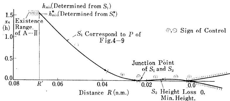
FIG. 11. Existence range of A-II optimal trajectory: aircraft-1, approach-2,  $\gamma_0 = -2.5$ , deg.,  $\theta_J = 0.0586$ ,  $|\delta_e| \leq 0.055$
