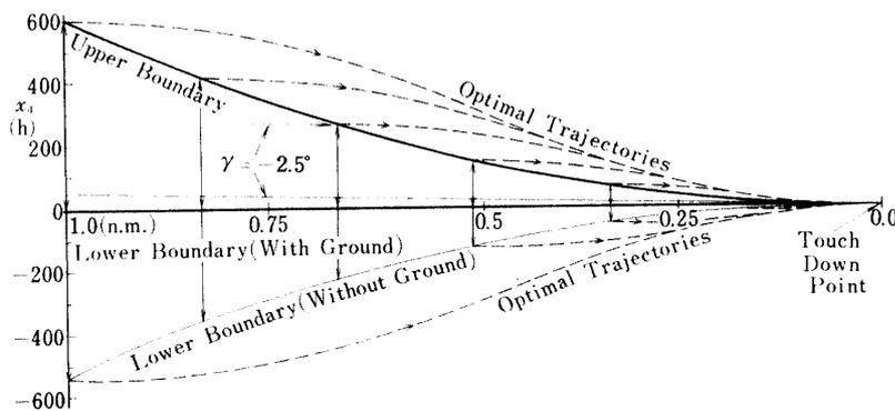
FIG. 5-2. Controllable height boundary and corresponding trajectories for  $\gamma_0 = -2.5$  deg. (continued)
