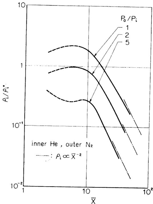
FIG. 5. Density distribution along the jet axis for Case I.
