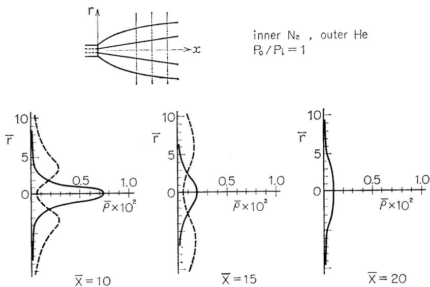
FIG. 9. Density distribution of the gases species in various cross sections normal to the jet axis for Case II with  $P_o/P_i=1$ .
