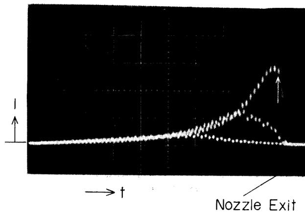
FIG. 4. Simultaneous record of luminosity along the lines parallel to the jet axis (50 m sec/div.).
