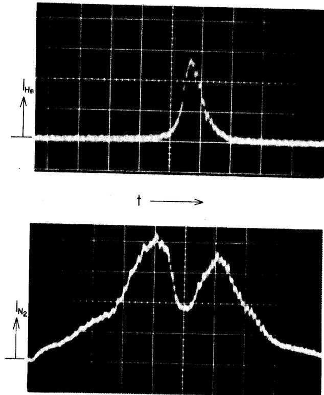
FIG. 7a. Luminosity of the gases species in a cross section normal to the jet axis for Case I (50 m sec/div.).
