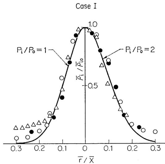
FIG. 13. Cross-sectional density profile of the inner gases species (Case I) (○;  $\bar{x}=10$ , ●;  $\bar{x}=15$ , △;  $\bar{x}=20$ ).
