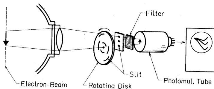
FIG. 2. Optical detection system.
