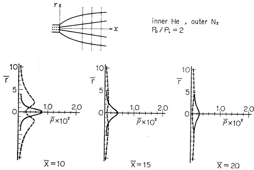
FIG. 10. Density distribution of the gases species in various cross sections normal to the jet axis for Case I with  $P_0/P_i=2$ .
