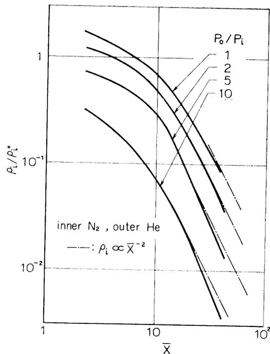
FIG. 6. Density distribution along the jet axis for Case II.
