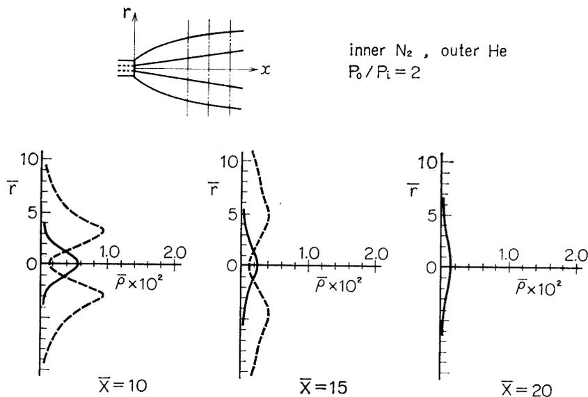
FIG. 11. Density distribution of the gases species in various cross sections normal to the jet axis for Case II with  $P_0/P_i=2$ .
