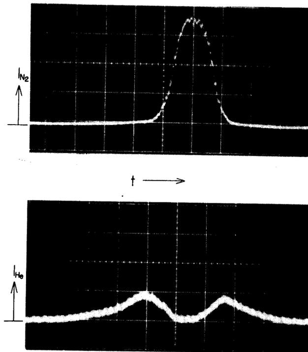
FIG. 7b. Luminosity of the gases species in a cross section normal to the jet axis for Case II (50 m sec/div.).
