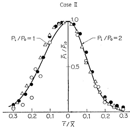
FIG. 14. Cross-sectional density profile of the inner species (Case II) (○;  $\bar{x}=10$ , ●;  $\bar{x}=15$ , △;  $\bar{x}=20$ ).
