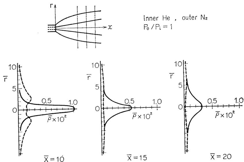
FIG. 8. Density distributions of the gases species in various cross section normal to the jet axis for Case I with  $P_o/P_i=1$ .
