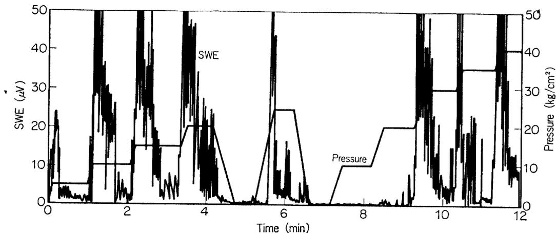
FIG. 13. SWE for the titanium-alloy rocket chamber.
