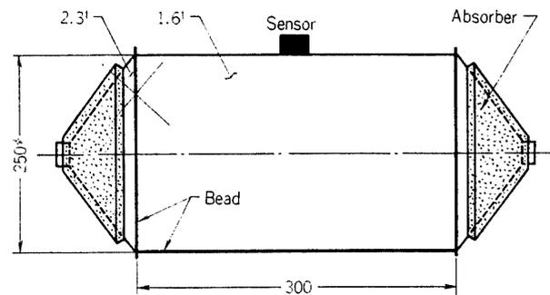
FIG. 5. Model pressure vessel for low-cycle fatigue testing.
