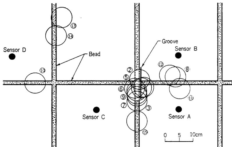
FIG. 9. SWE source locations on the vessel wall.
