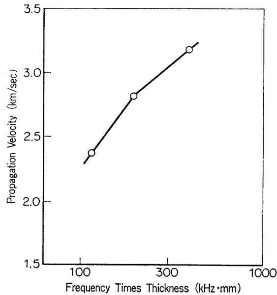
FIG. 8. SWE velocities in a thin plate.
