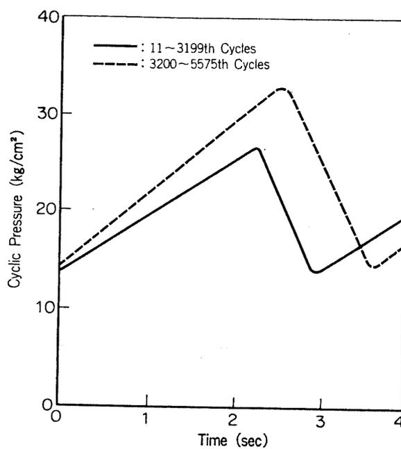
FIG. 11. Cyclic pressures of fatigue testing.
