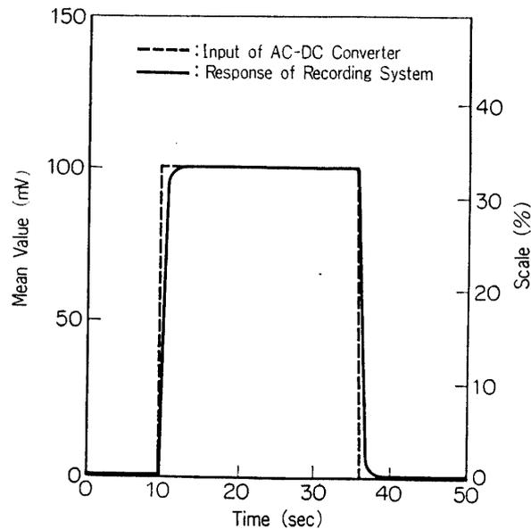
FIG. 3. Transient response of the recording system.
