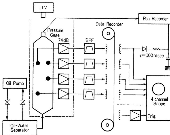
FIG. 1. SWE recording and locating system.
