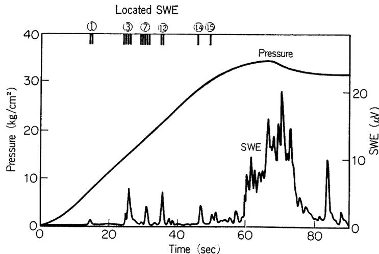
FIG. 7. SWE for hydrostatic testing.
