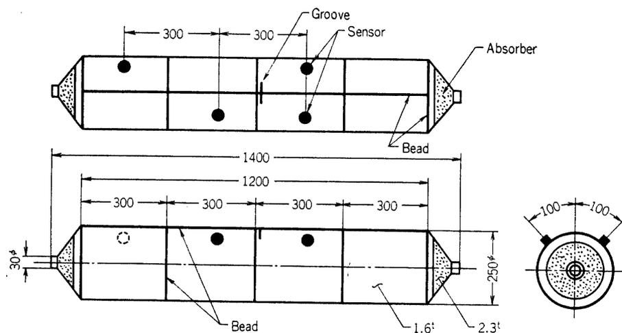
FIG. 4. Model pressure vessel for hydrostatic testing.
