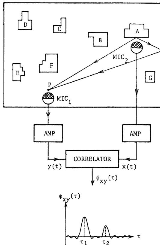
FIG. 1. Block diagram of setup for measuring contributions of noise sources by a correlation technique (K. W. Goff, 1955).
