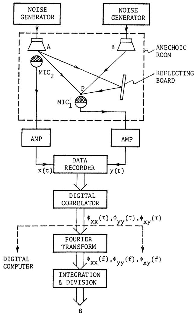
FIG. 4. Block diagram of setup for the preliminary experiments in an anechoic room.
