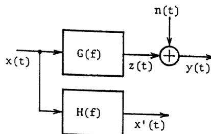
FIG. 3. Block diagram of the acoustic system including the transfer function of a microphone.
