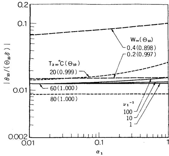
FIG. 4.7. Disturbance temperature at the interface (Water-air,  $T_{1\infty}=100^\circ\text{C}$ ,  $c=0$ ; —,  $T_{2\infty}=60^\circ\text{C}$ ,  $W_{\infty}=0$ ; - - - ,  $\nu_1^{-1}=10$ ,  $W_{\infty}=0$ ; - - - ,  $T_{2\infty}=60^\circ\text{C}$ ,  $\nu_1^{-1}=10$ ).
