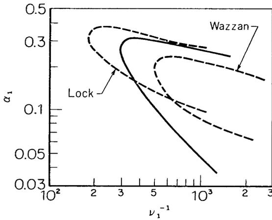
FIG. 5.1. Neutral stability curves of wave-number against Reynolds number (Water-air,  $T_{1\infty}=100^\circ\text{C}$ ,  $T_{2\infty}=20^\circ\text{C}$ ,  $W_\infty=80^\circ\text{C}$ ,  $W_\infty=0$ ).
