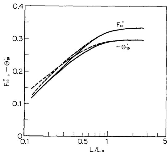
FIG. 3.7. Effect of latent heat of vaporization on coefficients of skin-friction and heat-transfer (Water-air,  $T_{1\infty}=100^\circ\text{C}$ ,  $T_{2\infty}=20^\circ\text{C}$ ,  $W_\infty=0$ ,  $L_0=539 \text{ cal/g}$ ).
