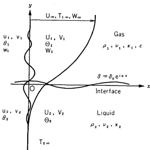
FIG. 4.1. Disturbance fields of laminar boundary-layer flows of gas and liquid having a wavy phase-changing interface.
