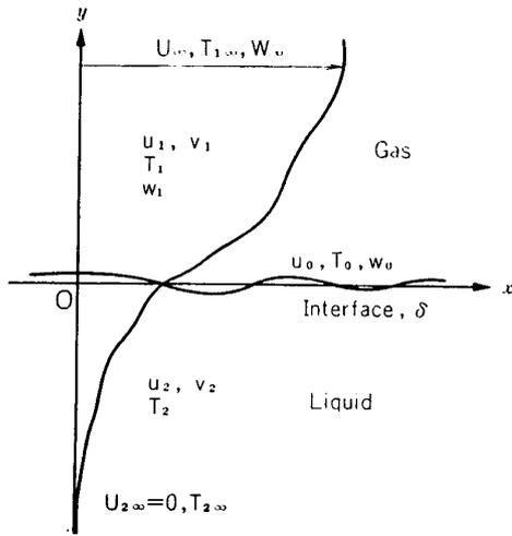
FIG. 2.1. Laminar boundary-layer flows of gas and liquid having a phase-changing interface.
