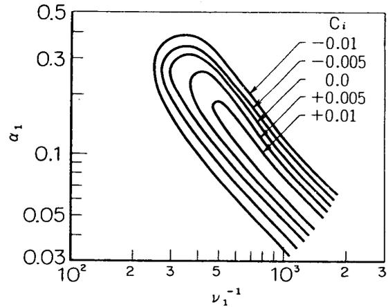
FIG. 5.2. Stability curves (Water-air,  $T_{1\infty}=100^\circ\text{C}$ ,  $T_{2\infty}=80^\circ\text{C}$ ,  $W_\infty=0$ ).
