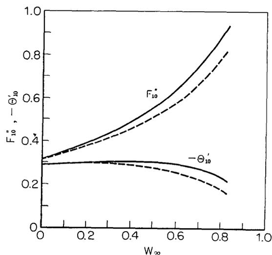
FIG. 3.6. Effect of vapor concentration on coefficients of skin-friction and heat-transfer (Water-air,  $T_{1\infty}=100^\circ\text{C}$ ,  $T_{2\infty}=20^\circ\text{C}$ ).
