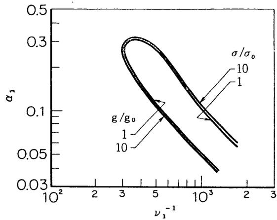
FIG. 5.4. Effect of gravity and surface tension on stability curves (Water-air,  $T_{1\infty}=100^\circ\text{C}$ ,  $T_{2\infty}=80^\circ\text{C}$ ,  $W_\infty=0$ ).
