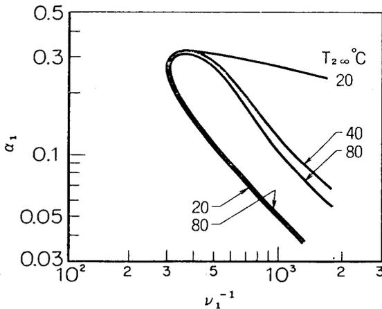
FIG. 5.3. Effect of phase-change (liquid temperature) on stability curves (Water-air,  $T_{1\infty}=100^\circ\text{C}$ ,  $W_\infty=0$ ).
