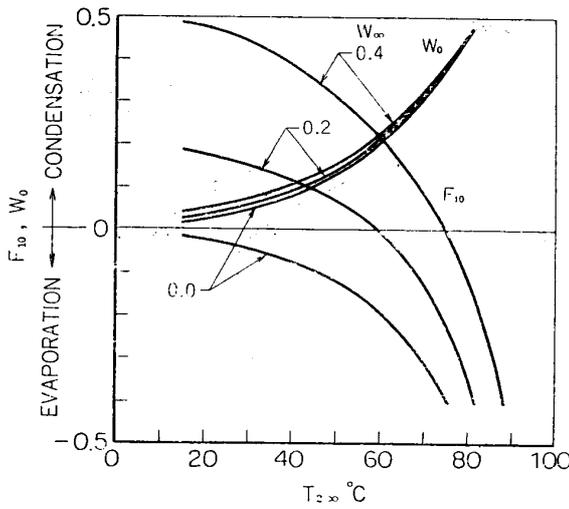
FIG. 3.3. Rate of phase-change and vapor-concentration at infinity (Water-air,  $T_{1\infty}=100^\circ\text{C}$ ).
