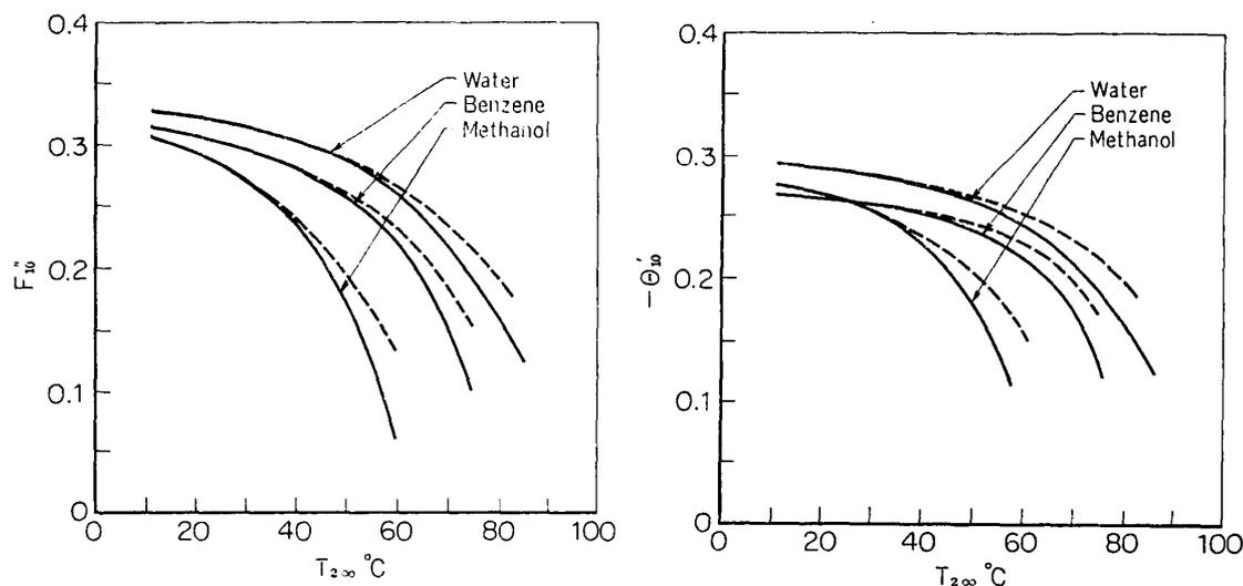
FIG. 3.5. Effect of liquid kind on coefficients of skin-friction and heat-transfer (Air,  $T_{1\infty}=100^\circ\text{C}$ ,  $W_\infty=0$ ).
