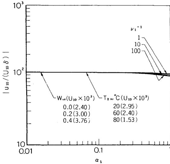
FIG. 4.6. Disturbance  $u$ -velocity at the interface (Water-air,  $T_{1\infty}=100^\circ\text{C}$ ,  $c=0$ ; —,  $T_{2\infty}=60^\circ\text{C}$ ,  $W_{2\infty}=60^\circ\text{C}$ ,  $W_{\infty}=0$ ; - - - ,  $\nu_1^{-1}=10$ ,  $W_{\infty}=0$ ; - - - ,  $T_{2\infty}=60^\circ\text{C}$ ,  $\nu_1^{-1}=10$ ).
