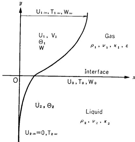
FIG. 3.1. Laminar boundary-layer flows of gas and liquid having a plane phase-changing interface.
