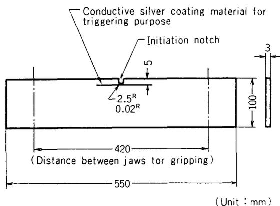
FIG. 4 PMMA specimen dimensions
