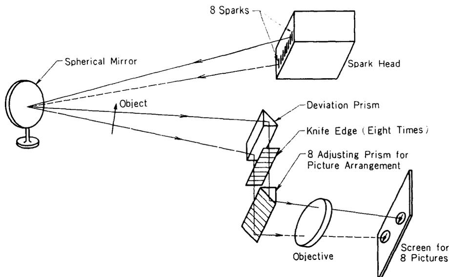
FIG. 1 Cranz-Schardin type multiple spark camera: Diagram showing the optical path and frame separation
