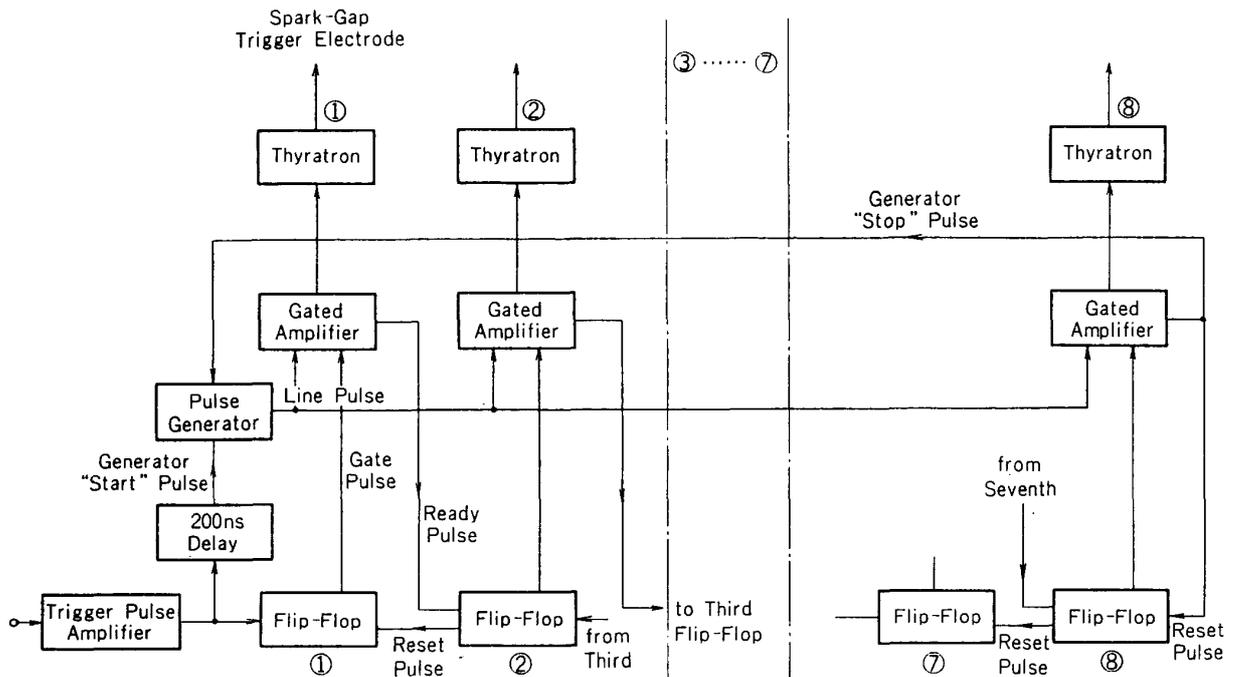
FIG. 2 Block diagram of the time control
