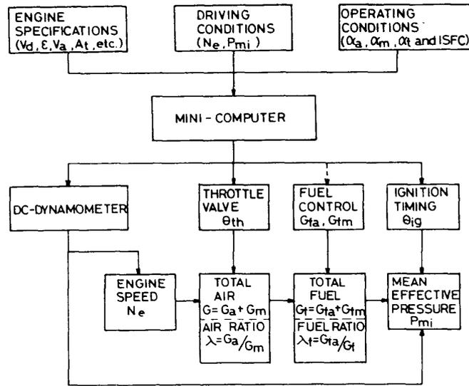
FIG. 5. Block Diagram for Engine Operation
