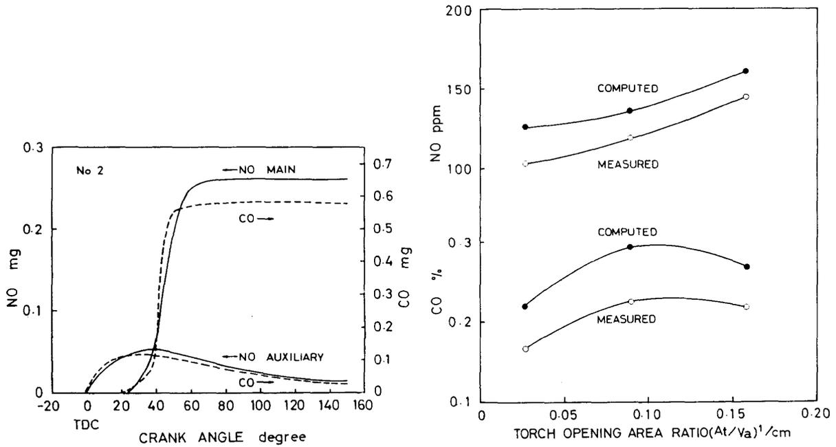
FIG. 8. Computed Emissions of NO & CO in both the Chambers
