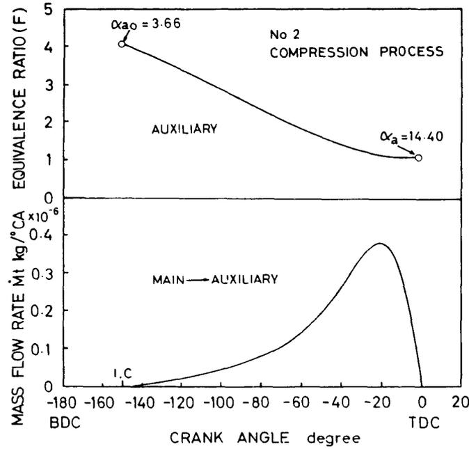
FIG. 7. Computed Equivalence Ratio in the Auxiliary Chamber and Mass Flow Rate through Torch Opening
