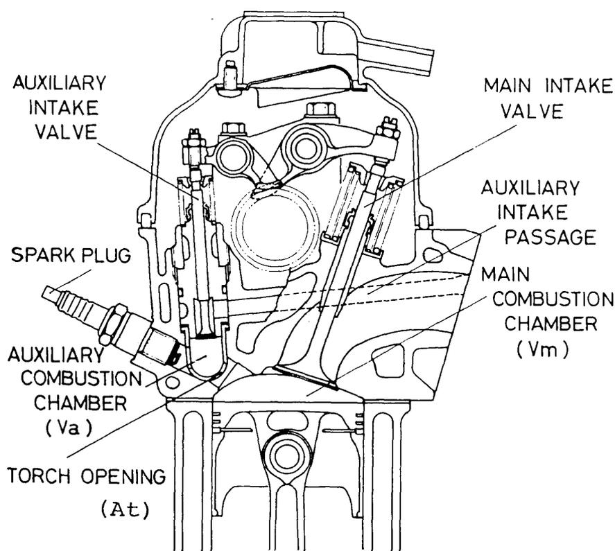
FIG. 4. Engine Cross Section
