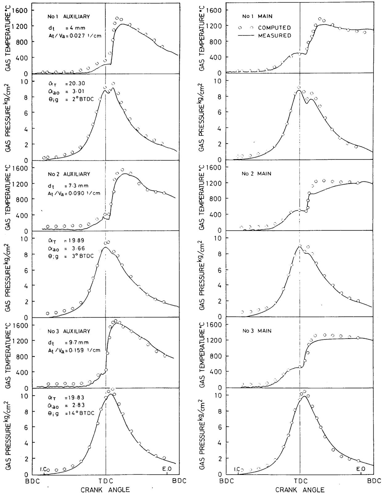
FIG. 6. Computed and Measured Temperature- and Pressure-crankangle Diagrams
