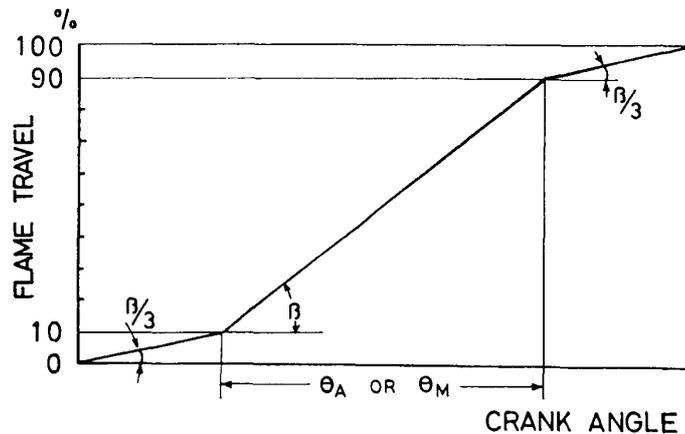
FIG. 2. Simple Burning Model
