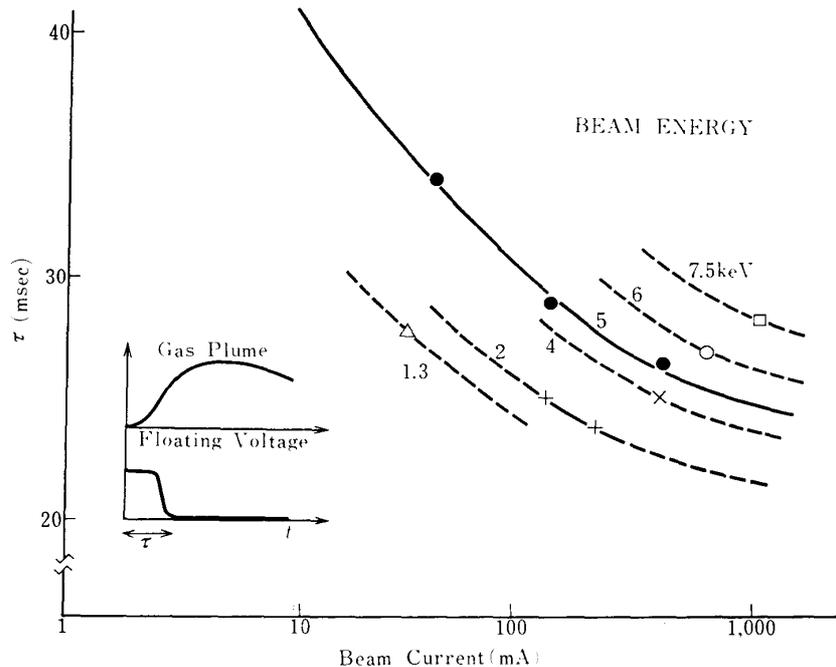
FIG. 3.1.5. (b) Time lag of neutralization by NGP
