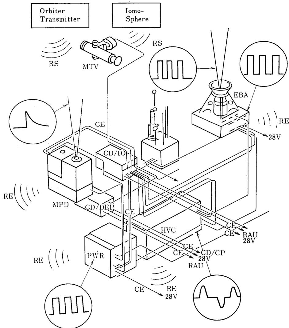
FIG. 3.3.1. Electromagnetic Environment
