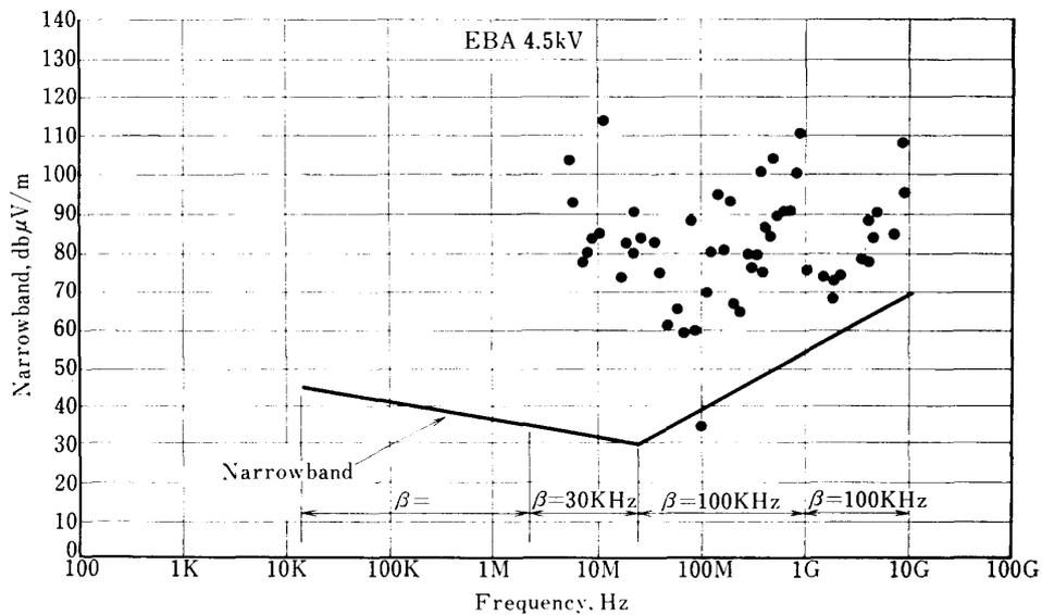
FIG. 3.3.4. (a) Narrow band noise spectrum of EBA
