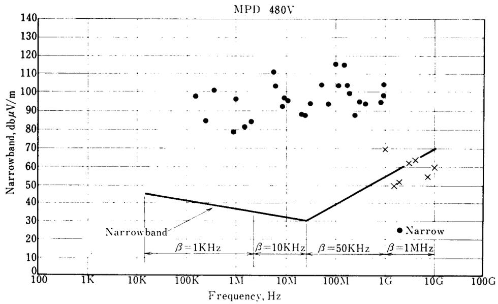
FIG. 3.3.6. (b) Narrowband noise spectrum of MPD
