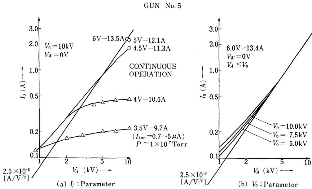
FIG. A-I.  $I_0$  vs  $V_A$  CHARACTERISTICS (GUN No. 5)
