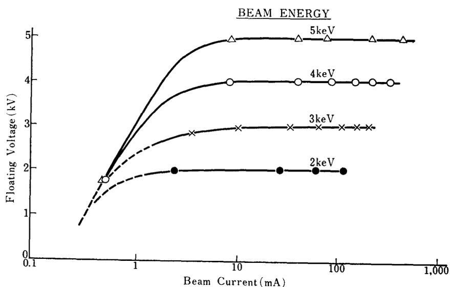
FIG. 3.1.3(b) The dependence of floating voltage on beam current. The floating voltage coincides with the beam acceleration voltage when the beam current is large enough.
