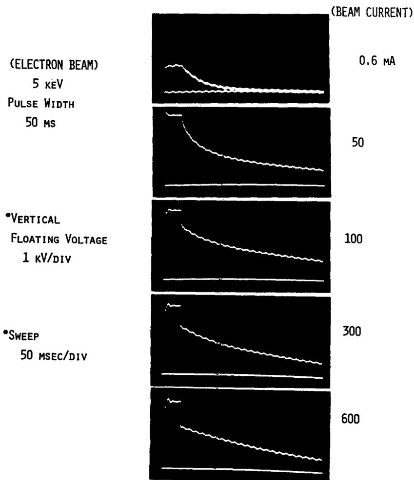
FIG. 3.1.3. (a) EBA Potential in floating mode operation
