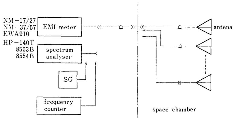
FIG. 3.3.3. (a) Block diagram of RE measuring setup
