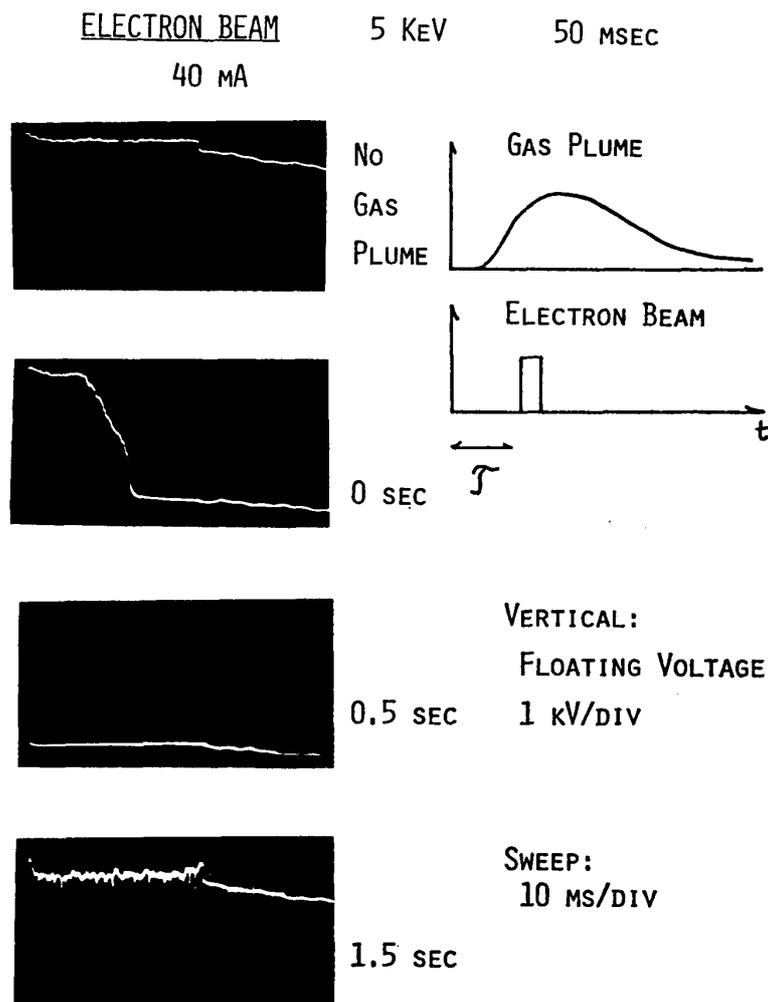
FIG. 3.1.5. (a) Neutralization by NGP operation
