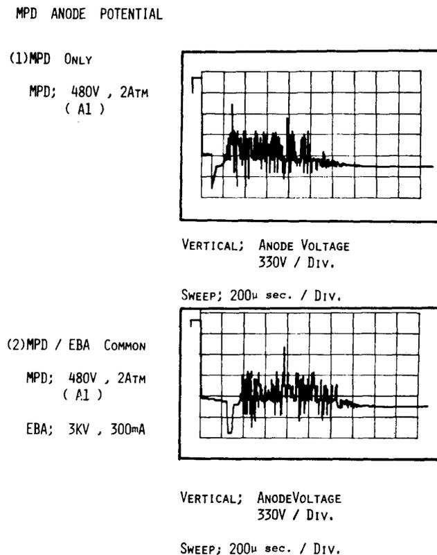
FIG. 3.2.1. MPD Anode Potential
