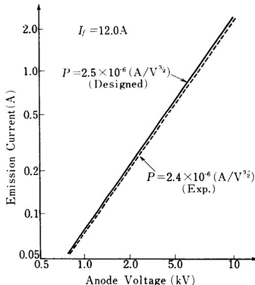
FIG. 3.1.1. EBA Current-Voltage Characteristics
