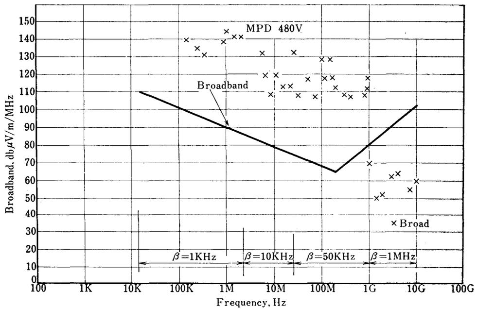
FIG. 3.3.6. (a) Broadband noise spectrum of MPD
