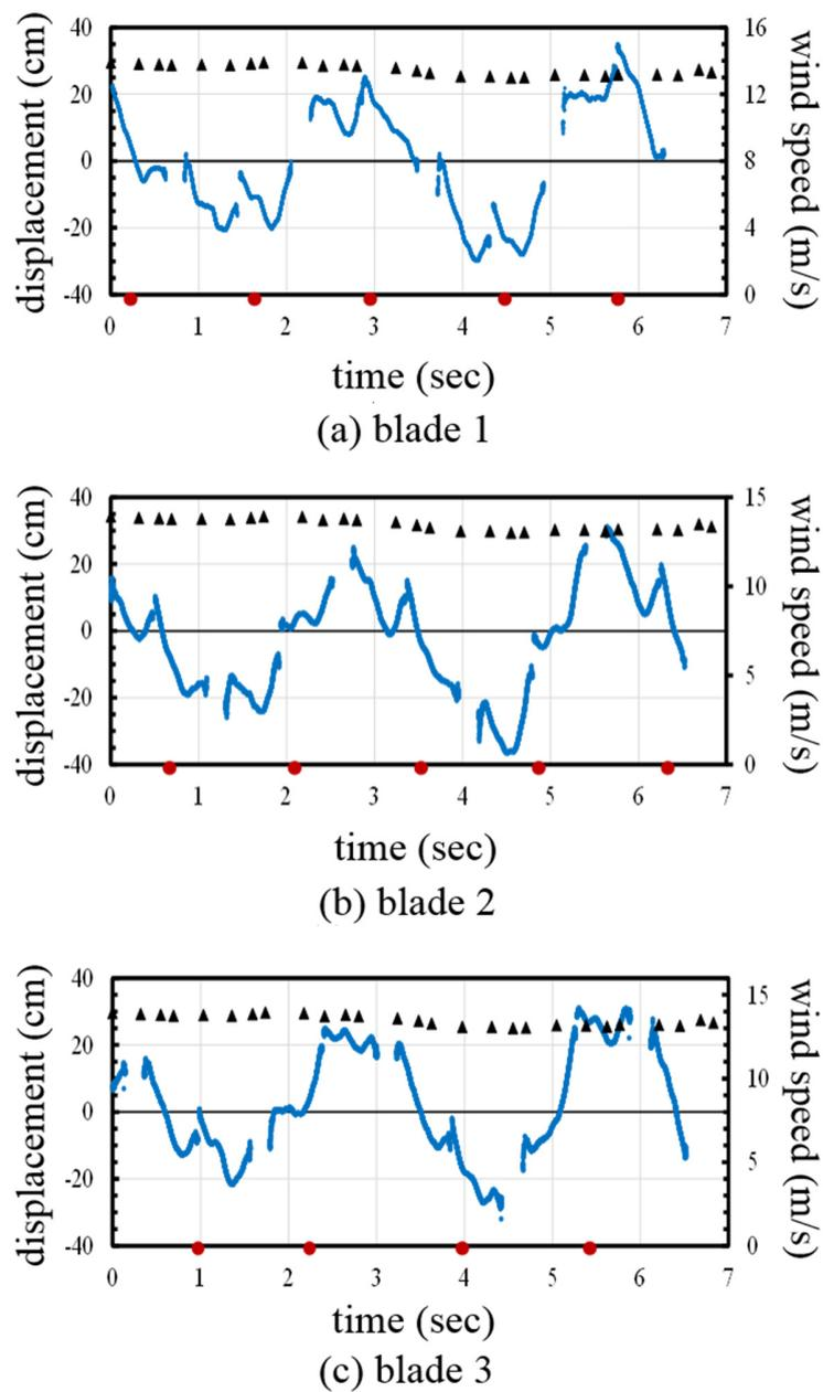
Figure 5: An example of measured blade tip displacements (Dec. 2, 2014).
