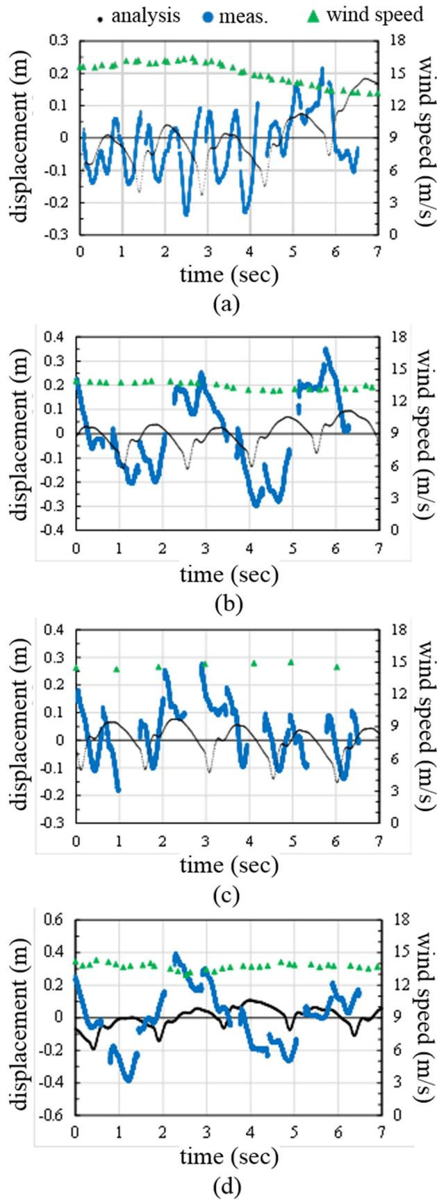
Figure 6: Comparison of measured and analyzed tip displacements.
