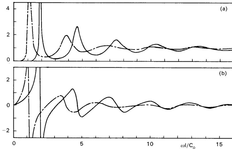
FIG. 11. Acoustic impedance at diffuser inlet. (a) Real part, (b) Imaginary part. — diffuser, - - - constant area duct.
