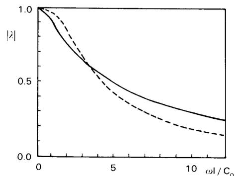
FIG. 12. Convection effect upon reflection coefficient  $\chi$ . —  $M_0 \neq 0$ , - - -  $M_0 = 0$ .
