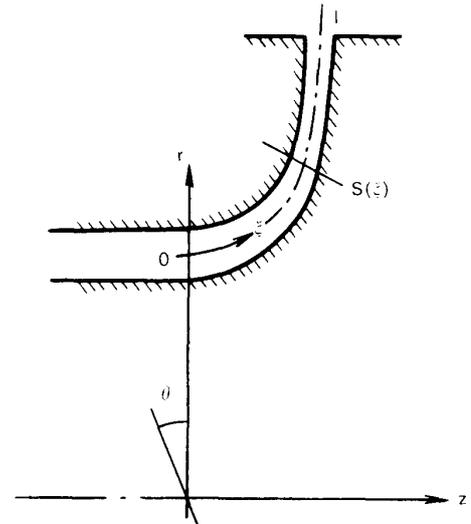
FIG. 4.  $\xi$ -coordinate along diffuser passage
