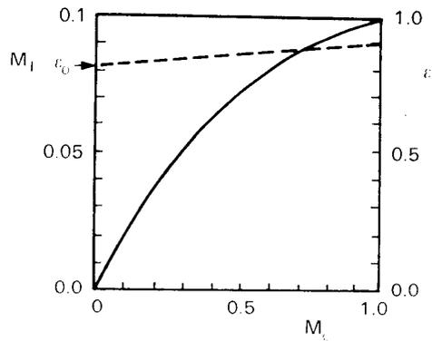
FIG. 7. Outlet Mach number  $M_l$  and deceleration rate  $\epsilon$  versus inlet Mach number  $M_0$ . —  $M_l$ , - - -  $\epsilon$ .
