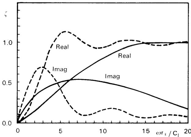
FIG. 9. Radiation impedance of plane wave mode. —  $\zeta_l$  circumferential opening, - - -  $\zeta_l^*$  flanged duct opening.
