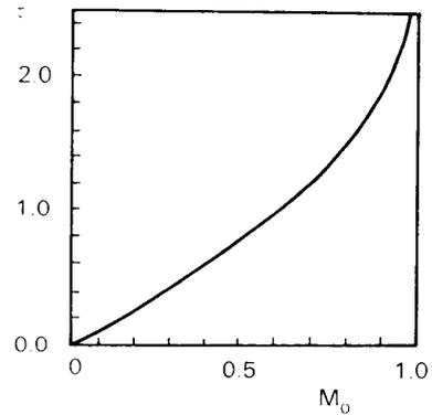
FIG. 8.  $\tau$ -function versus inlet Mach number  $M_0$ .
