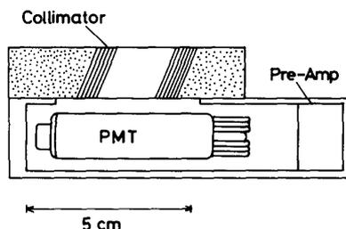
FIG. 2. The side view of the UV sensor.
