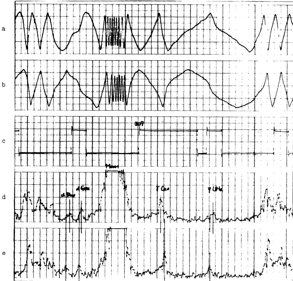
FIG. 5. An example of UV sensor data. The two top figures (a, b) represent the read-out data of the up-down scalers of two UV counters. The two bottom figures represent the counting rates versus the azimuthal angle for two counters.
