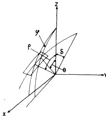
FIG. 6. The geometrical relation of angular variables. The z axis is parallel to the rocket axis. The field of view of the counter is shown by a parallelogram. The counter axis:  $\rho$ ,  $\delta$ ; the star:  $\theta$ ,  $\phi$ .
