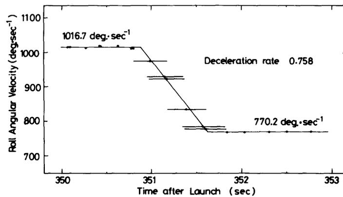
FIG. 8. The roll angular velocity versus time around the time of despin.
