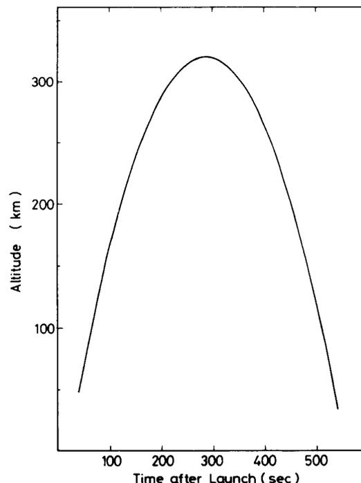
FIG. 4. Flight curve of K-9M-64.
