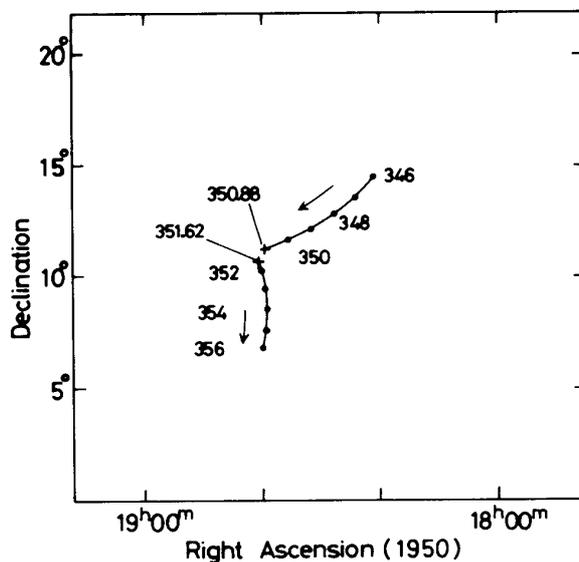
FIG. 9. The trajectory of the rocket axis around the time of despin.
