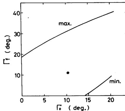
FIG. 1. The precession angle after wire release ( $\Gamma_f$ ) versus that before weight release ( $\Gamma_0$ ) calculated for the spin reduction ratio 0.737. The value of  $\Gamma_f$  lies between its maximum and minimum values indicated, depending on the phase of wire release. The values of  $\Gamma_0$  and  $\Gamma_f$  achieved in the experiment are indicated by a solid circle.
