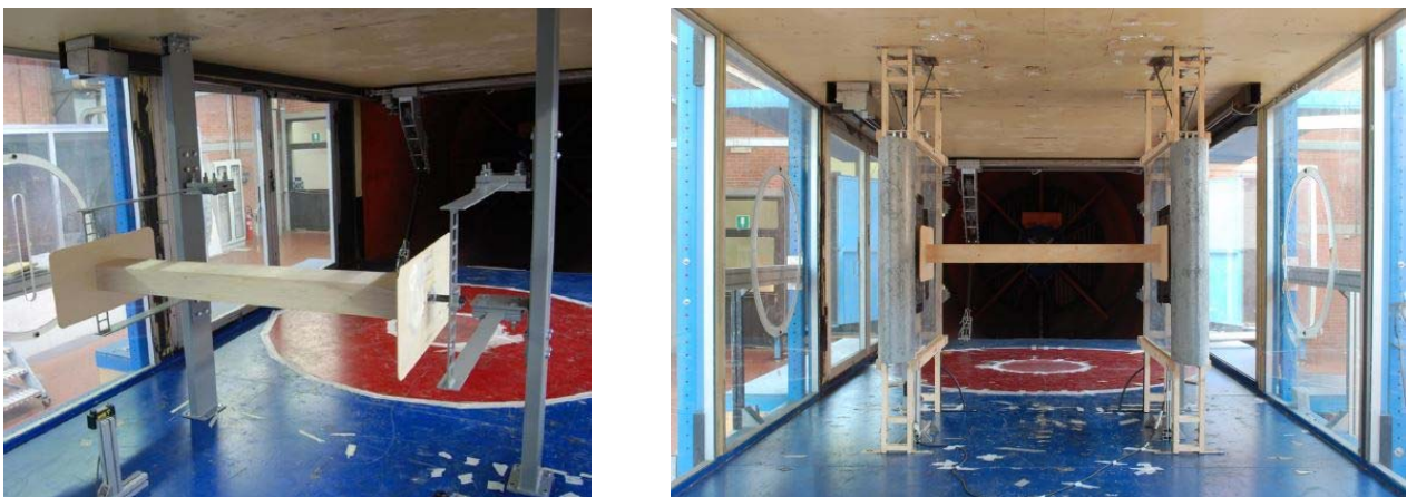
Figure 1: View of the dynamic setup without (left) and with (right) the sheltering system.
