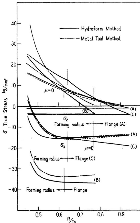
FIGURE 3. Stress distribution in specimen A, B, C for  $t_0 = 1.0$  mm according to hydroform and metal tool methods.
