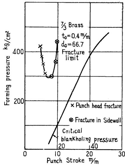
FIGURE 14. Punch stroke vs. forming pressure.
