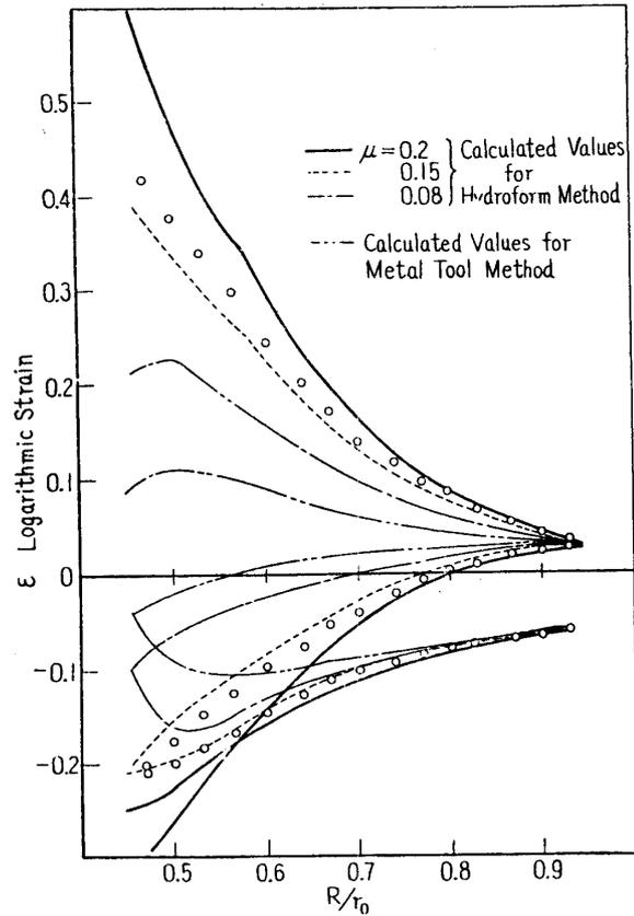
FIGURE 6. Strain distribution in specimen D ( $t_0=0.4$  mm) for various values of friction coefficient.
