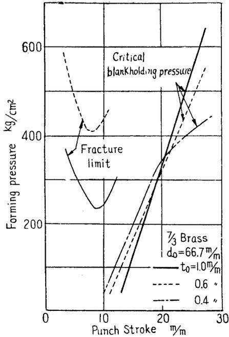
FIGURE 10. Variation of forming pressure according to plate thickness.
