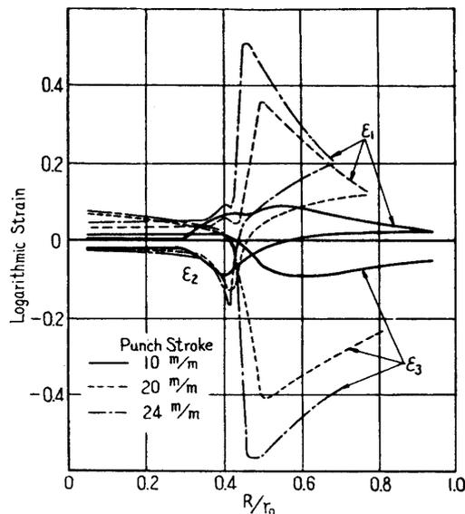
FIGURE 16. Strain distribution in cup according to hydroform method.
