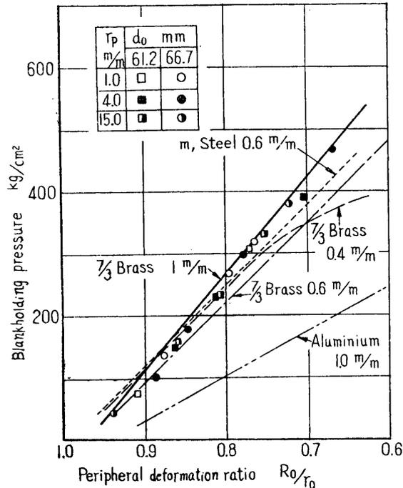
FIGURE 12. Relation of critical blank holding pressure to peripheral deformation ratio.
