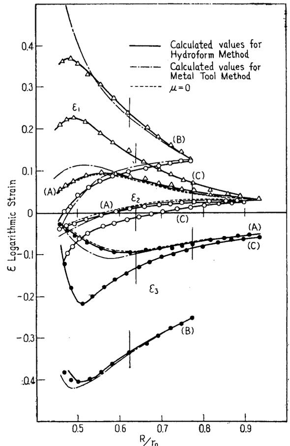
FIGURE 4. Strain distribution for specimen A, B, C for  $t_0 = 1.0$  mm according to hydroform and metal tool methods.
