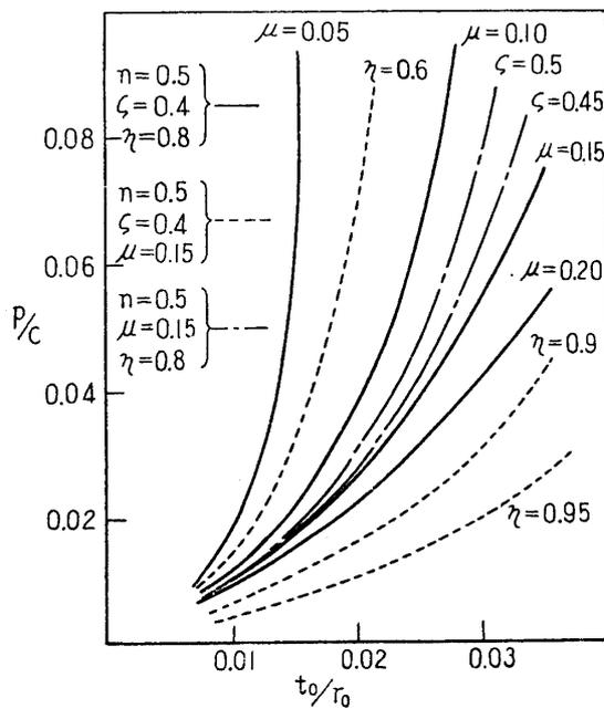
FIGURE 7. Influence of friction coefficient  $\mu$ , peripheral deformation ratio  $\eta$ , and drawing coefficient  $\zeta$ , to  $t_0/r_0$  vs.  $p/c$ .
