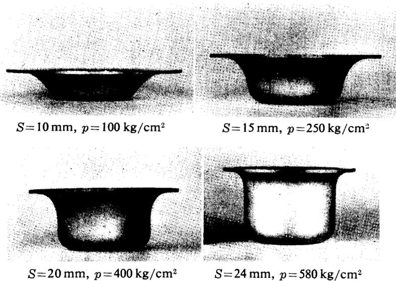
FIGURE 15. Process of blank deformation found in hydroform method. (Material 7/3 brass, 1.0 mm thick., 66.7 mm in diameter)
