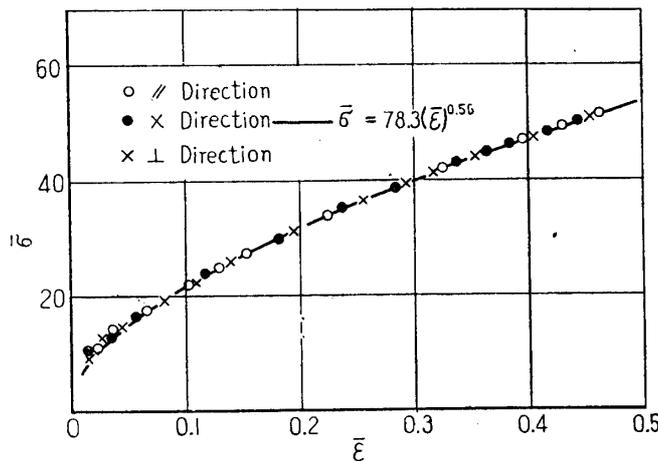
FIGURE 2. Stress-strain curve for 7/3 brass used for calculation.
