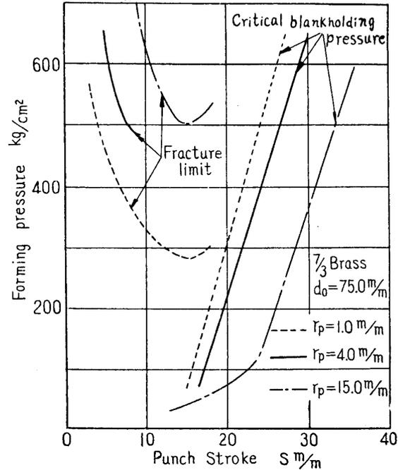
FIGURE 11. Variation of forming pressure according to punch shape.
