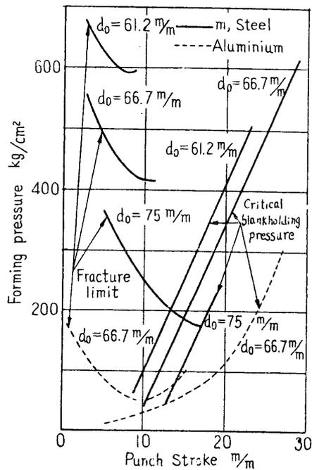
FIGURE 9. Variation of forming pressure according to material and blank diameter.
