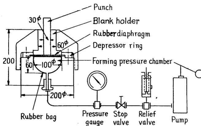
FIGURE 8. Experiment apparatus for hydroform method.
