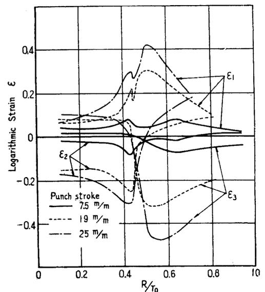
FIGURE 17. Strain distribution in cup according to metal tool method.
