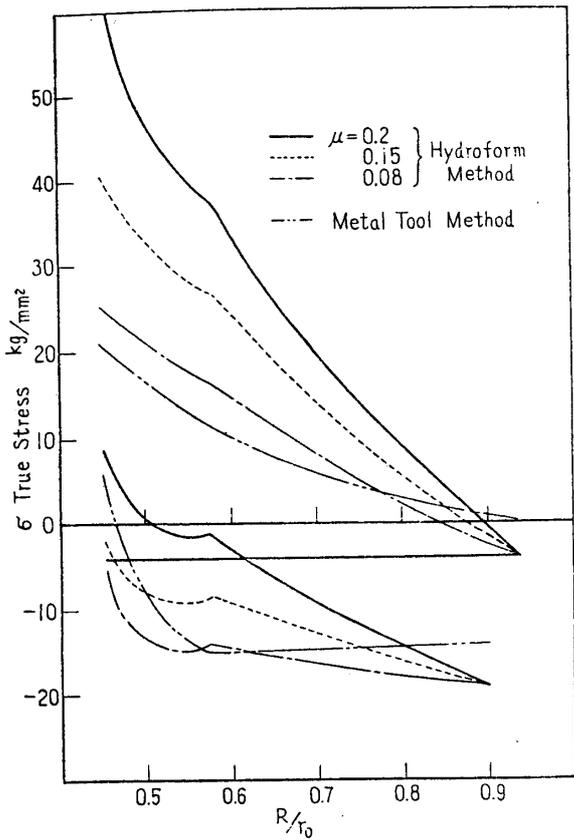
FIGURE 5. Variation of stress distribution for specimen D ( $t_0=0.4$  mm) for various values of friction coefficient.
