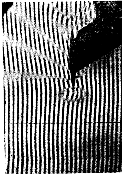
FIGURE 9. Superposed finite fringe interferogram; M_\infty=1.085, \tau=0.1060, \alpha=0^\circ .
