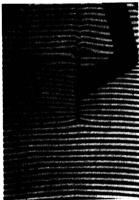
FIGURE 6. Finite fringe interferogram; M_\infty=0.911, \tau=0.0808, \alpha=0^\circ .
