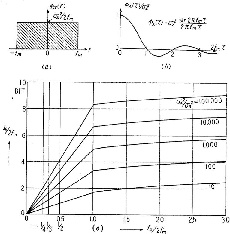
FIGURE 8. The power spectrum of a pure random signal (a), the auto-correlation function (b), and the average information amount obtained through the sampling measurement of this signal (c).
