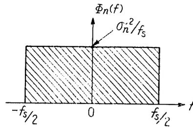
FIGURE 3. The power spectrum of the fictitious noise  $n(t)$ . The noise should be a pure random noise having a flat power spectrum. ( $f_s$ : repetition frequency of the sampling measurement,  $\sigma_n$ : the root mean square value of measurement errors)
