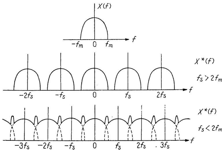
FIGURE 4. The Fourier transform of a impulse modulated signal is a periodic function having a period  $f_s$ .
