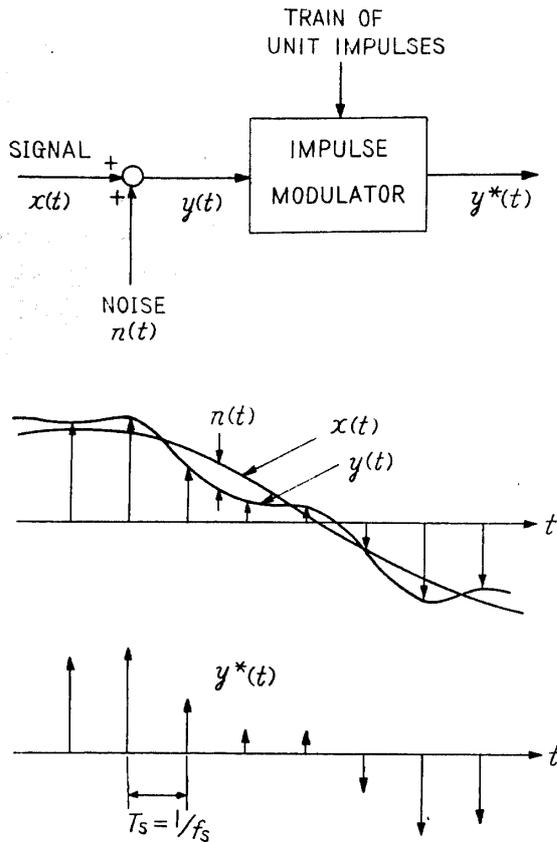
FIGURE 2. The operation of sampling measurement is considered as the impulse modulation of the signal  $y(t)$  which is the superposition of the measured signal  $x(t)$  and a fictitious noise  $n(t)$ .
