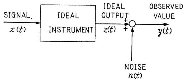
FIGURE 6. Observed value of continuous measurement can be considered as the superposition of ideal error-free output and a fictitious noise representing the errors.
