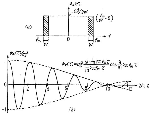
FIGURE 9. The power spectrum (a), and the auto-correlation function (b) of a Gaussena random signal, the frequency band of which does not start at zero.
