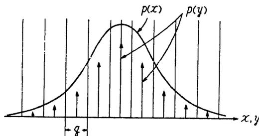
FIGURE 13. Quantization of a time varying random signal. The probability distribution of the magnitude of the quantized signal  $p(y)$  is a discrete one.
