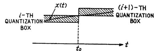
FIGURE 14. The time  $t_0$ , the instant of transition of a time varying random signal from a quantization box to the next, can be measured precisely when the sampling frequency of the A-D converter is increased.
