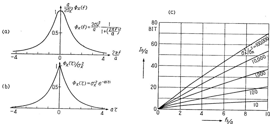
FIGURE 12. A signal power spectrum of bell-jar type (a), and its auto-correlation function (b). The relation of the information amount obtained through the sampling measurement of this signal vs. the sampling frequency is shown in (c).
