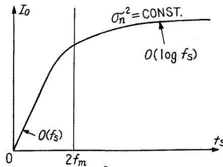
FIGURE 5. The order of increase of information amount obtained per unit time ( $I_0$ ) vs. the repetition frequency of the sampling measurement ( $f_s$ ) when the range of power spectrum of the signal to be measured is limited within  $-f_m \sim f_m$  as shown in Fig. 1.
