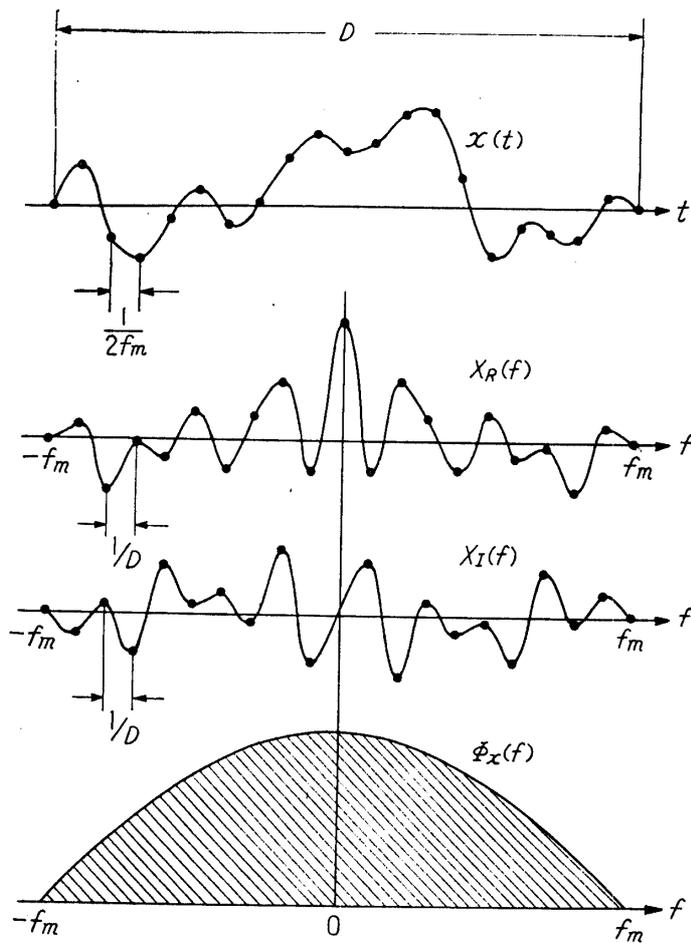
FIGURE 1. A Gaussian random signal which has time duration  $D$  and a maximum frequency  $f_m$ . The free points in the frequency domain are statistically independent of each other.
