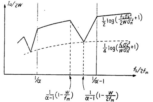
FIGURE 10. The information amount obtained through the sampling measurement of the signal of Fig. 9. The curves exhibit several minimum points.
