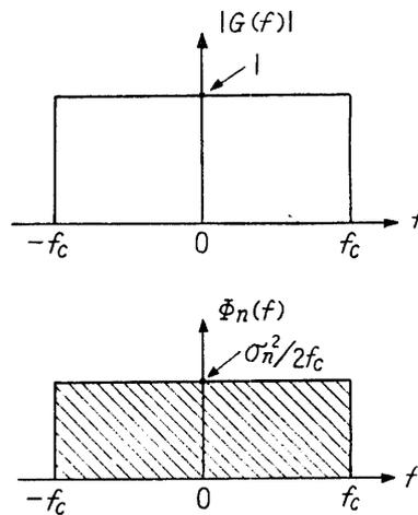
FIGURE 7. Assumed characteristics of the measuring instrument and the power spectrum of the fictitious noise.
