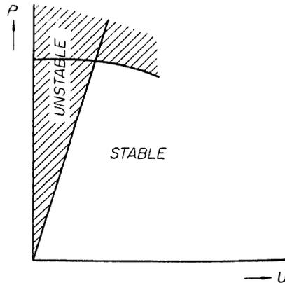
FIGURE 5. Stability Boundary of Elastic Rocket at Low Speed.
