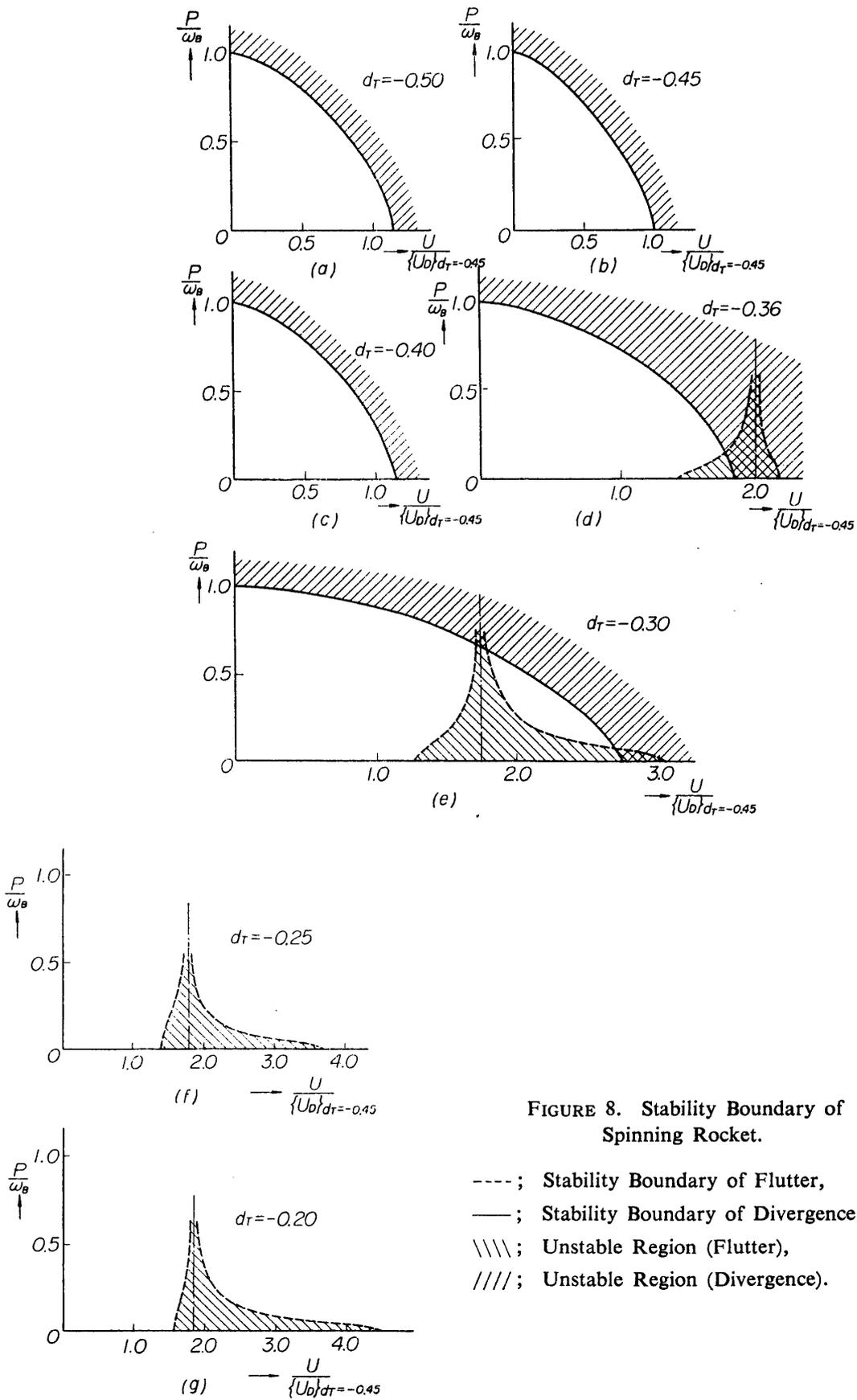
FIGURE 8. Stability Boundary of Spinning Rocket.
