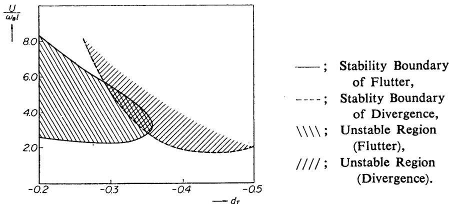
FIGURE 7. Stability Boundary of Nonspinning Elastic Rocket.
