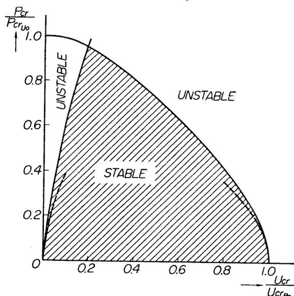
FIGURE 9. Stability Boundary of Spinning Elastic Rocket.
