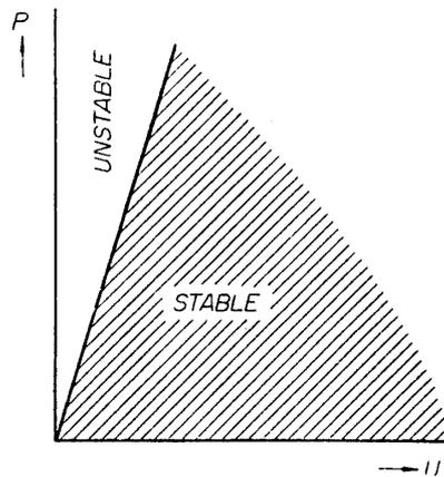
FIGURE 4. Stability Boundary of Rigid Body.
