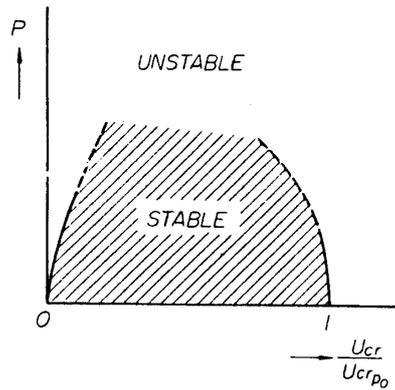
FIGURE 6. Stability Boundary of Elastic Rocket at Low Spinning Rate.
