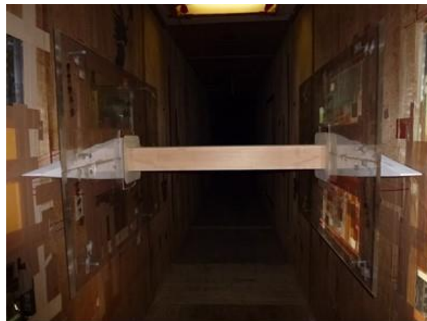
Figure 1: Section model for spring-supported tests mounted in Kyushu Institute Technology wind tunnel
