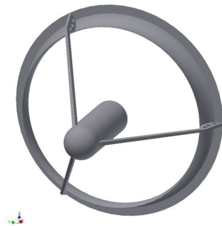
Figure 3: A brimmed diffuser shroud fixed by 3 supports
