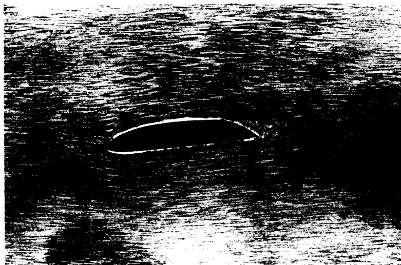
Fig. 98. The "3b" wing. \alpha = -6^\circ .
