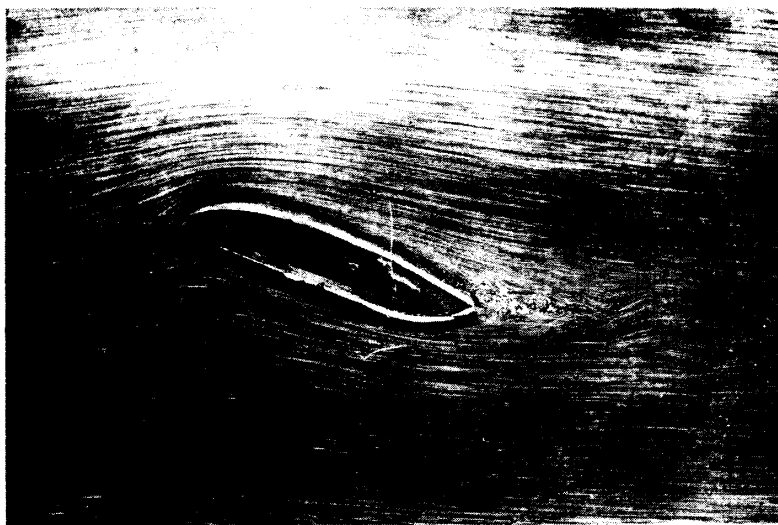
Fig. 111. The "3c" wing. \alpha = +20^\circ . In this case the wake of the wing is considerably small.
