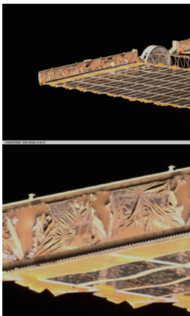
ISS photovoltaic array blanket box cover after one year 1)
