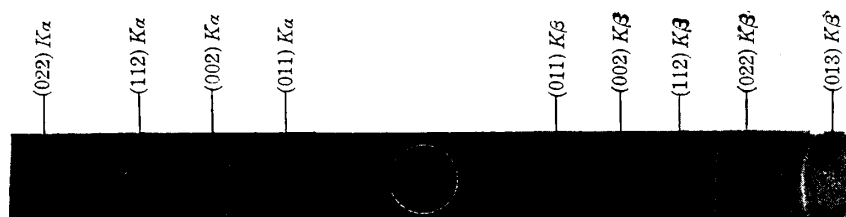
Fig. 7a Fe 70 NiAl 30 powder annealed (Debye-Scherrer camera)
