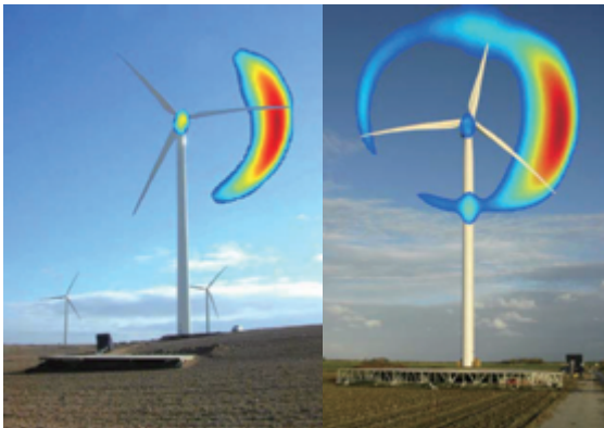
Fig.5 Visualised Noise source of wind turbines. 3)
