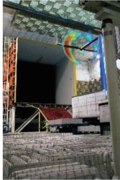
Fig.17 Wind tunnel test model of 3D rotating rotor. 17)
