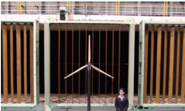
Fig.15 Set-up of wind tunnel test in turbulent wind model.
