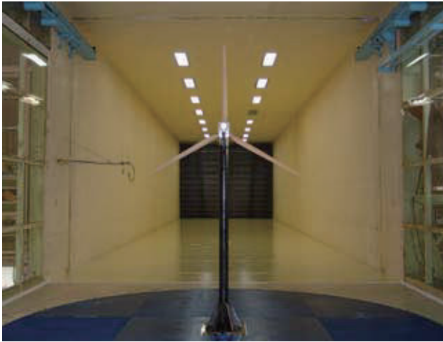
Fig.10 Wind tunnel test model of 3D rotor. 12)
