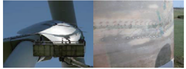
Fig.6 Rotor blade pressure measurement. 4)
