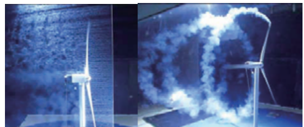
Fig.18 Flow visualisation around the rotating rotor.
