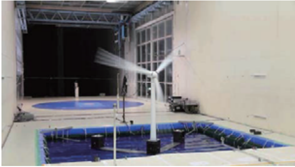
Fig.14 Wind tunnel test of floating wind turbine. 15)
