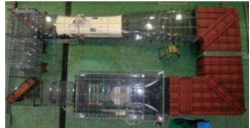
Fig.12 Top view of the model wind tunnel.
