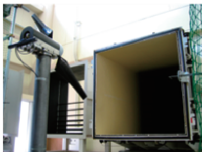
Fig.14 Small wind turbine in wind tunnel
