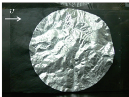
(c) Terrain model by NC machining
