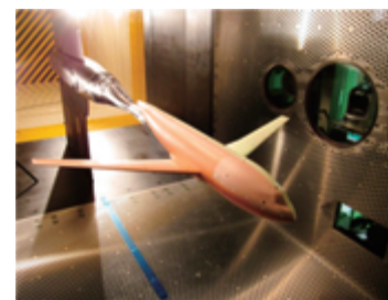
Fig.2 PSP measurement in 6.5m x 5.5m low-speed wind tunnel ( U_{\infty}=60\text{m/s} , \text{AoA}=15\text{deg} ).
