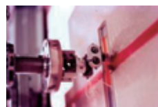
(b) Shackle part attached at left hand of the shaft of active model
