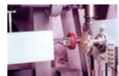
(c) Gimbal part attached at right hand of the shaft of dummy model
