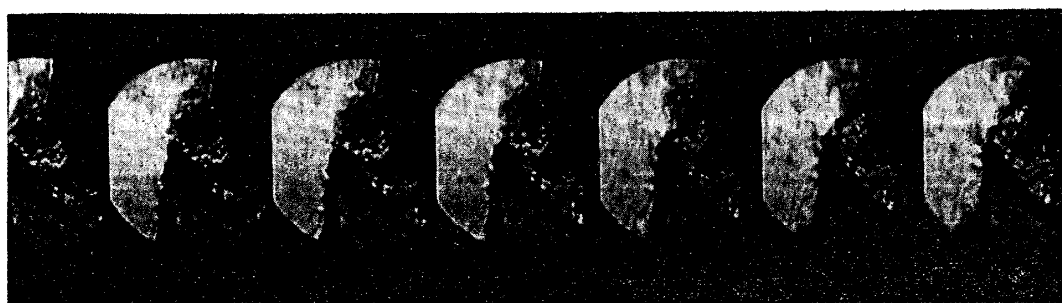
Fig. 12. Aluminium Alloy, the Built-up Edge formed, Slow Cutting Speed.
