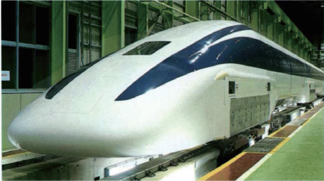
Superconductive Magnetically Levitated train System
