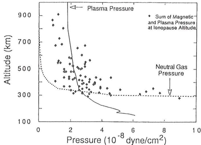
Fig.16: A plot of ionopause altitude versus  $P_{sw}$ . Also plotted are model values of plasma and neutral pressure. At low  $P_{sw}$ , ionopause tracks the plasma pressure but at higher values it tracks the neutral pressure (from Mahajan et al., 1989).
