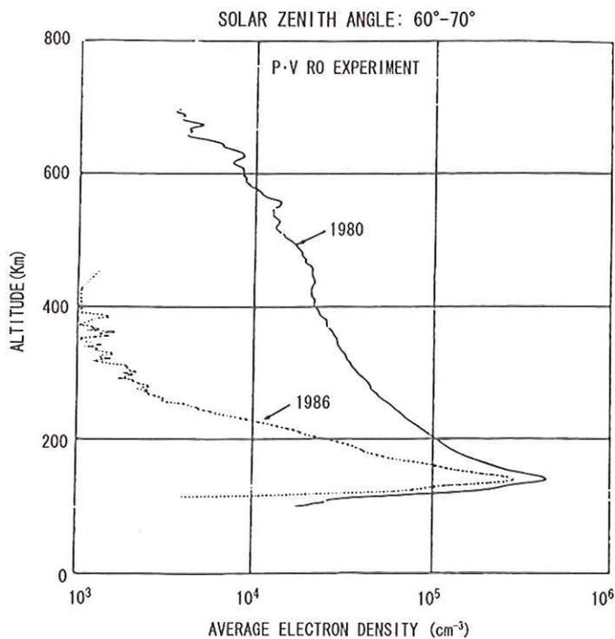
Fig.11: Electron density profiles obtained by PVO radio occultation at solar maximum (1980) and solar minimum (1986). A large depletion in the dayside upper ionosphere at solar minimum can be noted (from Knudsen et al., 1987).
