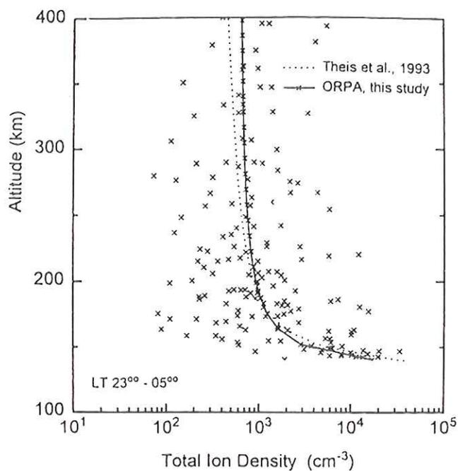
Fig.18: Nightside electron density values measured during the entry period by ORPA. Large variability in the density can be noted (from Spenner et al., 1995).
