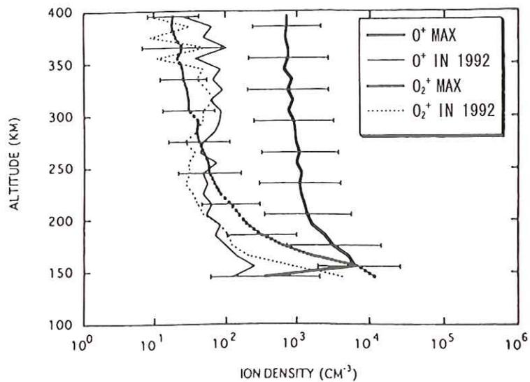
Fig.9: Average altitude profiles of  $O^+$  and  $O_2^+$  during the primary mission of PVO (solar max.) and in 1992 during PVO entry with data from midnight to 04:30 (from Kar et al., 1994).
