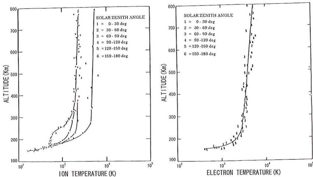
Fig.12: Plasma temperatures as measured by ORPA (a) electron temperatures (b) ion temperatures. There is little diurnal change in the temperatures. Ion temperature is about one half of the electron temperature, except in the antisolar region, where the two are equal (from Miller et al., 1980).
