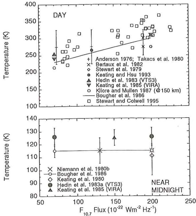
Fig.5: Dayside and near midnight exospheric temperature measured over a solar cycle. The temperature changed by 60 K for the day and less than 15 K for the night from solar maximum to solar medium (from Kasprzak et al., 1997).
