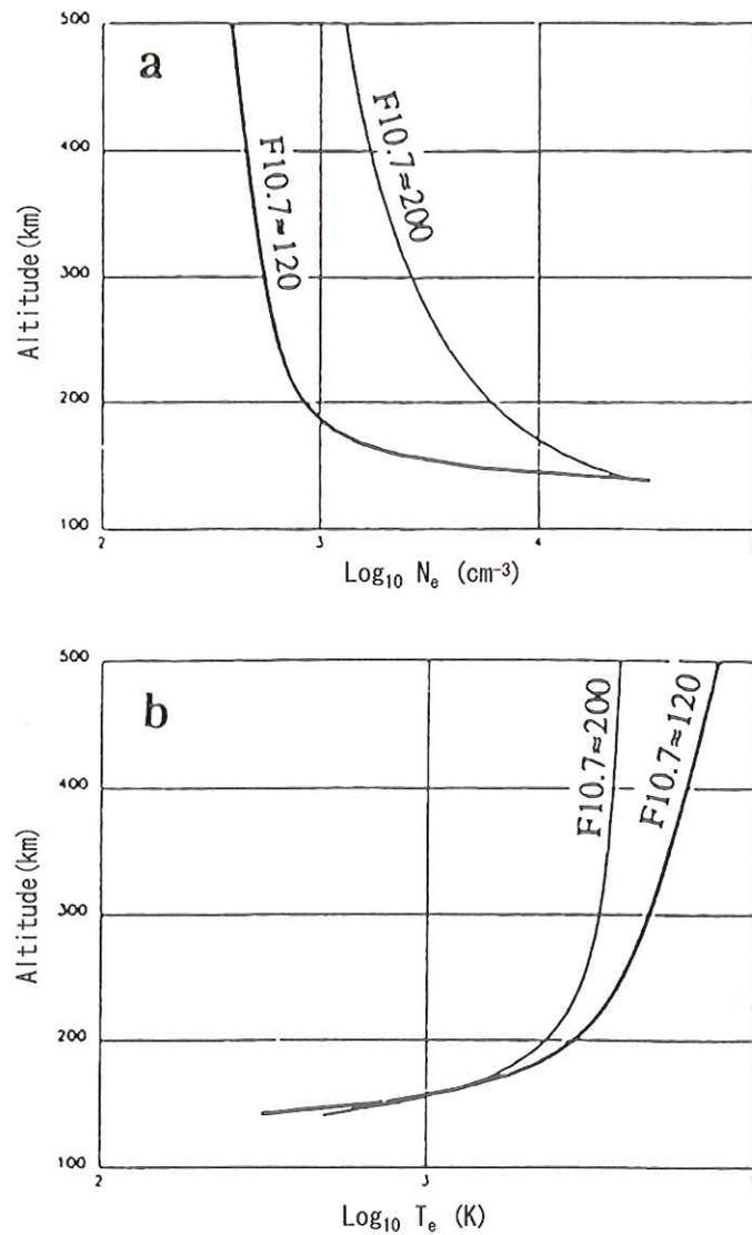
Fig.17: Comparison of electron densities and temperatures measured by the OETP instrument during the pre-entry period ( $F_{10.7} \approx 120$ ) and solar maximum ( $F_{10.7} \approx 200$ ). While the densities decreased, the temperatures increased during the pre-entry period (from Theis and Brace, 1993).
