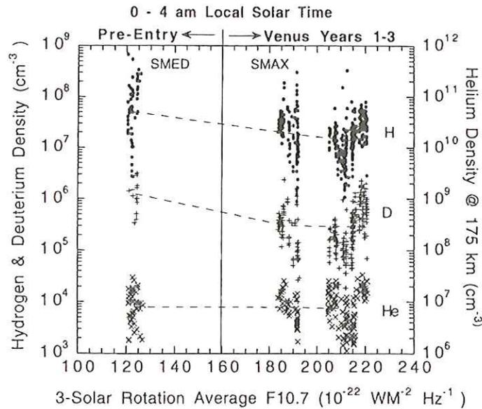
Fig.6: Variation of H, D and He densities with solar activity for local solar time 0 to 4 hr. Densities decrease with increase in solar activity (from Kasprzak et al., 1997).
