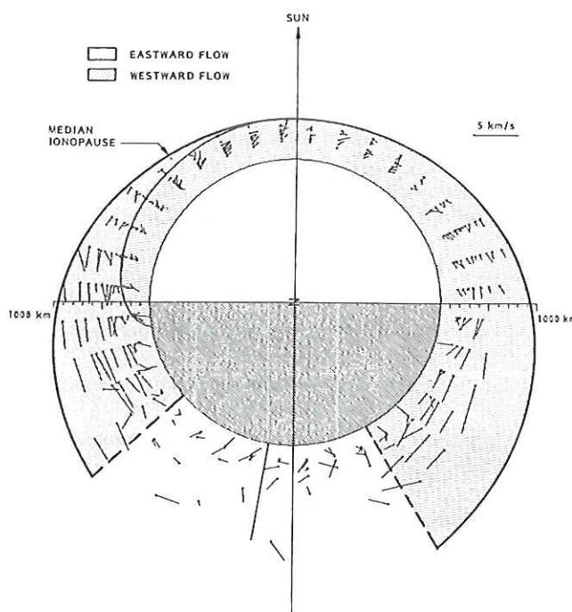
Fig.19: Average O<sup>+</sup> velocity as measured by the ORPA instrument. Large velocities at the terminators are responsible for the maintenance of the nightside ionosphere (from Miller and Whitten, 1991).
