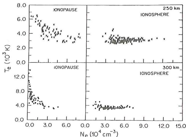
Fig. 13: Inverse correlation between the electron temperature and density in the ionopause region. The temperature in the main ionosphere remains nearly constant, while most of the variability is due to variations in the ionopause region (from Mahajan et al., 1994).
