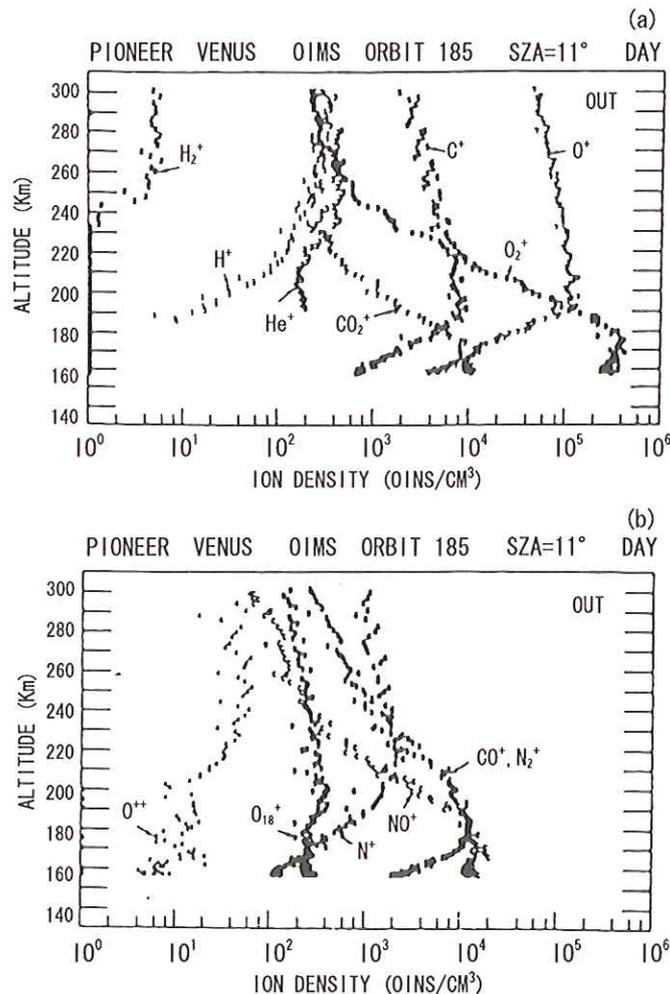
Fig.7: Ion composition measurements from a single PVO passage through the subsolar ionosphere demonstrating that  $\text{O}_2^+$  is the dominant ion below 200 km, while  $\text{O}^+$  dominates above it (from Taylor et al., 1980b).
