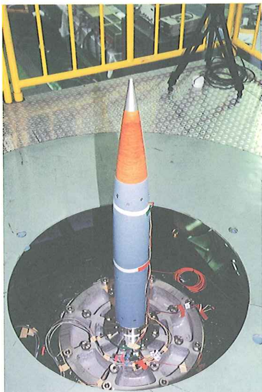
Photograph 4. Payload section of the MT-135 rocket mounted on the V-test stage
