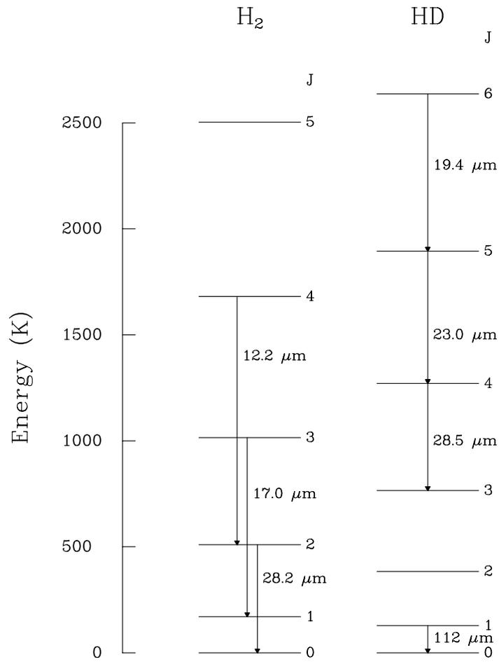
Fig. 3: Energy level diagrams for the H<sub>2</sub> and HD molecules, with the lowest few transitions labeled.
