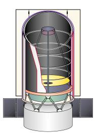
Fig. 1: Conceptual design of the HII/L2 mission with a 3.5 m primary mirror.
