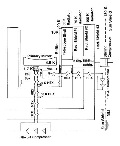
Fig. 2: Schematic drawing of the cryogenic system of the HII/L2 mission. The telescope is enshrouded with multi-layered radiators. One set of a JT cooler (with <sup>4</sup>He) and a two-stage Stirling cycle is used to cool the telescope and some of focal plane instruments to 4.5 K. Another set of a JT cooler (with <sup>3</sup>He) and a two-stage Stirling cycle is used to cool the far-infrared detectors to 1.7 K.
