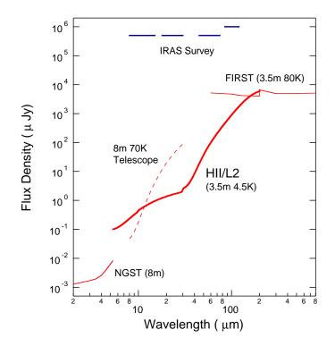
Fig. 4: Comparison of point-source sensitivity (5  $\sigma$  flux density at 3,600 s integration) of various infrared missions. Diffraction-limited observations with  $\lambda/\Delta\lambda = 5$  is assumed for HII/L2.
