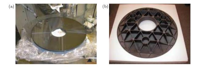
Fig. 7: Flight-model (FM) primary SiC mirror under polishing: (a) front surface and (b) rear surface.
