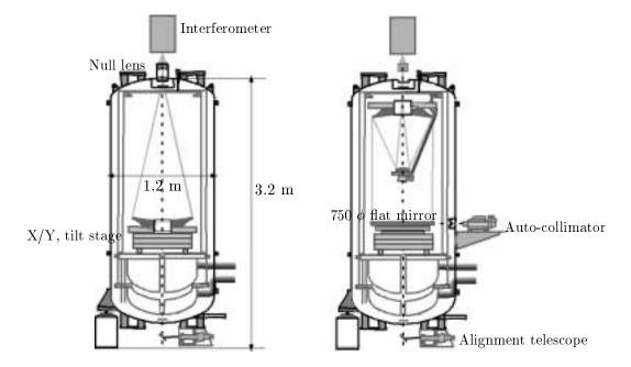
Fig. 5: Schematic view of measurements of mirror figures: primary mirror (left) and telescope assembly (right).
