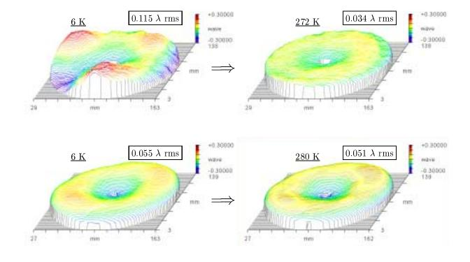
Fig. 3: The change of the surface figure for the second SiC test mirror (upper) and the fourth SiC test mirror (lower) with temperature. All figures are shown in the same scale.
