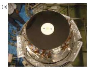
Fig. 6: (a) Cryogenic test chamber for 710-mm diameter mirrors. (b) Graphite-core-CVD-SiC-coat mirror placed at the cold stage inside the cryostat.
