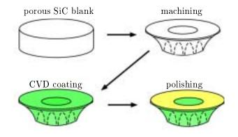
Fig. 2: Fabrication of sandwich-type SiC mirror
