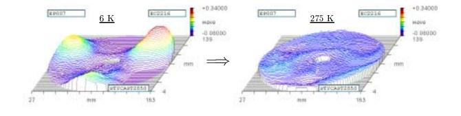
Fig. 4: The change of the surface with temperature: the fourth mirror + glue + super-invar (support structure)
