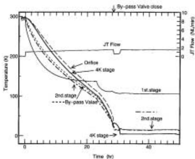
Fig. 5: Cool-down Operation (Orifice size  $20 \mu\text{m}$ )
