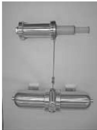
Fig. 3: Photograph of two-stage Stirling cycle cooler
