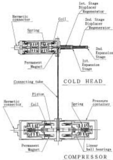
Fig. 2: Schematic Drawing of two-stage Stirling cycle cooler
