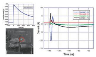
Figure 7. Discharge current waveforms and voltage waveform due to discharge on the thermal exposed sample. Corresponding ESD image captured by camera, inside red circle, is also shown.
