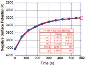
Figure 8. Charging profile coverglass while - 4kV biased sample was exposed to electron beam. Blue circles are the surface potential measured by TREK before the discharge occurred. Red line is the exponential fitted curve. Fitting parameters are shown on the table.
