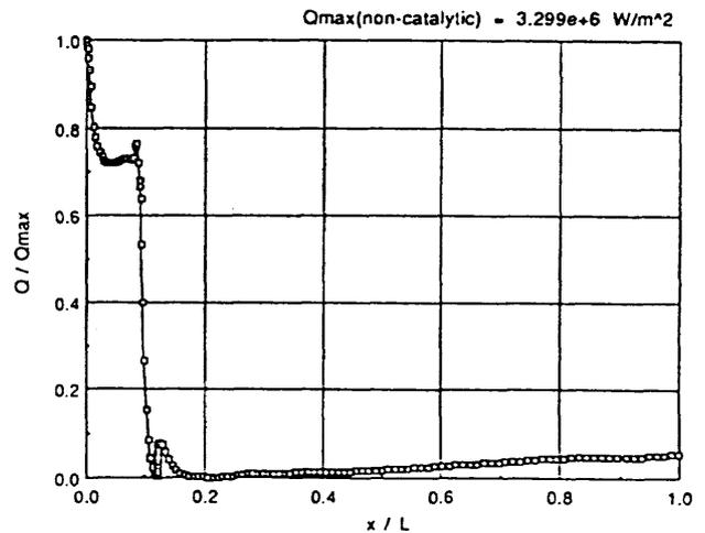
Fig 15 Heat flux distribution for Problem IV.1 (Non-catalytic wall case)
