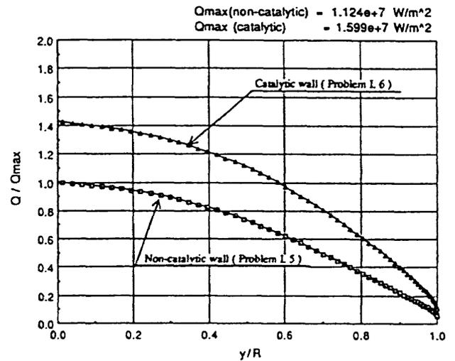
Fig. 8 Heat flux distribution for Problem I.5 and 6
