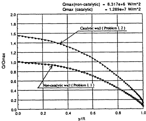
Fig. 6 Heat flux distribution for Problem I.1 and 2
