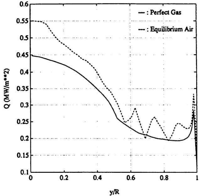
Fig. 3 Heat Flux Distribution on OREX
