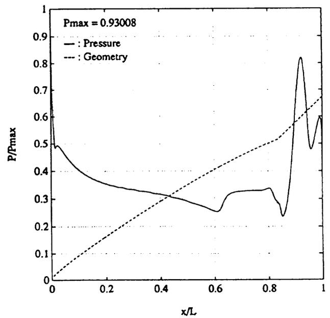
Fig.8 Pressure Distribution on Hyperboloid Flare
