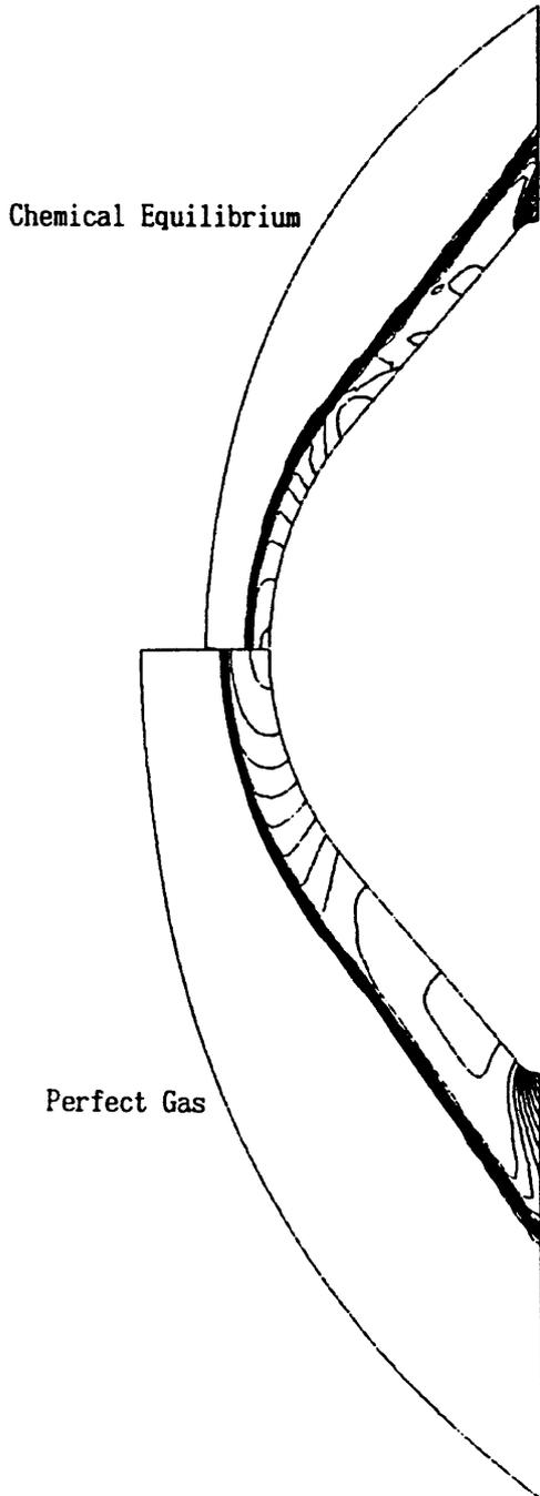
Fig. 2 Pressure Contours around OREX
