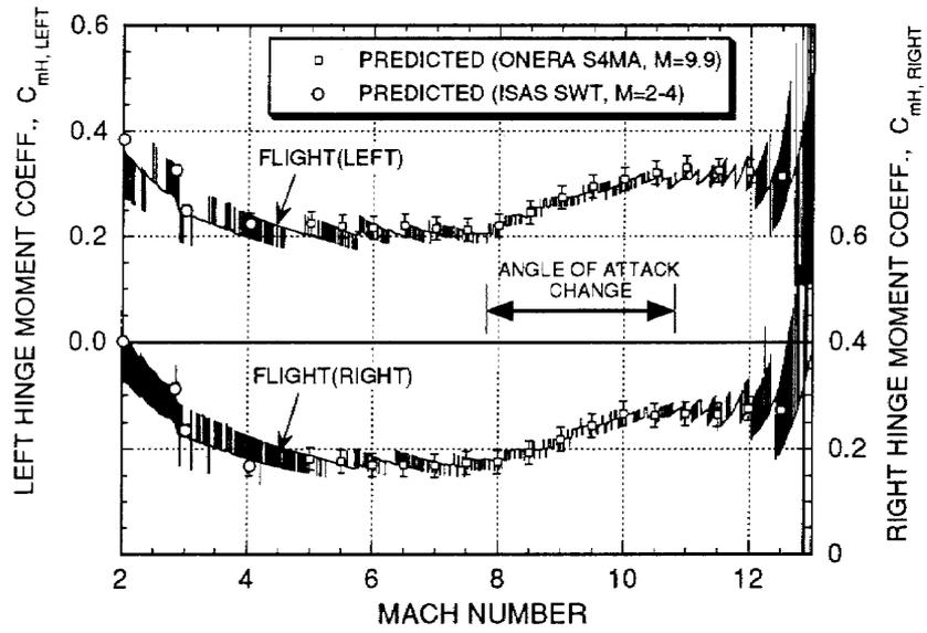
Fig. 9 Elevation hinge moment comparison.
