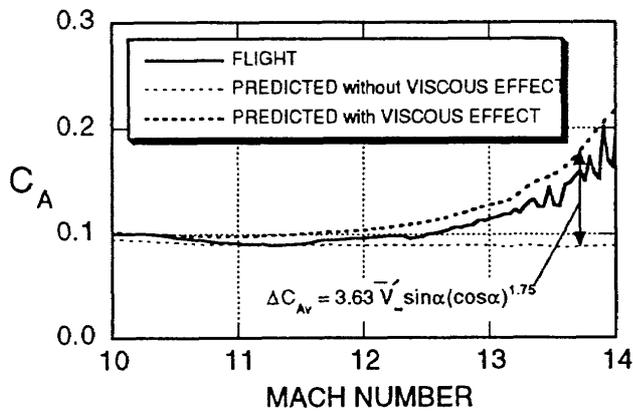
Fig. 5 Viscous interaction effects on axial force coefficients.
