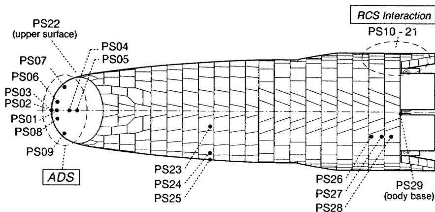
Fig. 3 Location of surface pressure measurement ports.
