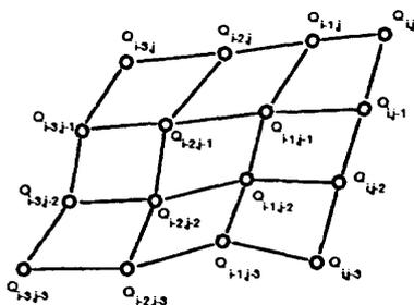
Fig. 6 Control points  $Q_{i,j}$  for B-spline surface.
