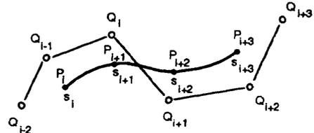
Fig. 3 A B-spline curve and control points.
