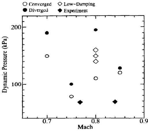
Fig 7. Flutter Boundary of YXX Wing Model ( $\alpha=0.0^\circ$ )
