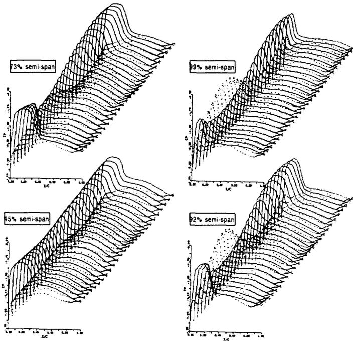
Fig. 6. Pressure Distributions of Upper and Lower Surfaces for One Cycle  $\alpha=0.0$ ,  $M=.7$ ,  $R_e=10^6$ ,  $K=.381$
