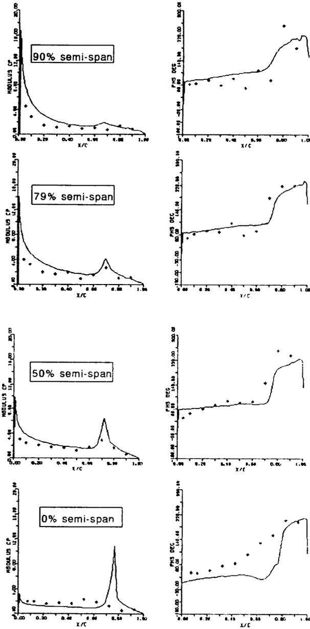
Fig. 1. Comparison of Magnitudes and Phase Angles Between Present Results and Experimental Ones (lines are present results)
