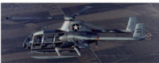
Fig. 2-4. The McDonnell Aircraft Corp., Helicopter Division's XV-1 Convertiplane. At maximum speed, the rotor operated at an advance ratio just below 1.
