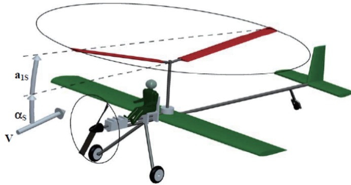
Fig. 2-10. The simple elements of autogyros and compound helicopters. Tail rotor not shown for clarity. Rendition provided by Gerardo Nunez from author's sketch.
