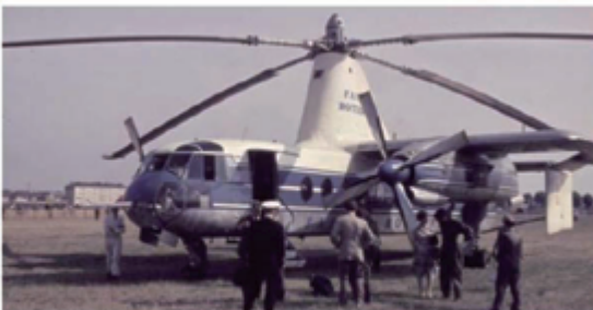
Fig. 2-5. The Fairey Rotodyne was successfully developed, but British Government and civil funding eroded in the late 1950s. This was the largest compound helicopter ever flown. Its maximum advance ratio was below 1.
