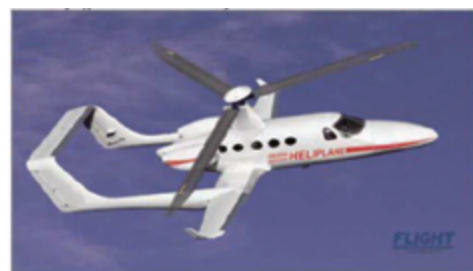
Fig. 2-9. The DARPA funded Groen Brothers Heliplane is expected to reach 400 mph with the rotor operating at an advance ratio near 2.
