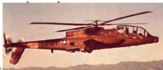
Fig. 2-7. The AH-56's rotor reached an advance ratio slightly over 0.52 at a flight speed of 204 knots.
