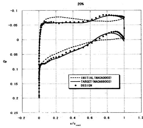
Figure 5. Comparison of surface pressure distributions ( $y/l=20\%$ )
