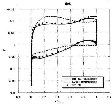
Figure 6. Comparison of surface pressure distributions ( $y/l=50\%$ )
