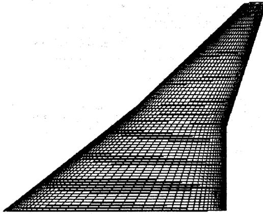
Figure 4. The wing geometry of initial wing
