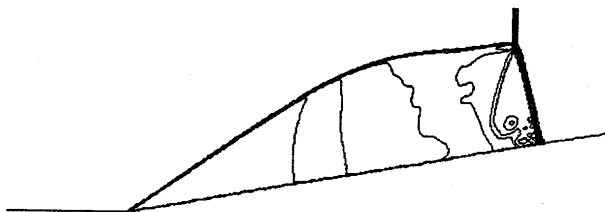
図 7: Computational result(instantaneous density contours), M_s=15 (Chemically frozen flow)
