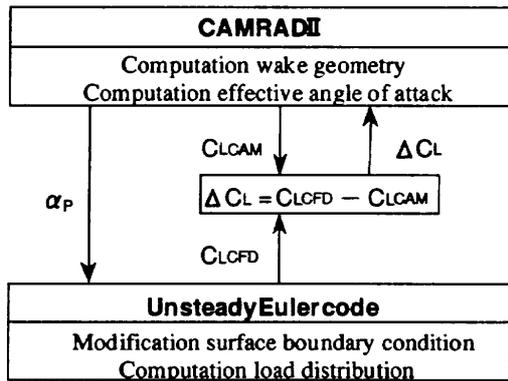
$\alpha P$  : partial angle of attack excluding effect of wake vorticity in computational domain of CFD
