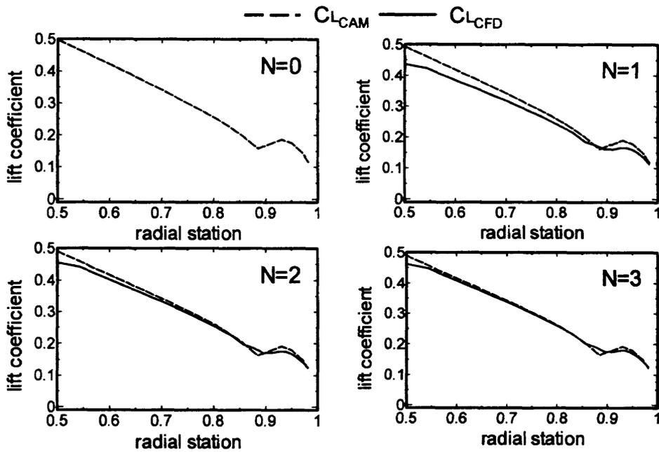
Figure 11 Evolution of lift coefficients ( $M_{tip}=0.663$ ,  $\mu=0.164$ ,  $\alpha_{tip}=2^\circ$ ).
