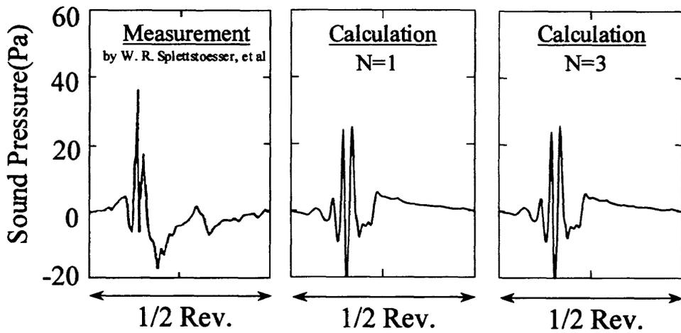
Figure 12 Iteration effect for BVI noise prediction.
