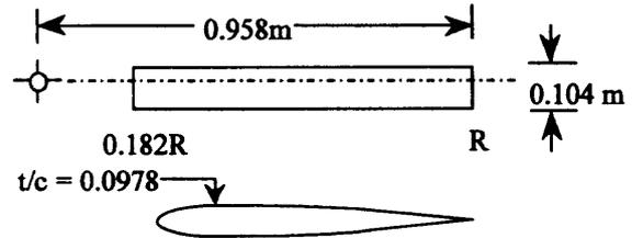
Figure 5 Rotor characteristics
