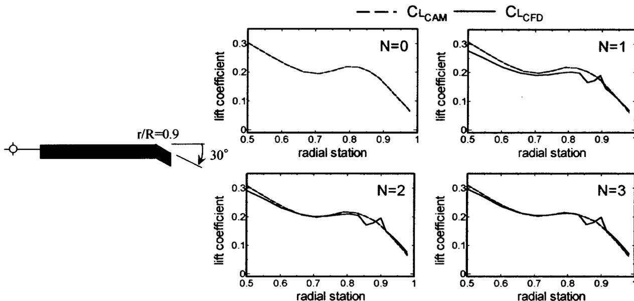
Figure 8 Evolution of lift coefficients ( $M_{tip}=0.663$ ,  $\mu=0.298$ ).
