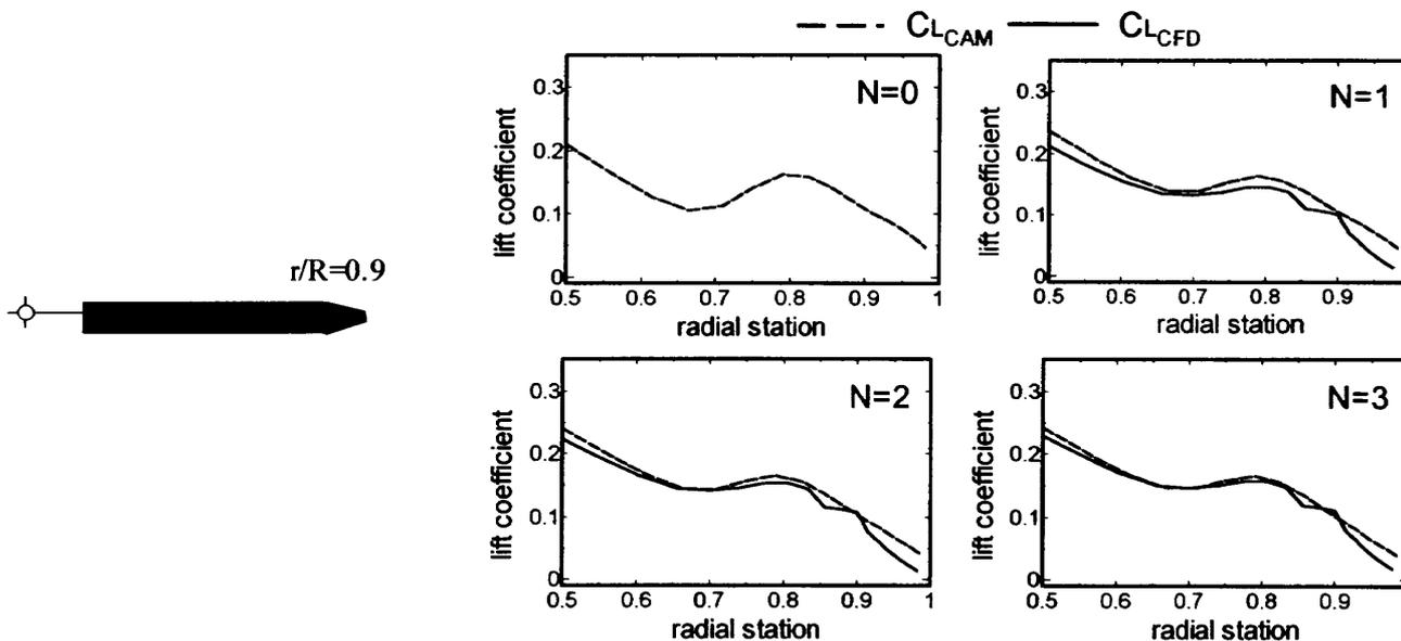
Figure 9 Evolution of lift coefficients ( $M_{tip}=0.663$ ,  $\mu=0.298$ ).
