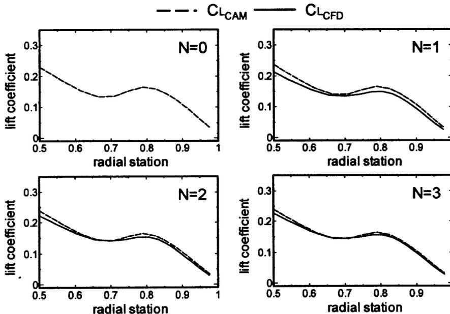
Figure 6 Evolution of lift coefficients ( $M_{tip}=0.663, \mu=0.298$ ).
