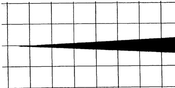
Fig.9 Grid around double wedge with refinement level 4 at  $C/L_{min} = 64$ , where edge point is off the cell center.
